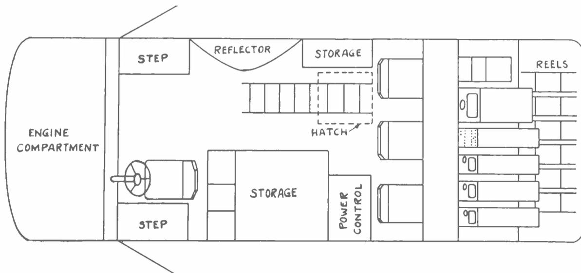
FIG. 13 (left). A novel part of this suggested plan is a provision for using the field equipment for studio pickup—without the necessity of removing it from the truck. The rear of the truck (see diagram at left) is, in effect, a glassed-in control position. When the truck is backed into the garage (see Fig. 14) this control position looks directly into the studios providing an entirely practical (although somewhat restricted) operating arrangement.
