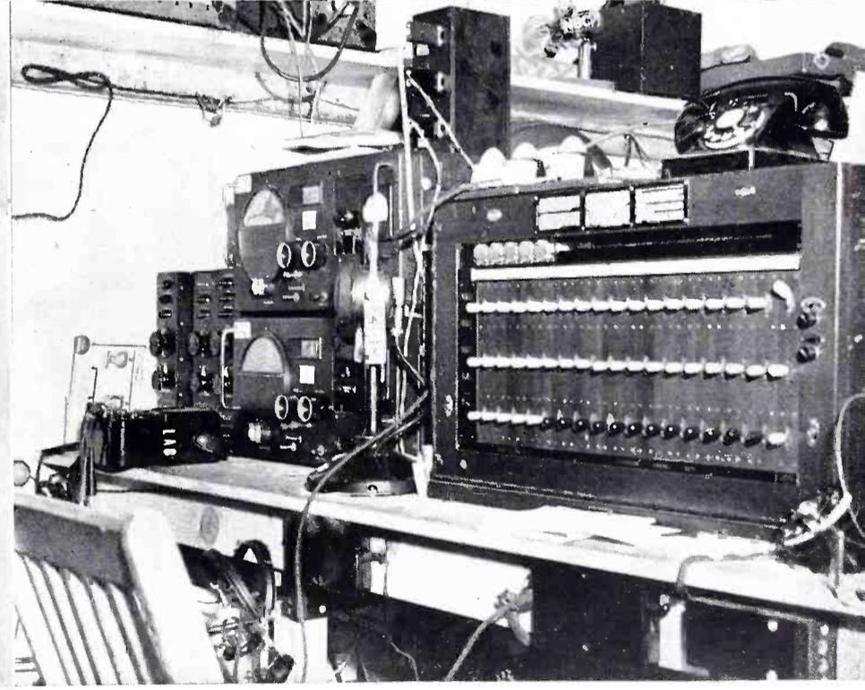
**RECEIVING POSITION** in NBC control room is shown here. Two communication-type receivers were used to pick up 27 mc transmissions from the radio mikes on the Convention Hall floor,
