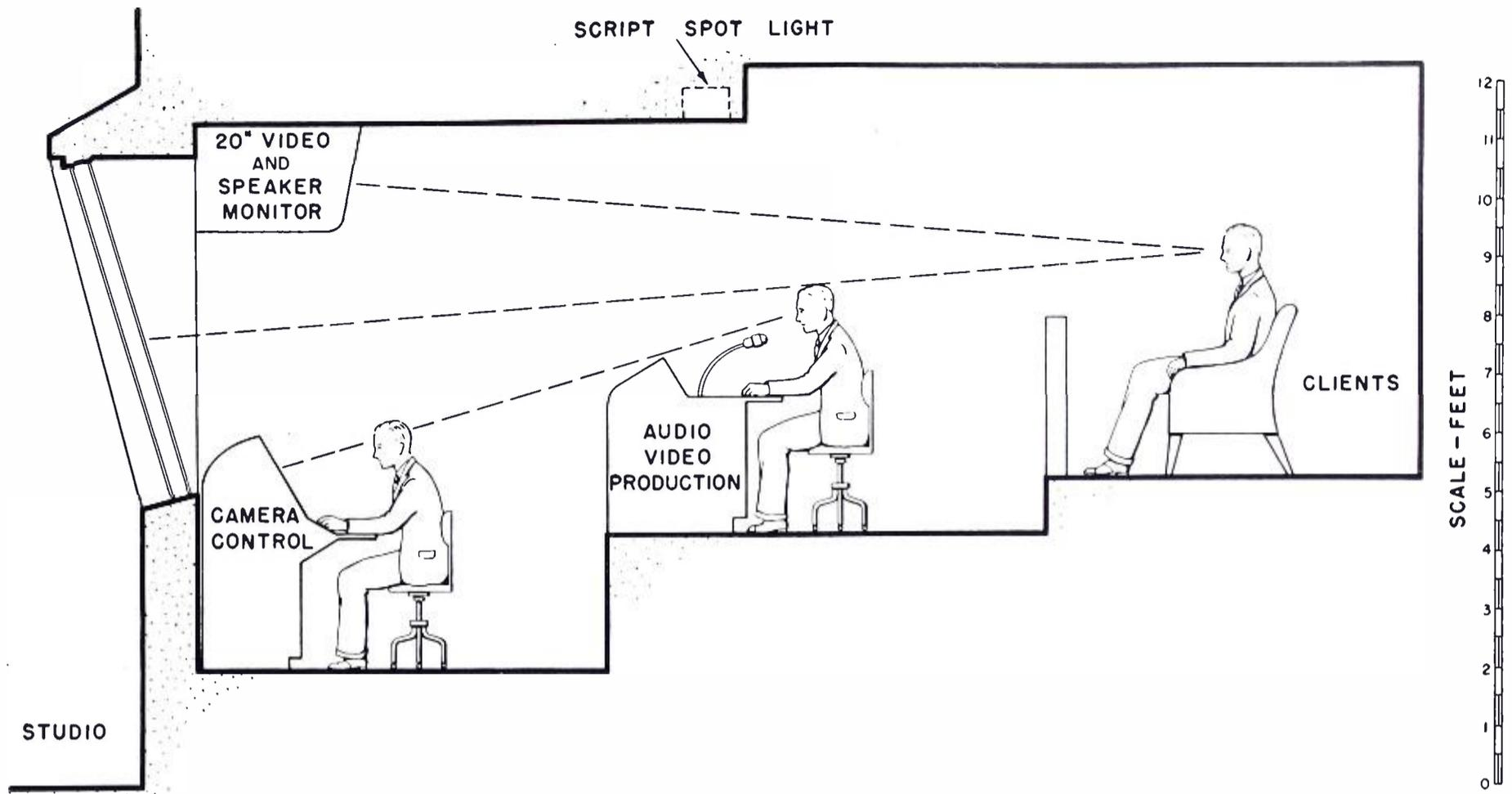
FIG. 7. Cross-section plan of the control rooms associated with Studios A and B. Video operators sit at a level slightly above the studio floor. Production director, switcher, and audio engineer on a second level, and clients at a third level. Broken lines indicate site lines.
