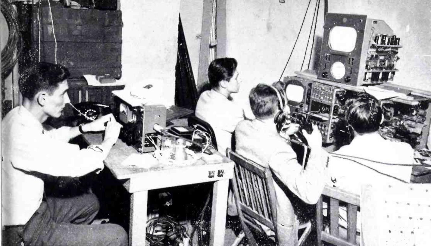
NBC's HOTEL CONTROL ROOM is shown at the left. Video units (at right of picture) include two RCA TK-30A Camera Control Units, with a TS-30A Switcher between, and a TM-5A Master Monitor on top. Audio position, at left, features an OP7.
