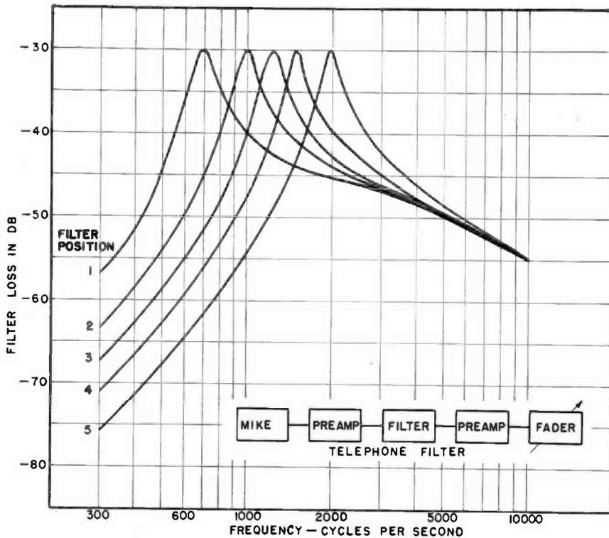
FIG. 6 (above). Typical telephone filter characteristics.
