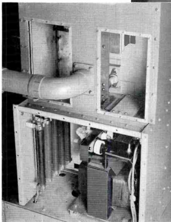
loaded three-quarter wave line, shorted at the input, is used for the filament circuit. This line is formed by the power-frequency filament buses which are folded over and pass down at the back of the plate line.
