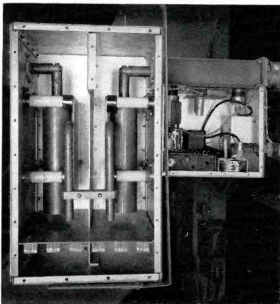
FIG. 14 (below). D. G. Robertson, RCA engineer, illustrates how hinged turret panels of the BTC-1A supervisory console provide complete accessibility. Note that individual meter panel may be tilted back for easy zero adjustments. Transmitter control turret is at left; audio control turret, at right.
