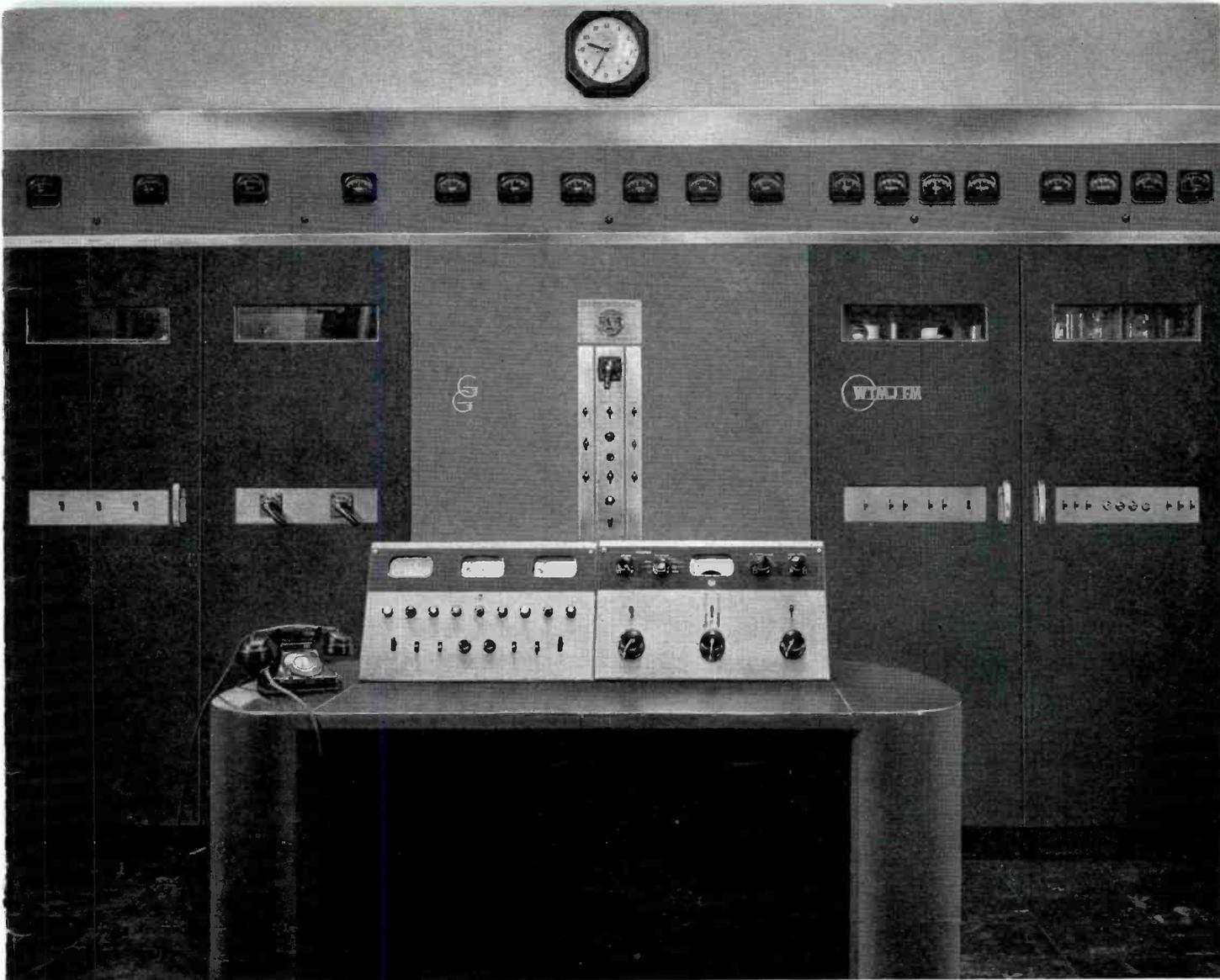
FIG. 2 (above). The final, commercial design 50 kilowatt FM transmitter as installed at WTMJ-FM, Milwaukee. The unified-front panel is finished in a two-tone umber gray to match companion equipment. In foreground is the BTC-1A supervisory console supplied with the transmitter.
