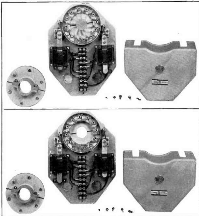
FIG. 3 (above). View of the shorting switch in the "open" position. Mounting flange is shown at left and protective cover at right.
