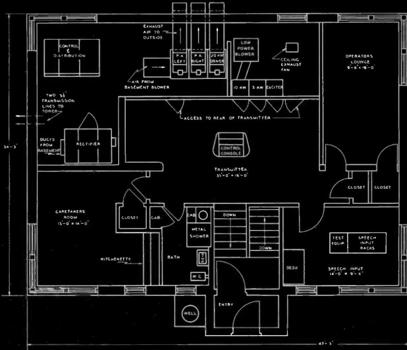
inets, and to the entire transmitter enclosure area. To the rear of the left-hand and center control panels are the three power amplifiers which combine to make up the 50 KW power amplifier.
