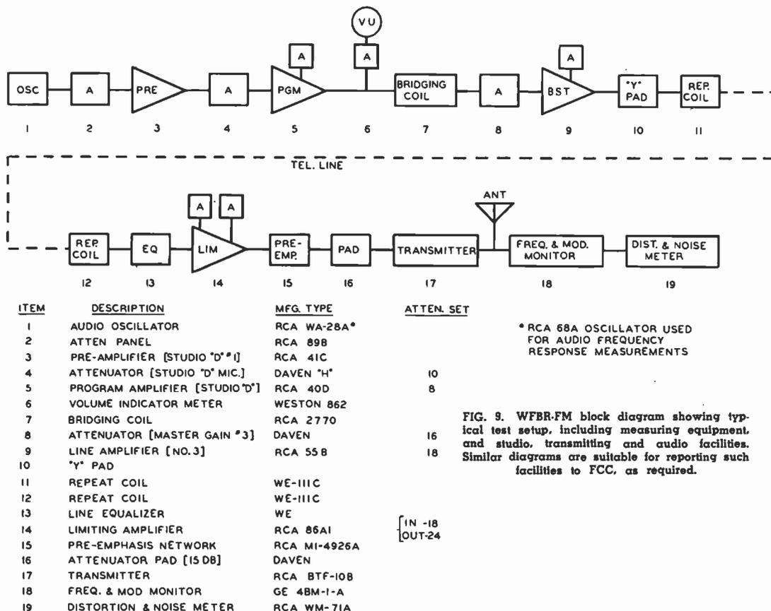
FIG. 9. WFBR-FM block diagram showing typical test setup, including measuring equipment and studio, transmitting and audio facilities. Similar diagrams are suitable for reporting such facilities to FCC, as required.
