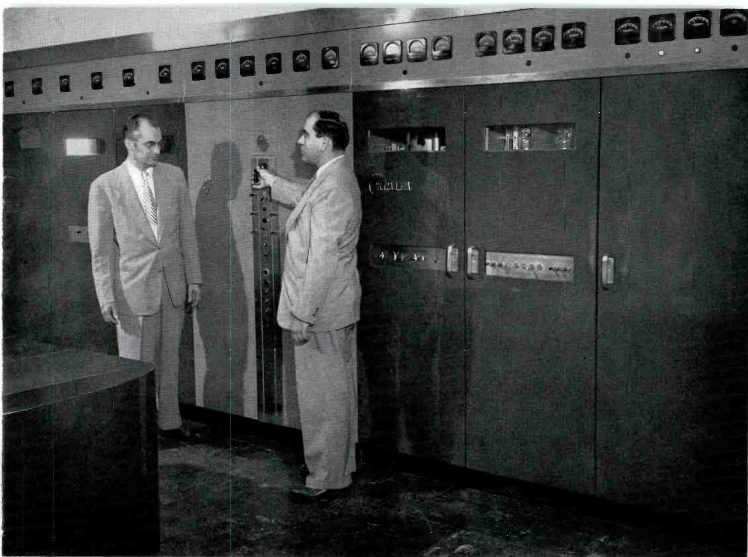
FIG. 2 (above). Phillip B. Laeser, WTMJ chief engineer, observes as W. B. Fletcher, RCA engineer, demonstrates ease of power cut-back to 10 KW from 50 KW operation. All units of the RCA 50 KW FM transmitter are mounted behind a unified front panel providing a neat business-like arrangement with complete accessibility.
