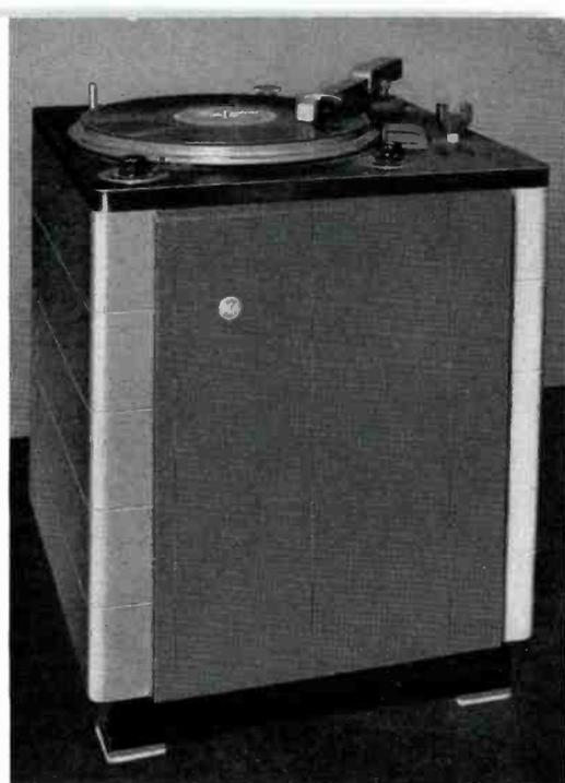
FIG. 1. View of popular RCA type 70-D turntable equipped with three simple sponge rubber shock mounts which effect an improvement of 6 db.
