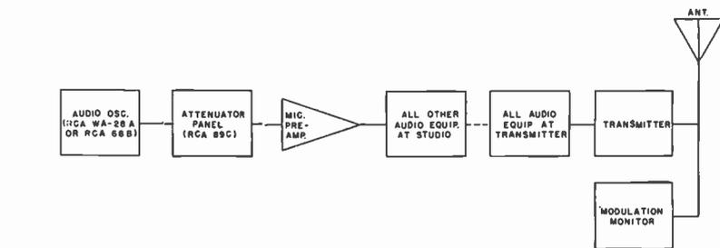
FIG. 2 (above). Block diagram of recommended equipment setup for measuring audio frequency response.
