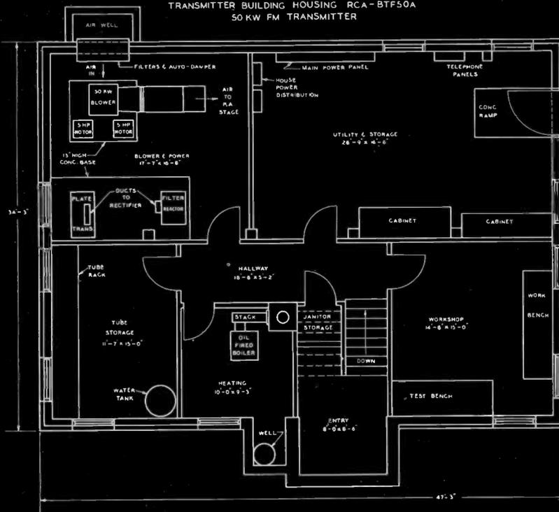
FIG. 4 (at top). First floor plan view of WTMJ-FM transmitter building shows location of 50 KW FM transmitter components. Note that doors provide walk-in access to entire transmitter enclosure.
