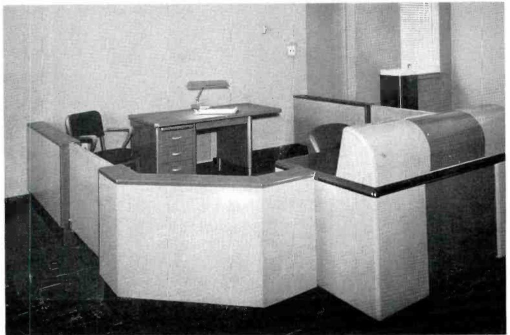
FIG. 3. The operator's console is enclosed on two sides by a low fence giving the enclosure the atmosphere of a private office. A modern desk serves as a convenient place for the operator to fill out the station log.
