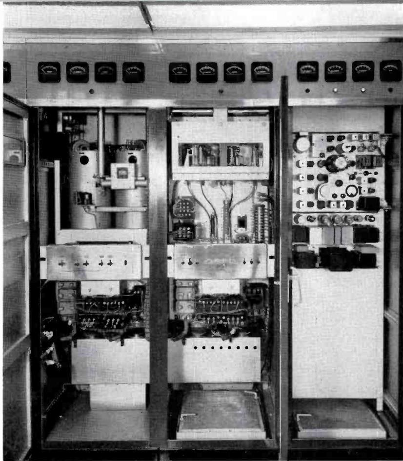
FIG. 6 (above). Closeup view of the "Direct FM" exciter at right, 1 and 3 KW low-power, grounded-grid amplifiers at center and 10 KW grounded-grid amplifier at extreme left.
