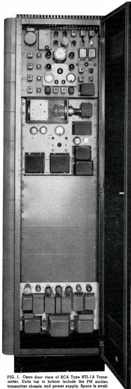
FIG. 1. Open door view of RCA Type BTL-1A Transmitter. Units top to bottom include the FM exciter, transmitter chassis and power supply. Space is available for installation of multiplexing equipment for message service or separate communications link.
