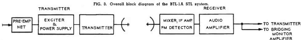
FIG. 3. Overall block diagram of the BTL-1A STL system.
