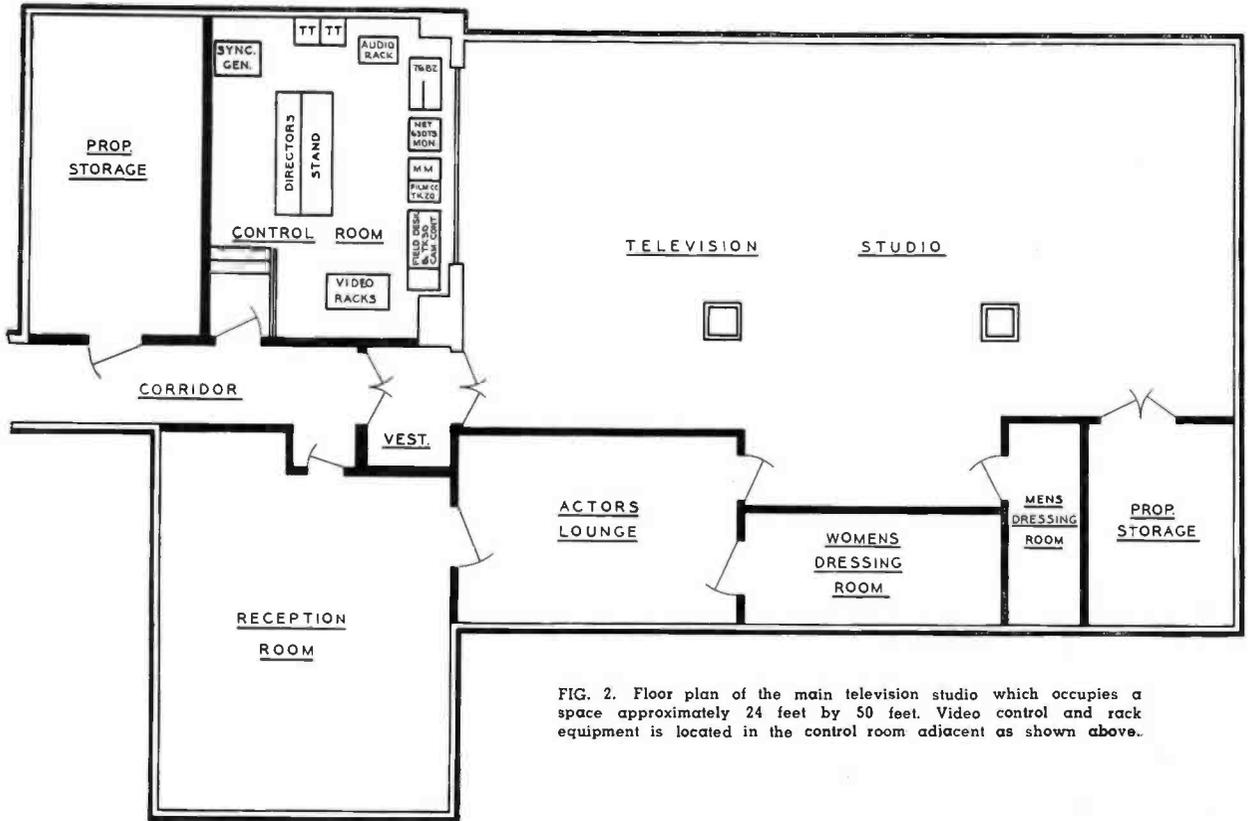
FIG. 2. Floor plan of the main television studio which occupies a space approximately 24 feet by 50 feet. Video control and rack equipment is located in the control room adjacent as shown above.
