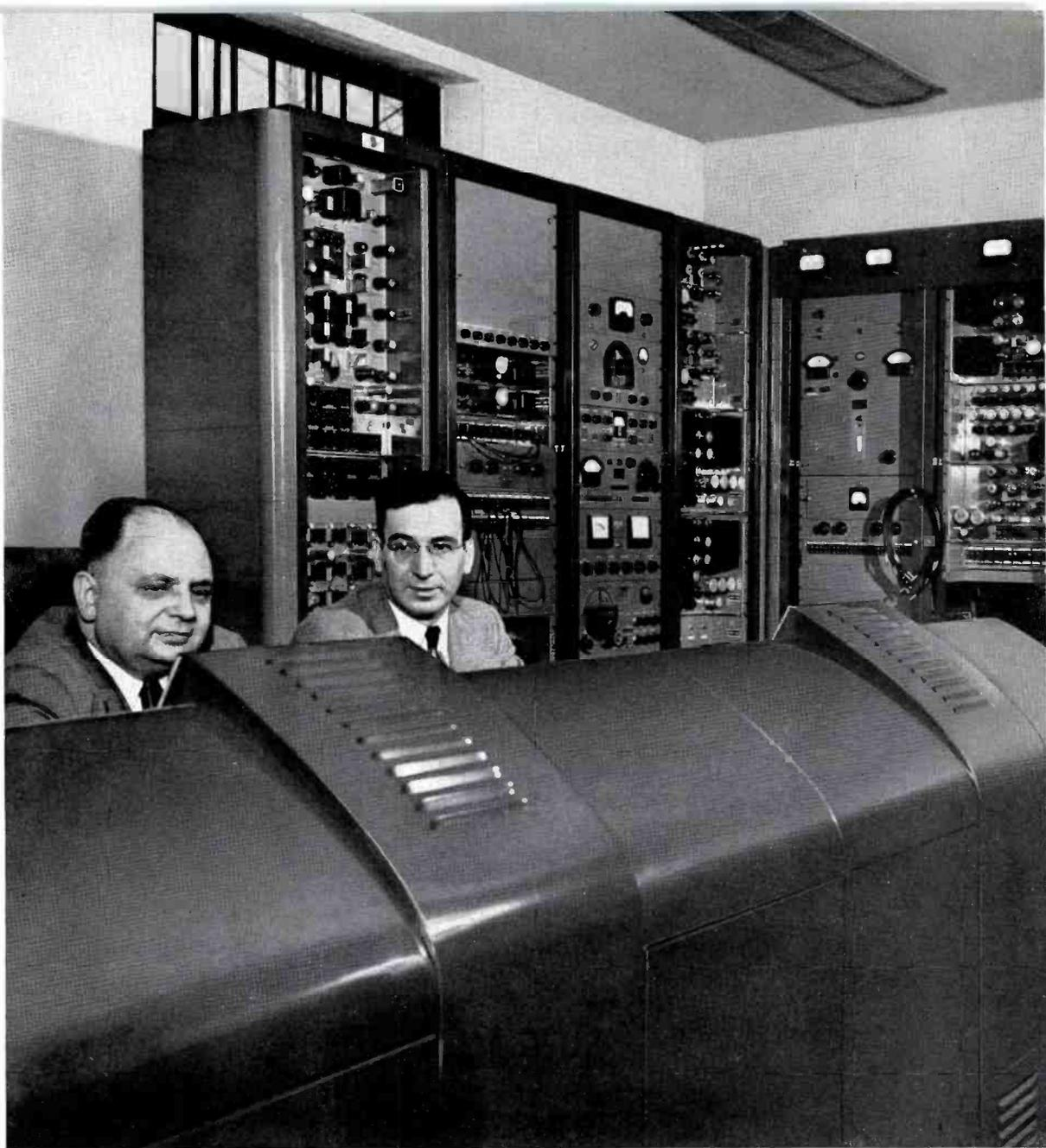
View from opposite side of transmitter room showing equipment racks arranged in one corner. Equipment consists of sync generator (left hand rack) audio and video patch panels, input and monitoring equipment, power supplies. Seated at the console with Nevin Straub is Ted Campbell, Assistant Chief Engineer.
