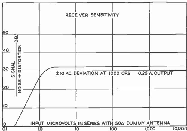
FIG. 14. Receiver sensitivity.
