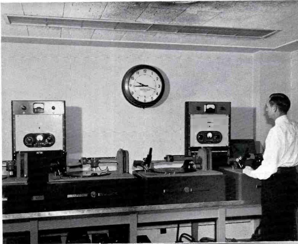
FIG. 2. The KSD Recording Studio which incorporates four RCA 73-B Professional Recorders in a compact, yet efficient, arrangement of equipment. Mr. Ray Herchert shown at the Recorder Console.
