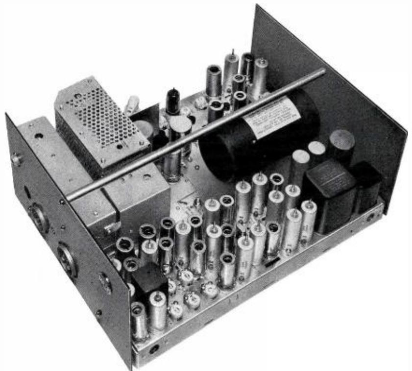
FIG. 3. The 30 watt RCA Super-Carlone, introduced recently, provides excellent performance in crowded metropolitan areas as well as farther out in the suburbs where the going is tough. Unique grounded-grid r-f input circuit provides high receiver sensitivity and simplified tuning.
