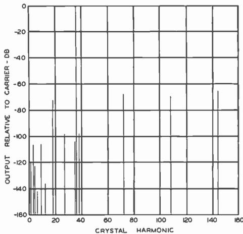
FIG. 21. Chart of spurious emissions of RCA Carbone transmitter, type CMV-1A, tuned to 158.31 mc.
