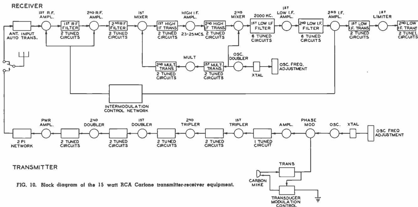
FIG. 10. Block diagram of the 15 watt RCA Carlone transmitter-receiver equipment.
