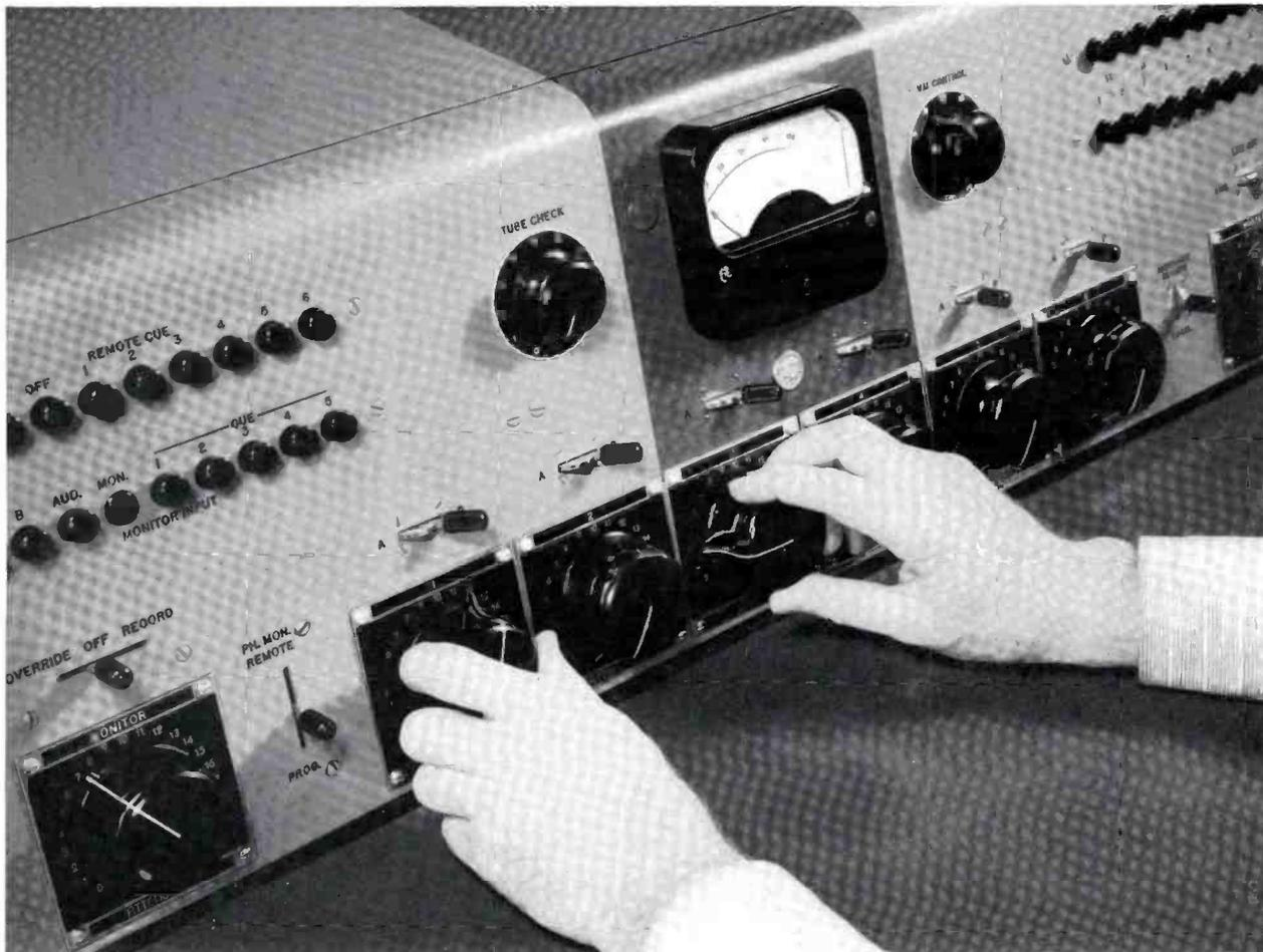
FIG. 2 (above). The RCA 76-B5 Consolette serves as an important part of the TV audio system. It incorporates four pre-amplifiers feeding a six-position mixer system.
