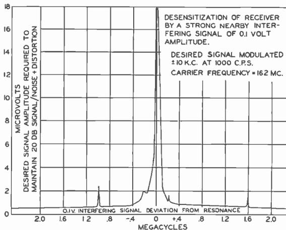
FIG. 15. Receiver spurious response rejection.
