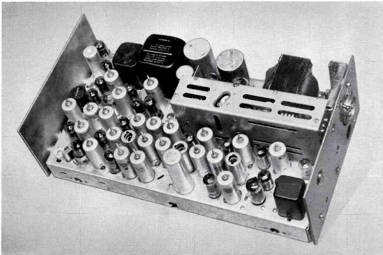
FIG. 1. The 15 watt RCA Carlone shown above, was the first adjacent channel two way radio equipment on the market. Completely open, accessible construction puts every component and every connection "on top". The unit can be removed for service in thirty seconds.
