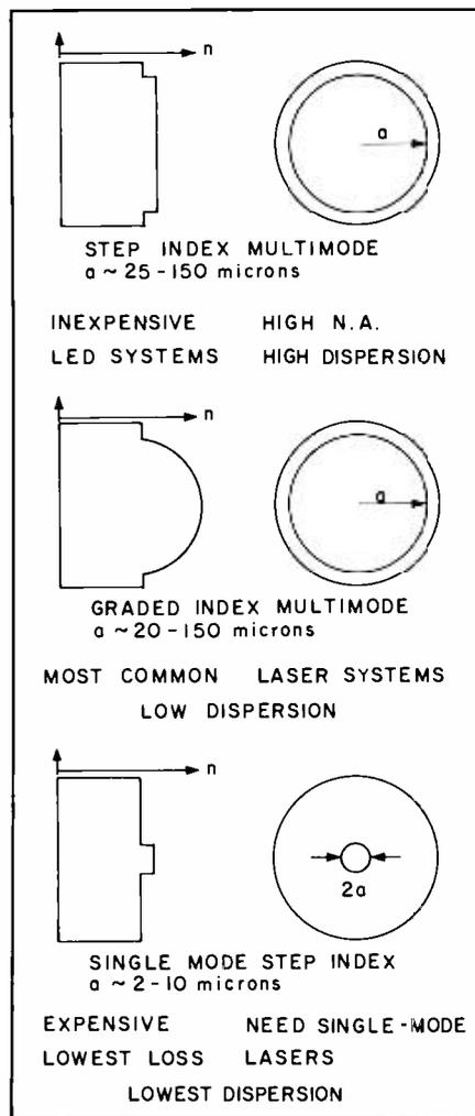
Fig. 2. Three main types of optical fibers.
