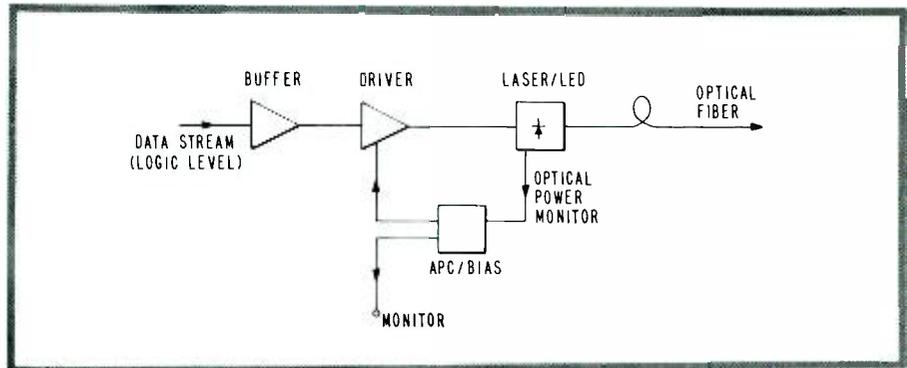
Fig. 16. Components of a fiber optic transmitting system.
