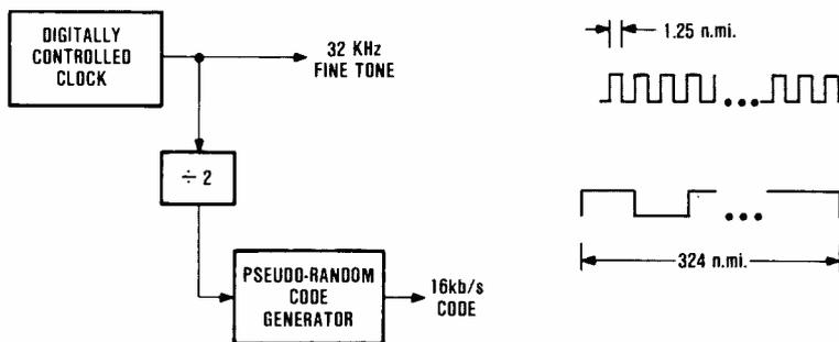
**Fig. 5. Ranging waveform generator and waveforms.** The ranging waveform combines a fine tone with a pseudo-random code. The fine tone provides accuracy by supplying many transitions for edge tracking. The pseudo-random code provides the equivalent of a coarse tone to resolve range ambiguities out to 324 nautical miles.
