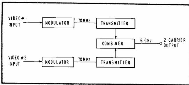
Fig. 5. Implementation of two-carrier system at transmitter site.
