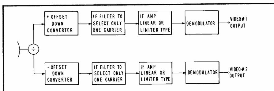
Fig. 10. Implementation of two-carrier system at receiver site.
