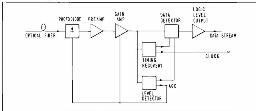
Fig. 18. Basic layout for an optical data receiver.
