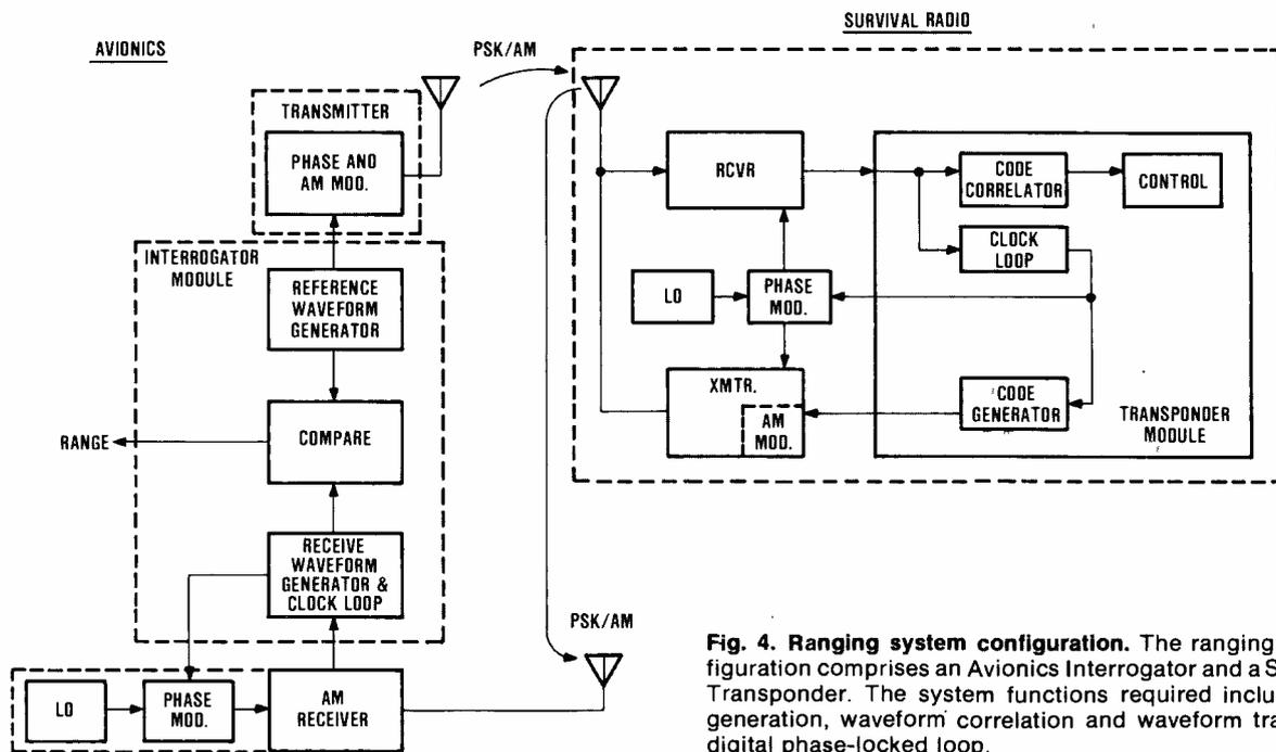
**Fig. 4. Ranging system configuration.** The ranging system configuration comprises an Avionics Interrogator and a Survival Radio Transponder. The system functions required include waveform generation, waveform correlation and waveform tracking with a digital phase-locked loop.
