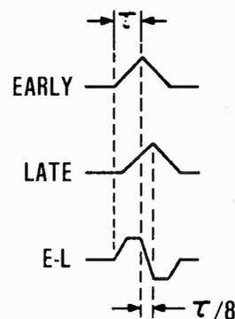
**Fig. 10. Early/late correlation function.** Advancing and delaying the system timing provides early and late correlation functions. When the early waveform is subtracted from the late waveform, a discriminator curve is generated which provides an error voltage of different polarities for early and late timing.
