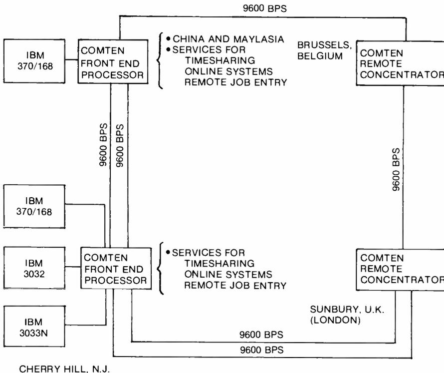
Fig. 5. Geographically dispersed customers can gain access to the IDN through the COMTEN nodes. In the event of line failure, alternate paths are automatically selected.
