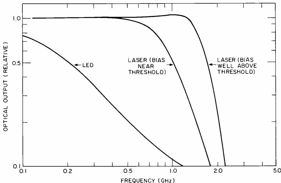
Fig. 8. Relative output versus frequency for LEDs and lasers.
