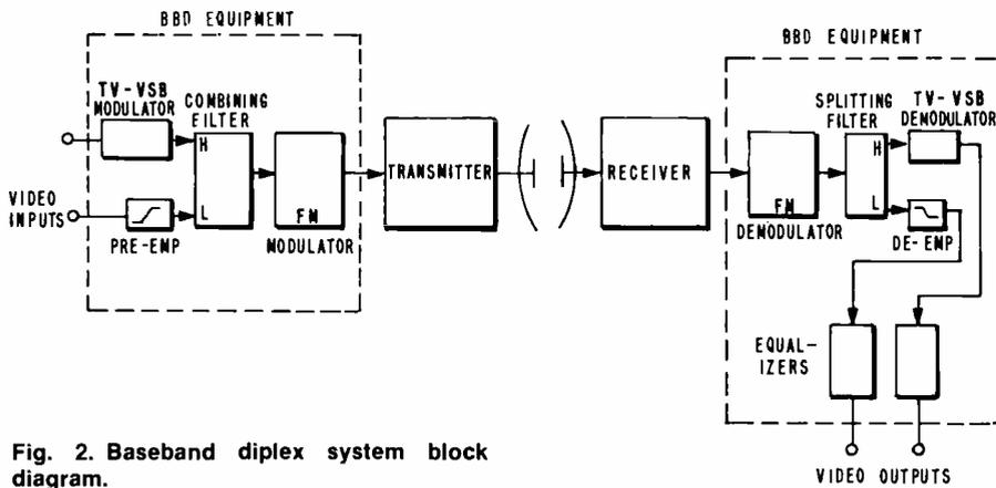
Fig. 2. Baseband duplex system block diagram.
