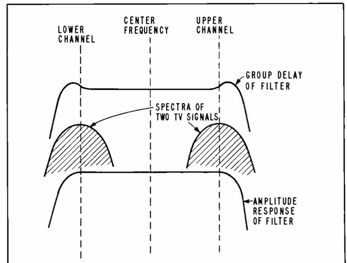
Fig. 16. FM to AM conversion mechanism for carriers with excessive spacing.
