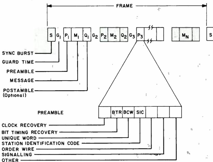
Fig. 4. Overhead in a time-division multiple-access (TDMA) system consists of bits used to label and control the blocks, as well as guard time between them.
