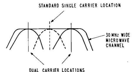
Fig. 4. Carrier locations for single-carrier and dual-carrier approaches.
