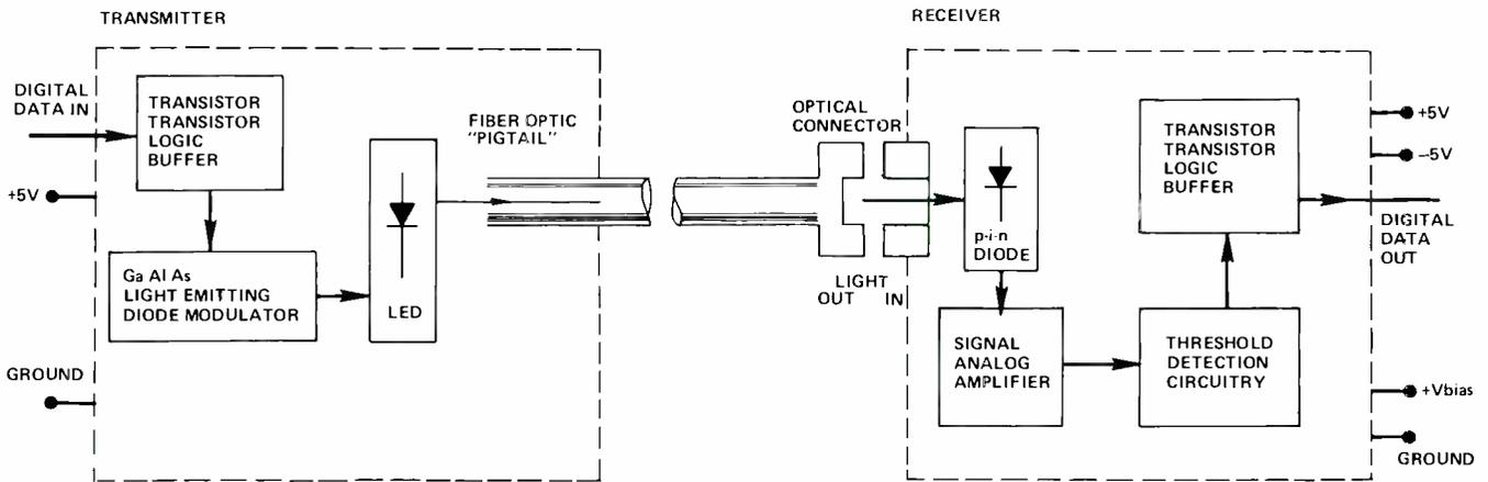
Fig. 10. Circuitry for device electronics used for RCA lasers and LEDs.
