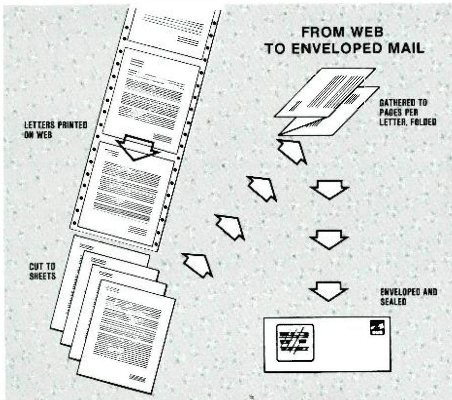
**Printing takes place along a web of sprocketed paper.** The letters are printed in sorted order. In the ETS, this can be down to a carrier's neighborhood-walk sequence. The envelope cuts the web into sheets; accumulates one, two or three sheets per letter; and folds, inserts and seals the letter in an envelope.
