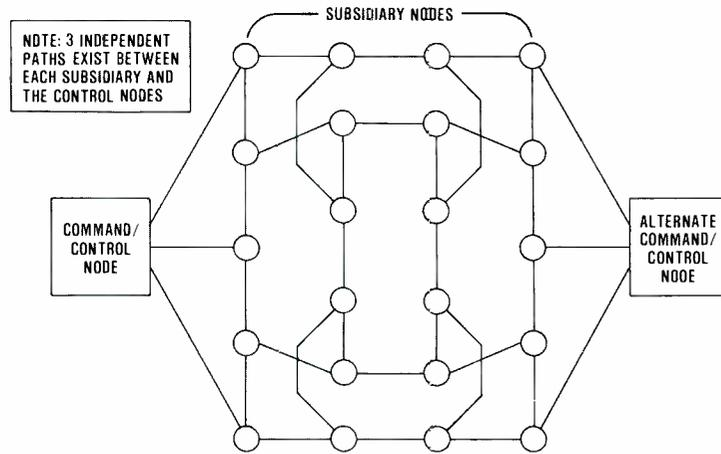
Fig. 1. Typical net connectivity.
