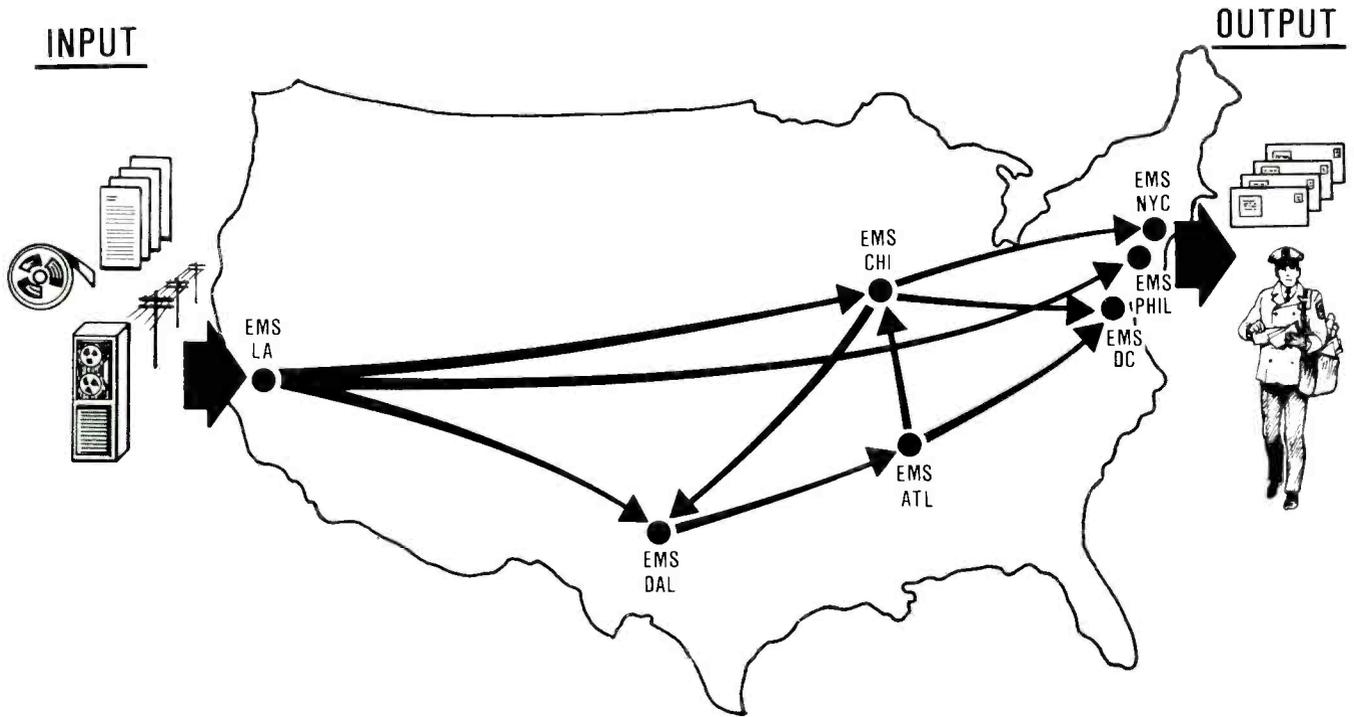
The RCA System Definition study projects a volume of 25-billion pieces per year for the mature electronic mail system. Inputs are on various media: paper, magnetic tape, floppy disk, and by communications. Output is an enveloped multi-sheet letter, postal carrier delivered.
