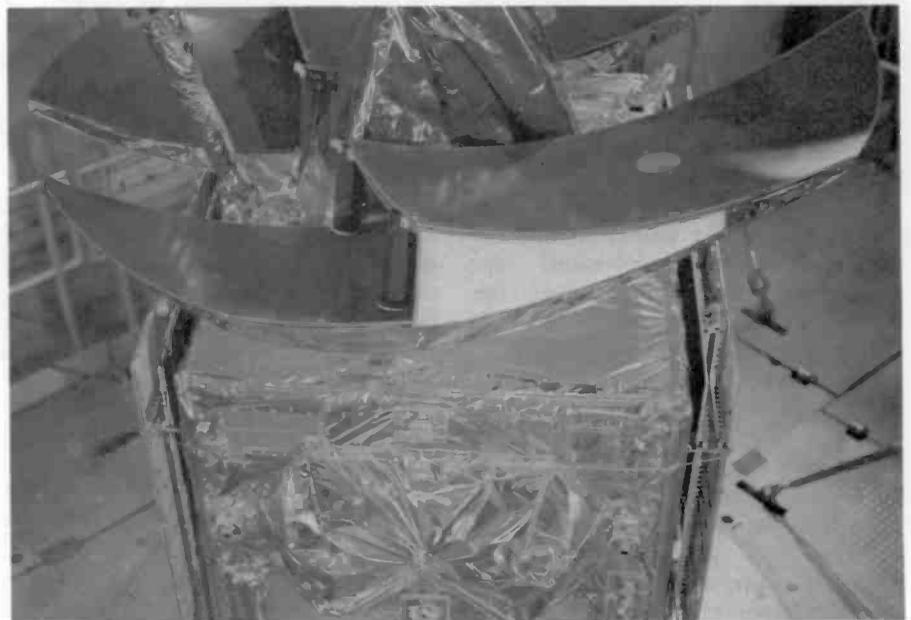
**Fig. 4. Kevlar/epoxy antenna reflector assembly of Satcom I. The assembly consisted of an embedded photo-etched polarizing grid structure, making each reflector segment transparent to r.f. energy of one polarization and reflective to energy of the opposite polarization. Similar Kevlar/epoxy composite designs were used for RCA-built ANIK-B satellite reflectors.**
