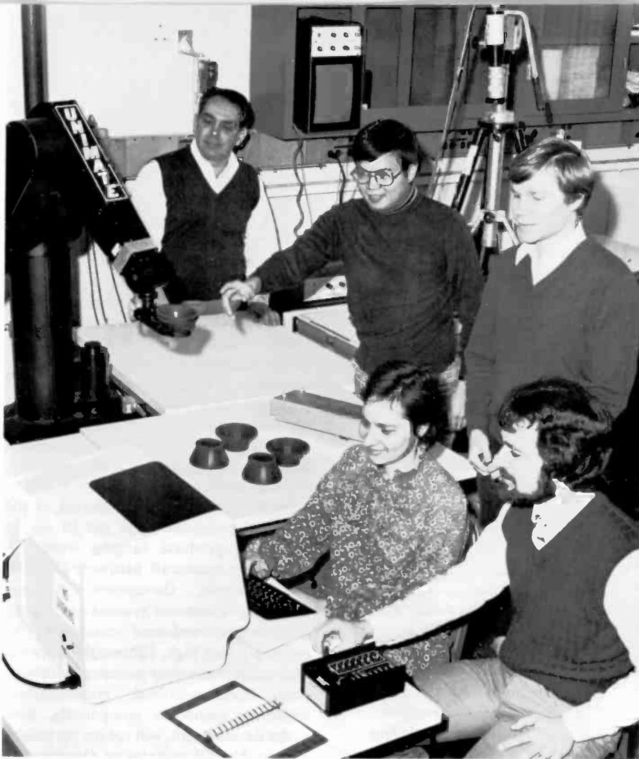
**Members of DSRC's robotics laboratory.** The Unimate 600 is used to conduct an exercise in handling deflection yoke parts. At the Unimate computer/controller are **M. Herman** (left) and **M. Martinez**. Looking on (left to right) are **S. Noto**, **D. Yang** and **H. Baird**. On the tripod is the CCD camera for the SRI image analyzer used to recognize parts.
