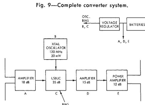
Fig. 9—Complete converter system.
