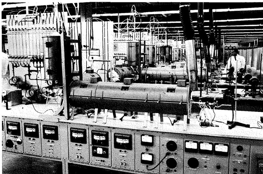
Fig. 3—View of production facilities at Harrison for vapor deposition of niobium stannide superconductive material. Cylindrical furnaces produce stoichiometric, single-phase pure Nb<sub>3</sub>Sn.
