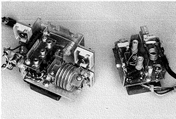
Fig. 7—The driver-power amplifier for the 50- and 150-MHz transmitters.
