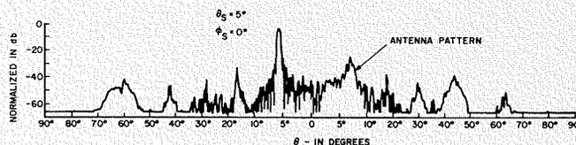
Fig. 2—Computed pattern (1000-element circular-grid array).
