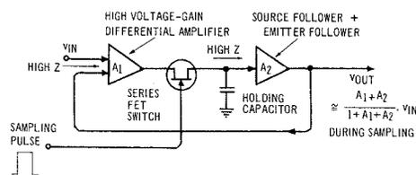
Fig. 5—Realization of the sample-and-hold circuit.
