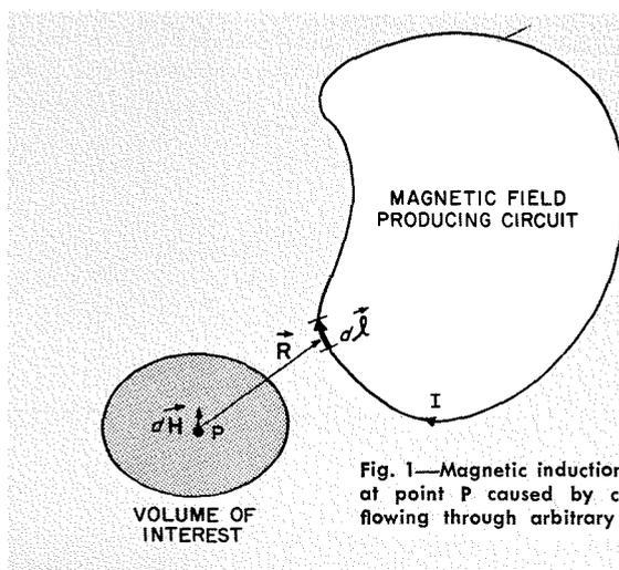
Fig. 1—Magnetic induction field at point P caused by current flowing through arbitrary loop.
