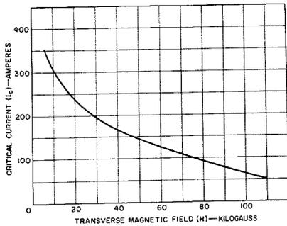
Fig. 1—Critical current as a function of transverse magnetic field for a nominal  $2.5 \times 10^{-4}$  inch vapor-deposited  $Nb_3Sn$  layer.
