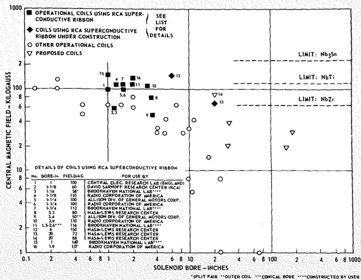
Fig. 1—Central magnetic field vs. superconductive solenoid bore for some existing and proposed magnets.
