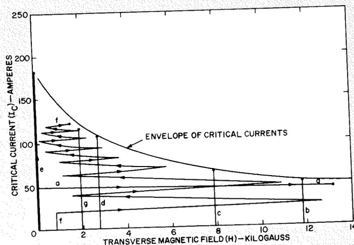
Fig. 1—Critical current vs. transverse magnetic field of Nb<sub>3</sub>Sn deposited on a platinum substrate.
