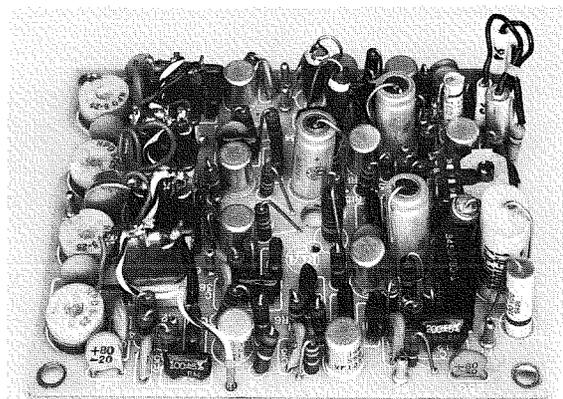
Fig. 4—High-band exciter printed-board assembly.
