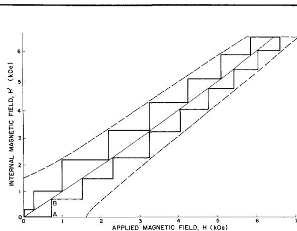
Fig. 4—Typical magnetization curve for a  $Nb_3Sn$  sample.
