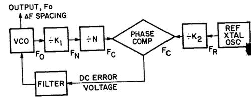
Fig. 1—Frequency synthesizer basic block diagram.
