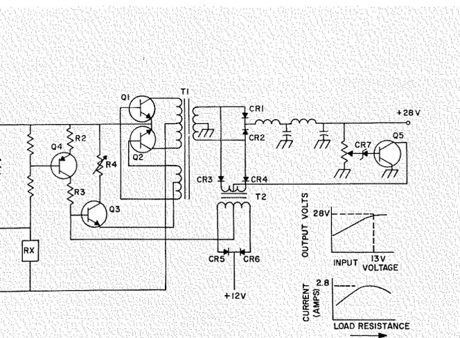
Fig. 14—Conventional square-wave DC-to-DC inverter circuit.
