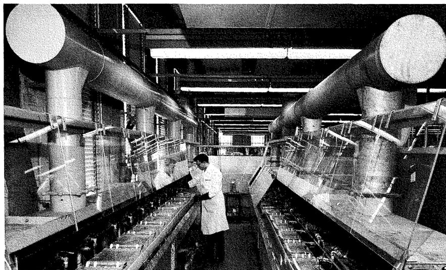
Fig. 4—View of production equipment used for electroplating a silver coating on the surface of the deposited Nb<sub>3</sub>Sn.
