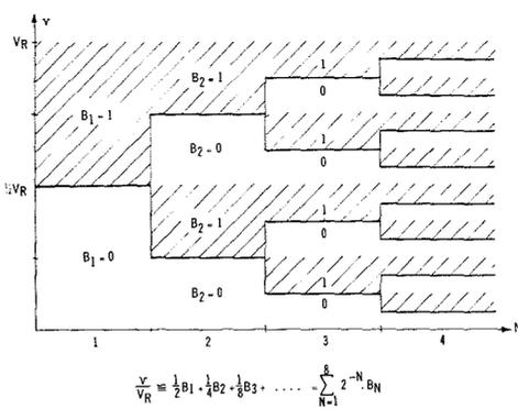
Fig. 7—Diagram illustrating the process of straight binary coding.
