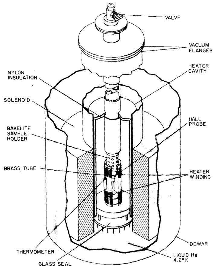
Fig. 1—Cross-sectional view of apparatus.
