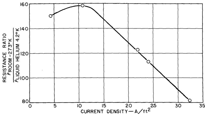
Fig. 3—Effect of plating current density on resistance ratio of silver.
