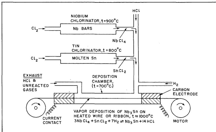
Fig. 2—Equipment used for production of  $Nb_3Sn$  superconductive ribbon by vapor deposition process.
