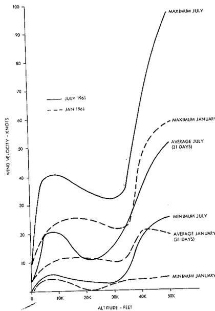
Fig. 4—Maximum, average, and minimum wind velocity vs. altitude, Southeast Asian jungle.
