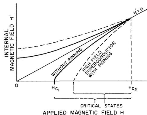
Fig. 2—Internal magnetic field ( $H'$ ) as a function of applied magnetic field ( $H$ ) with and without pinning.
