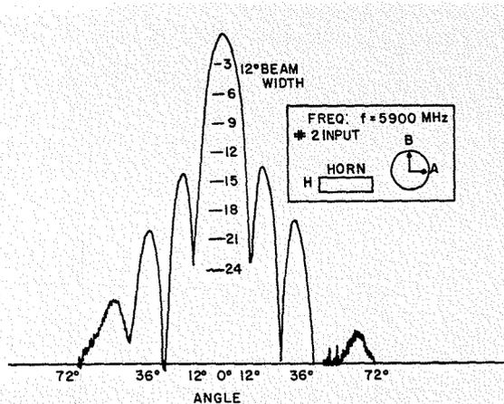
Fig. 7—Gain measurements on isolated antennule.
