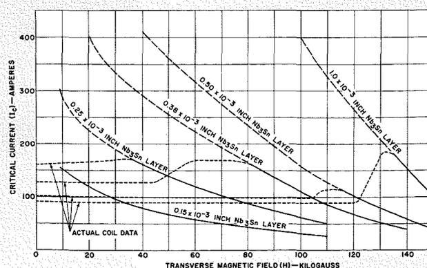
Fig. 5—Stability as a function of Nb<sub>3</sub>Sn layer thickness.
