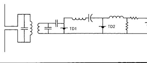
Fig. 10—Tunnel-diode transponder.
