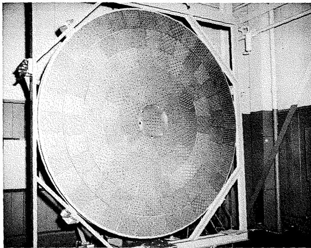
Fig. 4—Circular-grid array antenna model.
