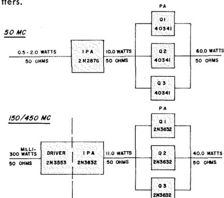
Fig. 9—Power amplifier simplified schematic.
