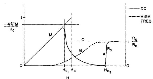
Fig. 4—Magnetization and resistive transitions for a type II superconductor.
