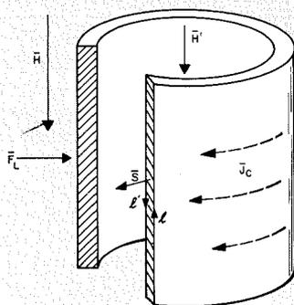
Fig. 3—An annular cylinder of known dimensions as used to determine  $J_c$  with  $H$  and  $H'$  known.
