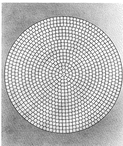
Fig. 1—Circular grid consisting of 18 concentric rings and 1048 antennules (30-foot diameter).
