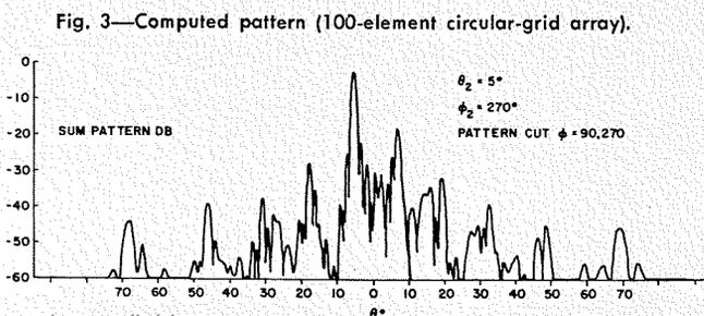
Fig. 3—Computed pattern (100-element circular-grid array).
