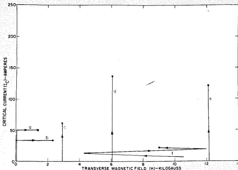
Fig. 2—Critical current vs. transverse magnetic field of Nb<sub>3</sub>Sn deposited on a stainless steel substrate.
