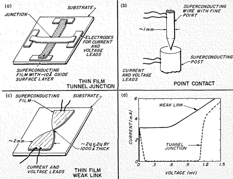
Fig. 7—Schematic diagrams depicting (a) a thin-film oxide-layer tunnel junction, (b) a point-contact weak-link junction, (c) a thin-film weak-link junction, and (d) the  $I-V$  curve of a weak link and the  $I-V$  curve of a tunnel junction displaying the dc Josephson current.
