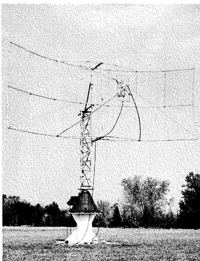
Fig. 3—The LOCOTAC unit showing reflector.
