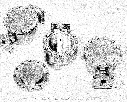
Fig. 6—A one- and a two-port X-band superconducting electroplated lead cavities.
