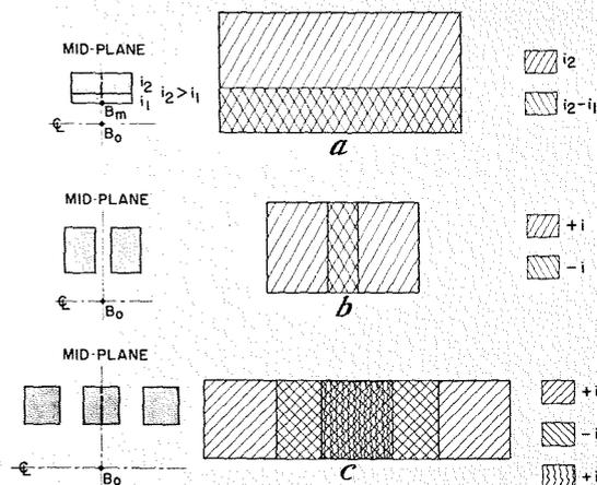
Fig. 4—Superposition of simple solenoids to simulate more complex magnets—(a) magnet with two different current densities, (b) window magnet ("split pair"), (c) system composed of three regularly spaced, identical, co-axial magnets.
