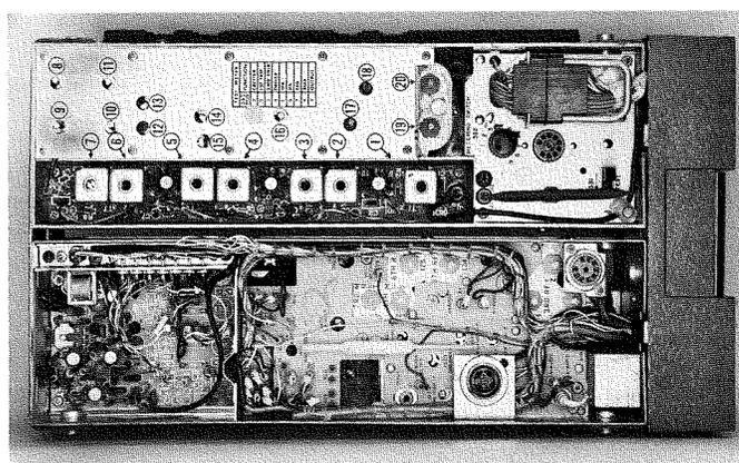
Fig. 15—The 150 MHz mobile unit with all modules in place.
