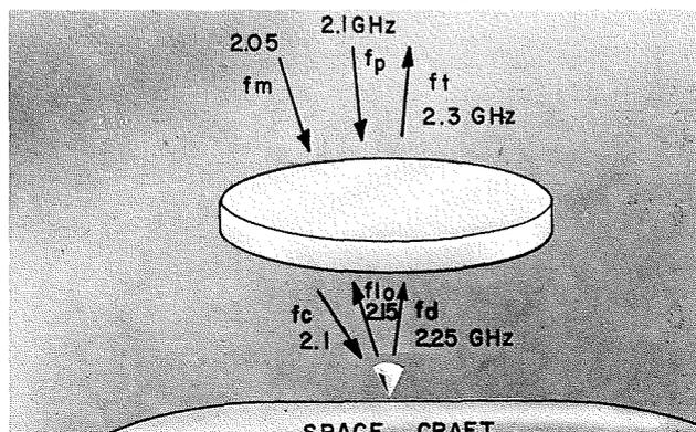
"OPTICAL" DISTRIBUTION OF INFORMATION AND LOCAL OSCILLATOR SIGNALS IN A RETRO-DIRECTIVE ARRAY
