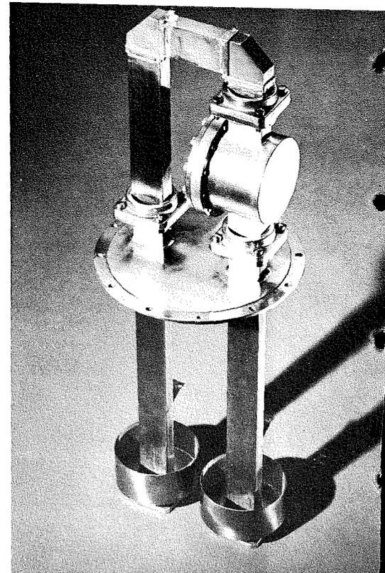
Fig. 7—An assembled X-band superconducting filter.
