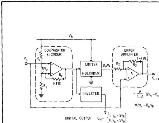
Fig. 6—One-bit encoder/decoder pair with error-detecting amplifier.
