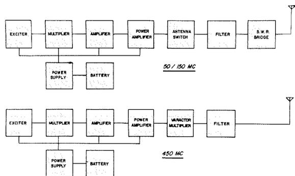
Fig. 2—Solid-state transmitters based on modular arrangements.
