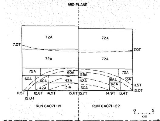
With these data the SIMPLE code can be used to find the required dimensions for the equivalent, uniform-current-density magnet. For the present case, field homogeneity is not specified; therefore, the geometric shape requiring the minimum amount of conductor is used for the initial equivalent magnet, as shown by the outline of Fig. 6.
