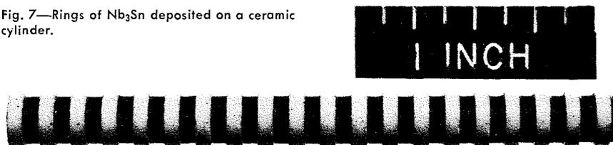
and the use of considerably less magnet-support structure to contain the stresses of high fields. For example, the ultimate tensile strength of a composite ribbon composed of  $Nb_3Sn$ , 0.00025-inch thick deposited on stainless steel 0.002-inch thick is 95,000 psi at room temperature.
