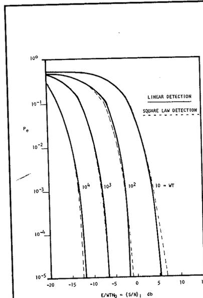
Fig. 1—Comparison of linear and square law envelope detection for wideband FSK systems.
