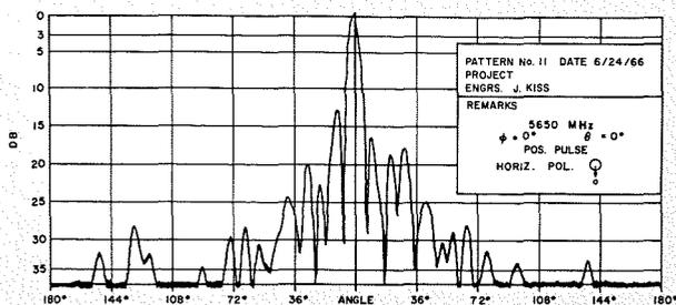
Fig. 8—Measured pattern, 100-element circular-grid array, scan angle 0 degrees.
