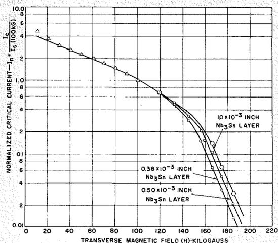
Fig. 4—Normalized critical current as a function of transverse magnetic field. (Based on results obtained by the author at M.I.T., June 1966.)
