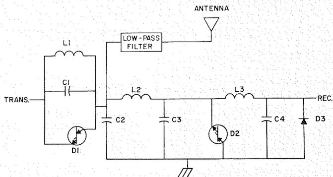
Fig. 11—RF activated antenna switch.
