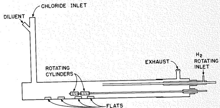
Fig. 4—Schematic diagram of apparatus used for a static deposition of  $\text{Nb}_3\text{Sn}$  on ceramic substrates.
