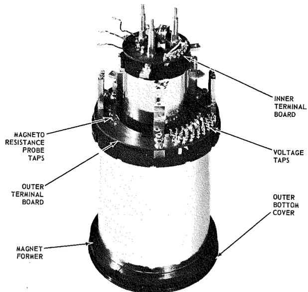
Fig. 2—Photograph with cover removed of first compound superconductive magnet having a field above 100 kilogauss and a bore size of 1.28 inches and a field of 55 kilogauss in a bore size of 3.375 inches. The maximum central field value for this magnet is 112 kilogauss in the 1.28-inch bore.
