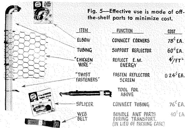
Fig. 5—Effective use is made of off-the-shelf parts to minimize cost.
