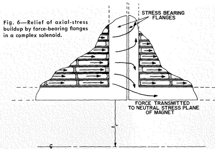
Fig. 6—Relief of axial-stress buildup by force-bearing flanges in a complex solenoid.
