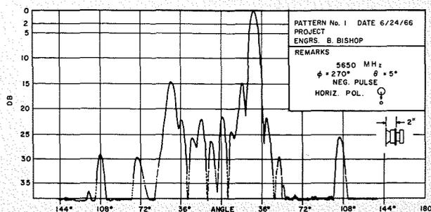
Fig. 9—Measured pattern, 100-element circular-grid array, scan angle 5 degrees.
