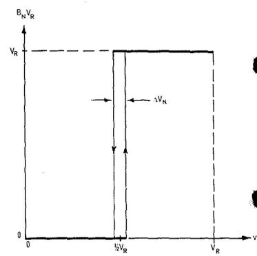
Fig. 8—The  $(v_N, B_N V_R)$  transfer function.
