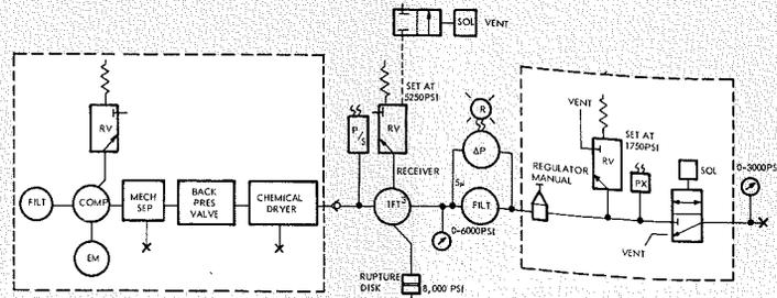
Fig. 13—Hydraulic test system—truck-mounted configuration
