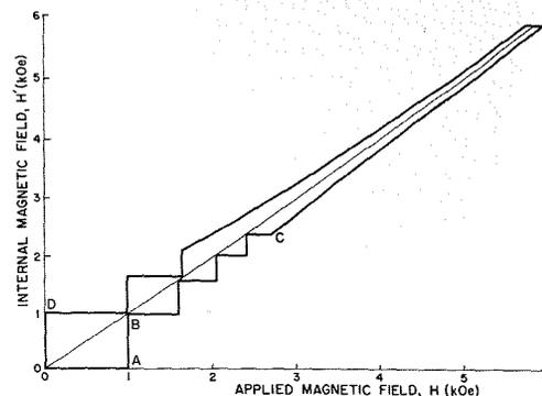
Fig. 6—Magnetization curve for  $Nb_3Sn$  at higher temperature.
