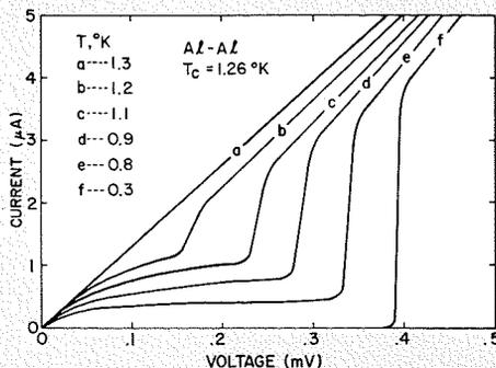
Fig. 4—Typical normal-electron  $I$ - $V$  curves for a superconducting tunnel junction composed of bottom and top films of the same superconductor. The onset of the sharp break in the curves for  $T < T_c$  occurs when  $eV = 2\Delta(T)$ .
