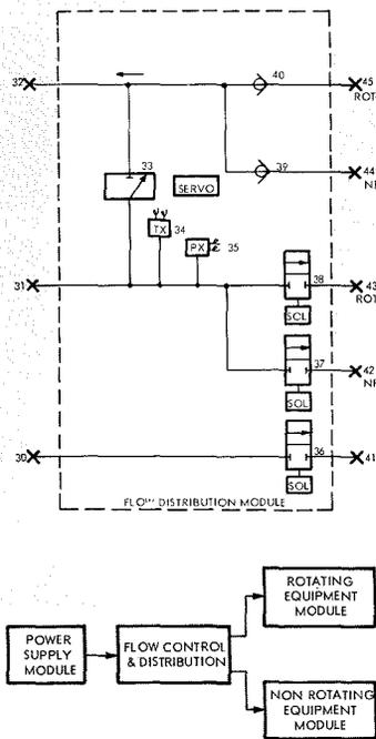
Fig. 9—Hydraulic schematic—flow distribution module
