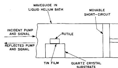
that of the Esaki diode by a factor of 20 or so because of the smaller current in the superconducting device (the major contribution to the noise is probably shot noise).
