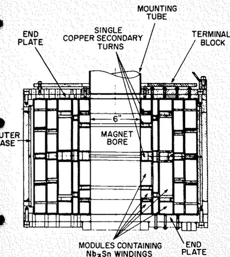
Fig. 7—Cross section view showing mechanical design of a 150-kilogauss magnet with a 6-inch bore.
