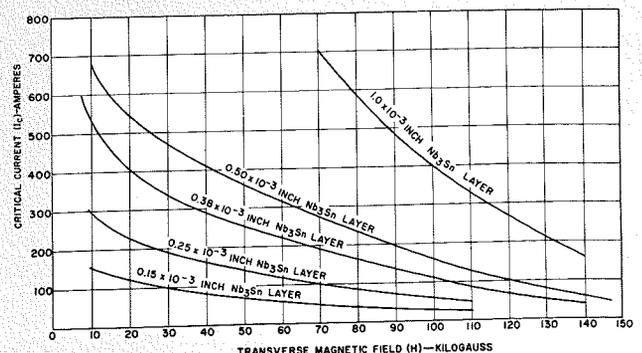
Fig. 3—Critical current as a function of transverse magnetic field for various thicknesses of  $Nb_3Sn$ .
