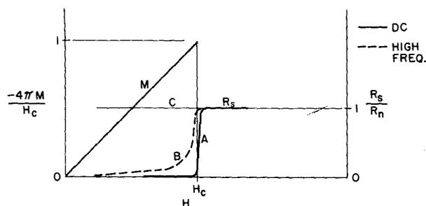
Fig. 3—Magnetization and resistive transitions for a type I superconductor.
