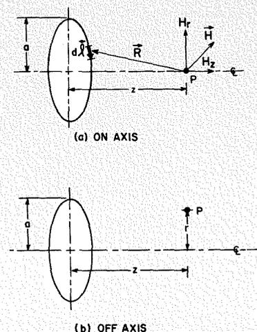
Fig. 2—Magnetic field at point P of a circular filament, (a) on geometric axis and (b) off axis.
