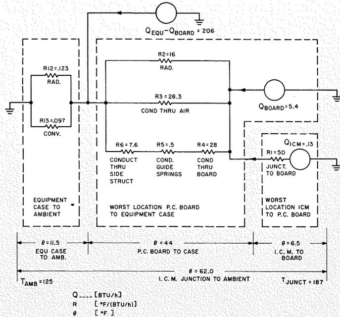
Fig. 5—Thermal diagram of equipment when forced air recirculation inside of equipment case is added.
