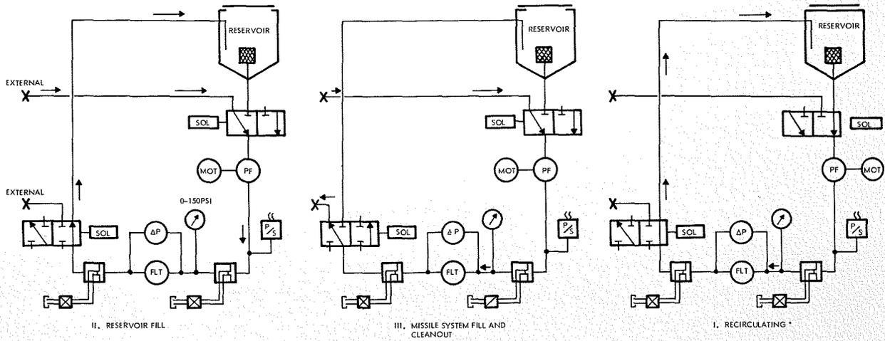
Fig. 8—Fill and filtering section—power supply module
