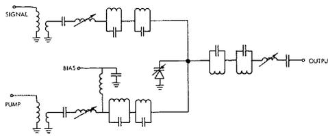
Fig. 8—Converter circuit configuration.
