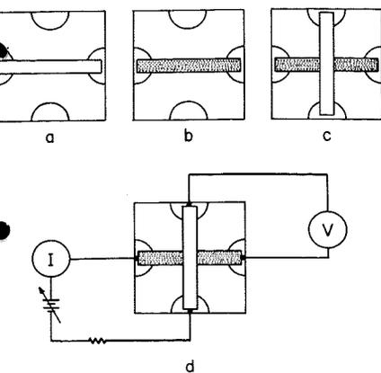
Fig. 3—Step by step procedure for fabricating superconducting tunnel junctions: (a) deposition of the bottom film in strip form (about 0.25 mm wide by 2000Å thick) onto a substrate (1" square) with pre-evaporated electrodes; (b) oxidation of the surface of this film in air or oxygen to a thickness of about 10-20 Å; (c) deposition of a top strip similar to the bottom strip, forming a junction; (d) measurement of the current-voltage (I-V) curve of the junction.
