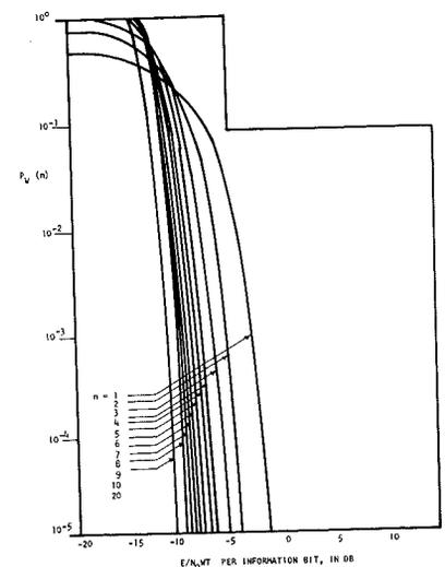
Fig. 2—Word error probability  $P_w(n)$  versus channel SNR per information bit for FSK systems using square law detectors.
