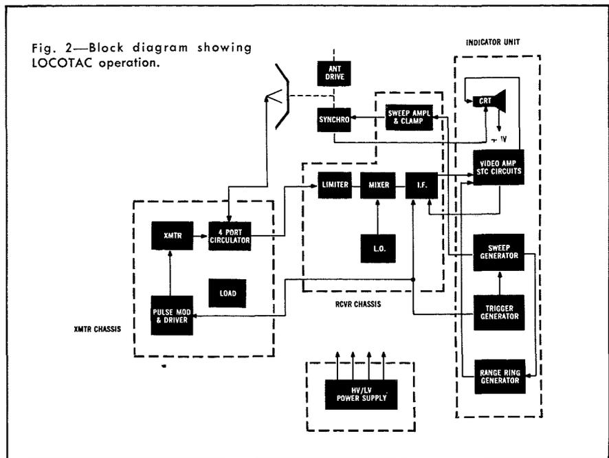
Fig. 2—Block diagram showing LOCOTAC operation.
