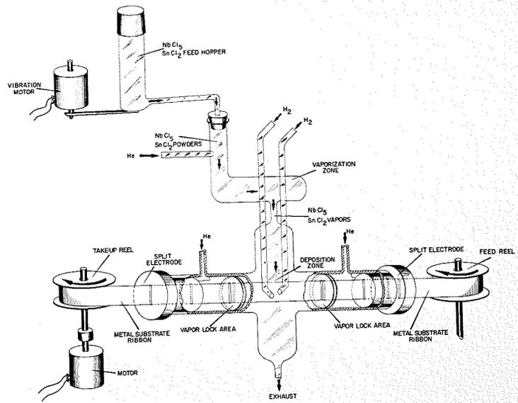
Fig. 3—Diagram of equipment used for production of wide superconductive ribbon.
