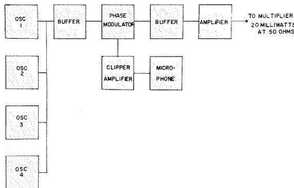
Fig. 3—The exciter provides four-channel operation with individual oscillators.
