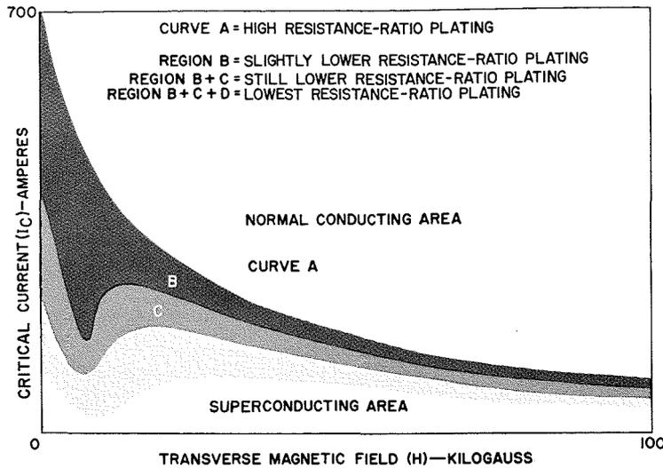
Fig. 5—Effect of plated-metal resistivity ratio on short-sample stability.
