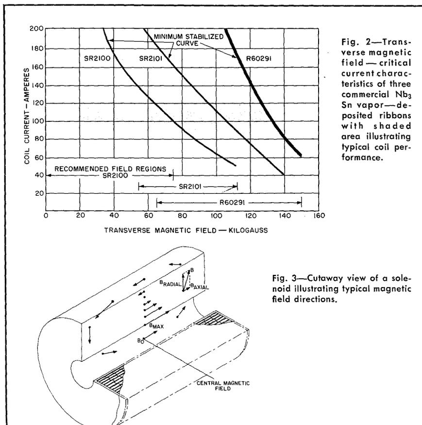
Fig. 2—Transverse magnetic field—critical current characteristics of three commercial Nb<sub>3</sub>Sn vapor-deposited ribbons with shaded area illustrating typical coil performance.
