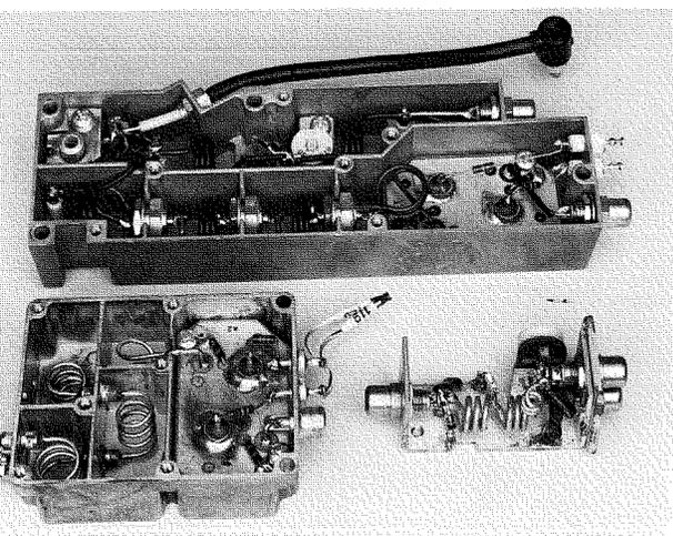
Fig. 12—Antenna switch, filter and reflectometer circuit.
