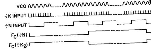
Fig. 2—Voltage waveform in frequency synthesizer.
