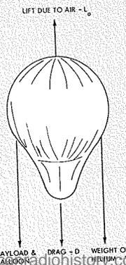
where  $P_h$  and  $P_a$  are the helium and ambient air pressures, and  $T_w$  and  $T_c$  are the warm and cold temperatures. When the balloon is inflated to this higher pressure, any temperature change will not cause it to go slack. For example, a super-pressure of 64 mbar will keep the volume of a balloon constant if it is flying at a pressure of 900 mbar with a daytime temperature of 300° ABS and a night temperature of 280° ABS.
