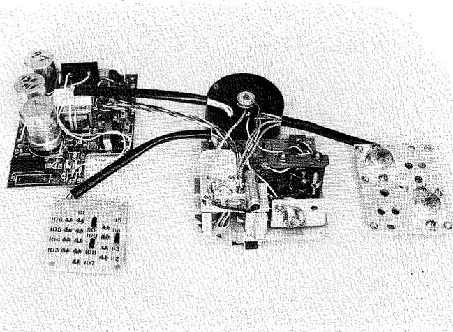
Fig. 13—The 50 MHz transmitter power supply.
