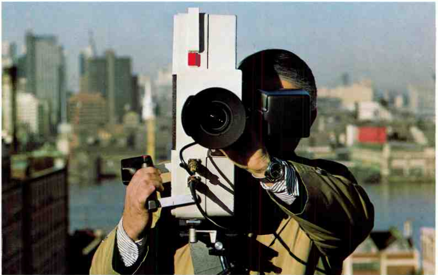
RCA's newest commercial color TV camera weighs less than 20 pounds and provides the picture quality of much larger studio cameras.
