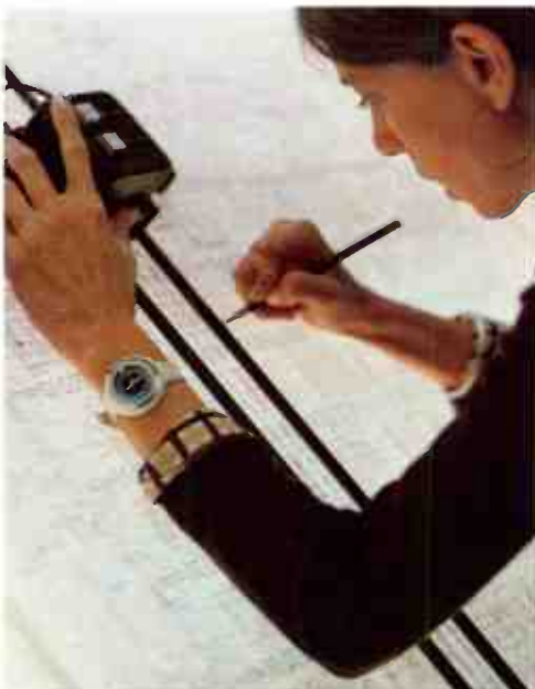
Elements of an integrated circuit are plotted at Solid State plant in Somerville, N.J.
