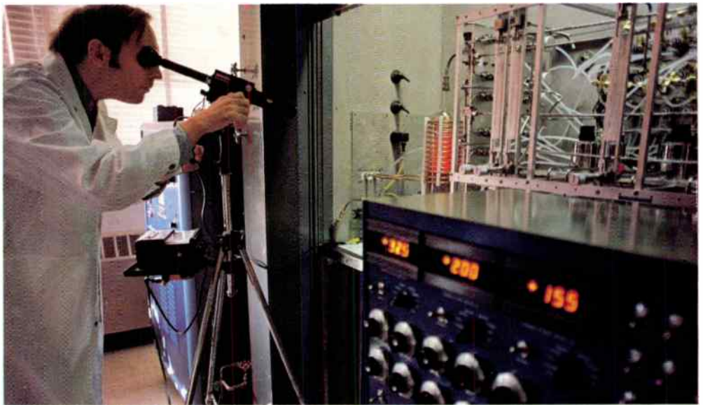
Scientist studies growth of an experimental crystal using radio-frequency heating device.
