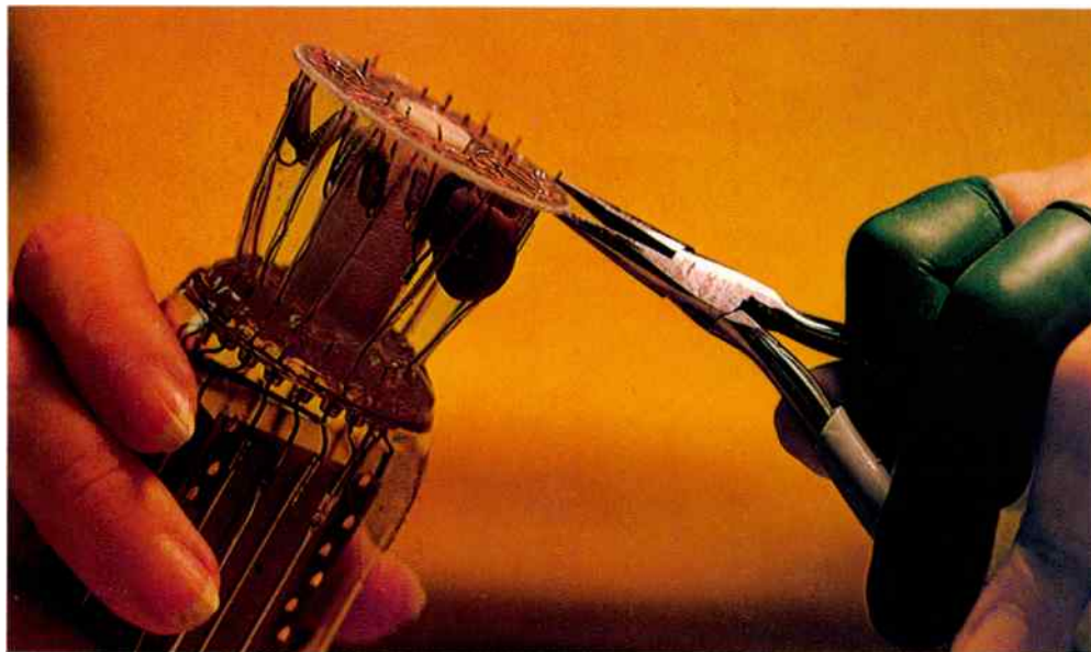
Photomultiplier tubes are assembled at Electronic Components plant in Lancaster, Pa.
