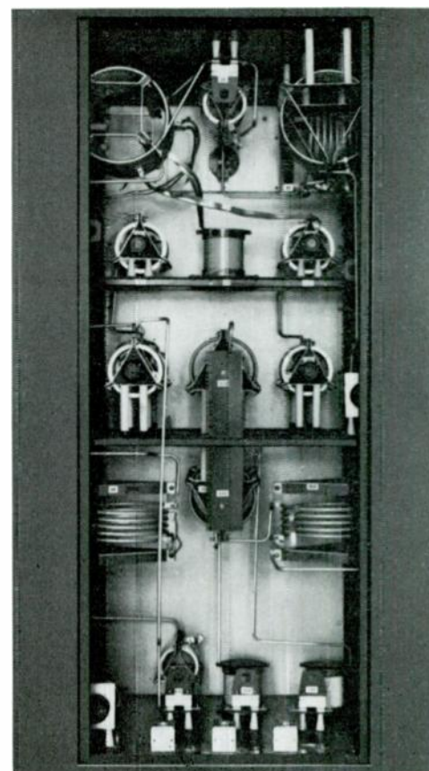
FIG. 9. Phasing equipment for a three-tower system.
