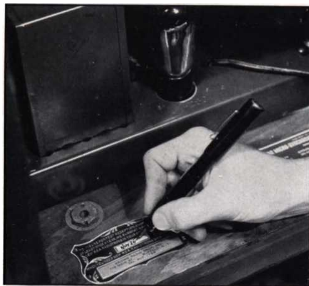
Write date on which tubes should next be renewed on celluloid strip. Easily erased
