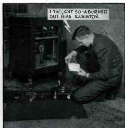
8. Use the RCA Radiotron Reference Book's circuit analysis chart to help you quickly locate the trouble
