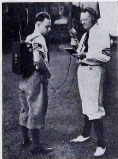
Fig. 2—1930 model pack-set in use for broadcast of American Open Golf Championship Tournament. Note antenna, approximately quarter wave, bent in form of loop.
