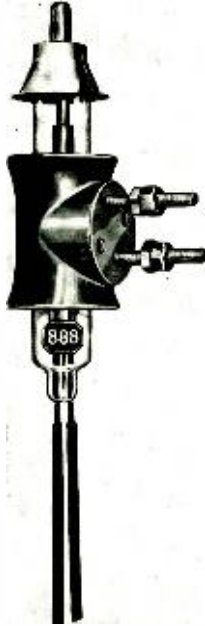
Fig. 1—Water-cooled high-frequency triode, RCA 888 750 watts Class C output. Overall length is 7 inches from top of grid post to near end of flexible filament leads.
