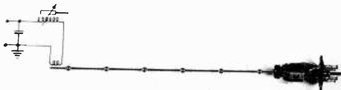
Fig. 5—Typical drive and take-off arrangement for magnetostrictively operated filters.
