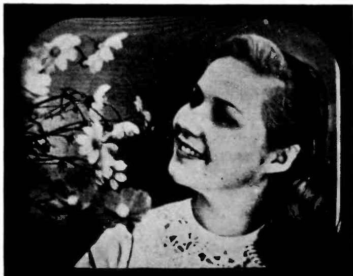
Fig. 10—Half tone transmitted by an experimental image isocon.
