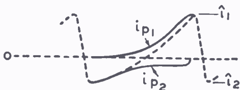
Fig. 5c—Waveform distortion increasing the average value of i_{p2} .
