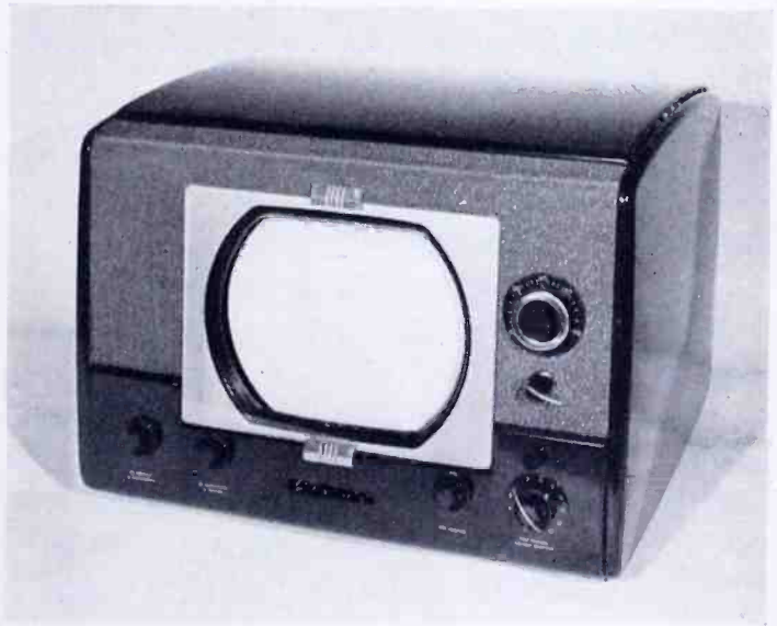
Fig. 13—Standard VHF receiver with UHF tuner added. UHF controls are to the right of the kinescope.
