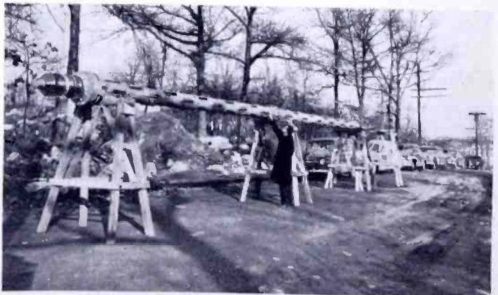
Fig. 11—The RCA TFU-20A UHF antenna in test position before erection on tower.
