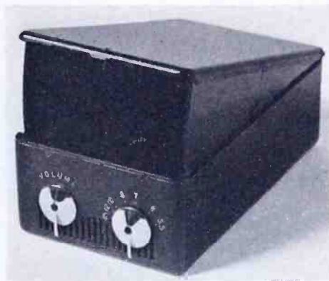
Fig. 15—Photograph of the laboratory personal receiver model 1 with the lid open forming the horn which is the operating condition.
