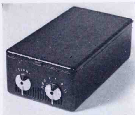
Fig. 14—Photograph of the laboratory personal radio receiver model 1 with the lid closed. Dimensions: 6'' \times 3\frac{3}{8}'' \times 2\frac{1}{32}'' .
