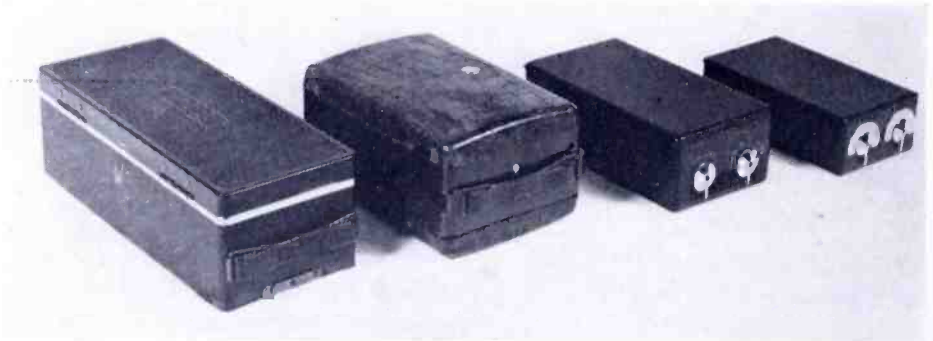
Fig. 19—Photograph of the RCA-BP10 and RCA-54B commercial personal radio receivers and the two laboratory models, 1 and 2.
