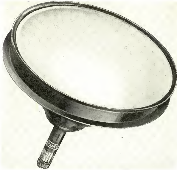
Fig. 1—Photograph of 21AXP22 color kinescope.
