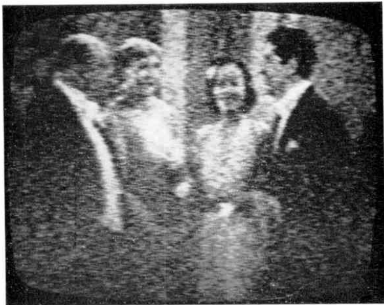
Fig. 19—Photographs of pictures displayed on UHF television picture tube: top picture received with point-contact diode frequency converter at input of receiver, and bottom picture received with tunnel-diode frequency converter at input of receiver.
