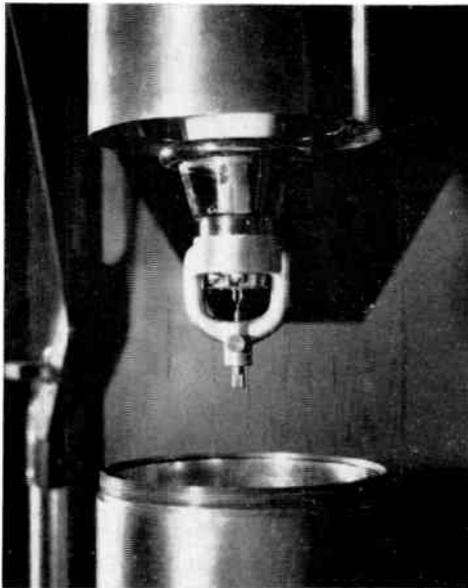
Fig. 14—Jig for positioning filament in the gun assembly.
