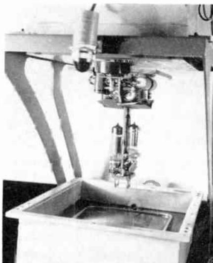
Fig. 18—Pulse circuit attached to transformer and ready to be inserted in the bottle and oil bath.
