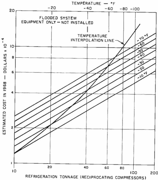
Fig. 9—Estimated refrigeration costs (1968) as a function of temperature.
