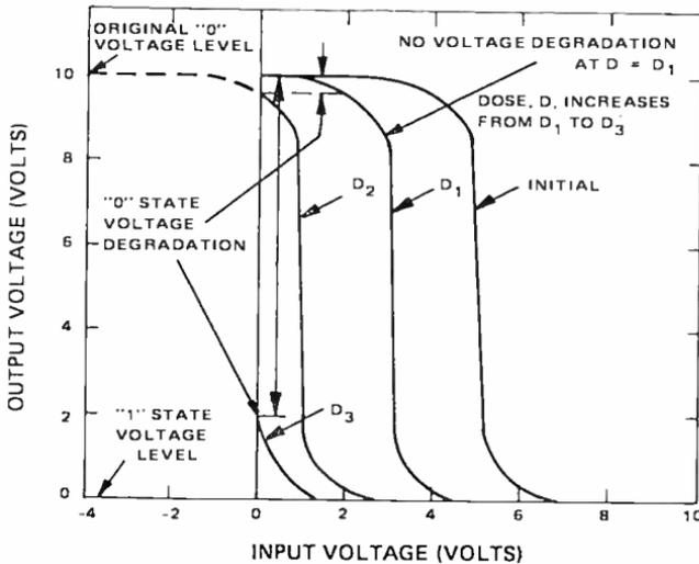
Fig. 8—Permanent radiation-induced shifts in the transfer characteristics of a complementary-symmetry MOS inverter.
