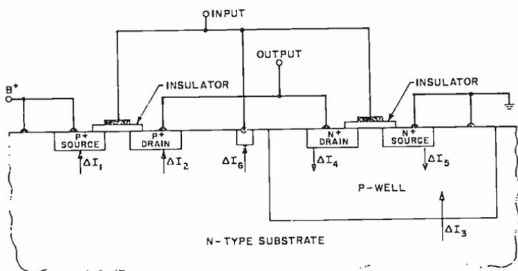
Fig. 11—Model for analyzing transient response of CMOS circuit.
