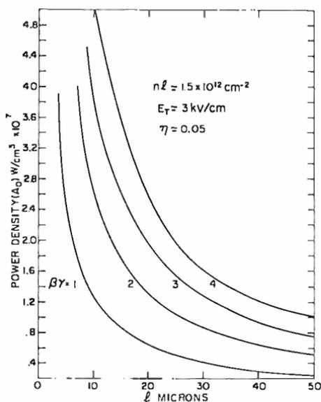
Fig. 2—Variation of input power density with layer thickness.
