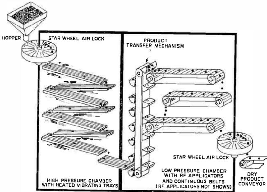
Fig. 11—Composite continuous freeze-drying chamber.
