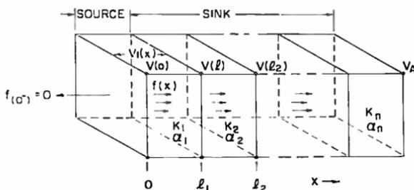
Fig. 3—Cascaded thermal network.
