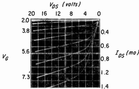
Fig. 6—Typical drain characteristics of the p-type MOS transistors.
