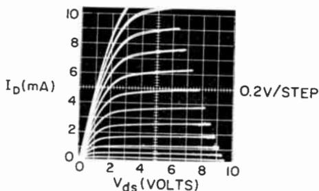
Fig. 17—Typical  $\text{Al}_2\text{O}_3$  MOS transistor characteristic.
