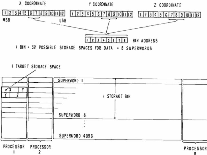
Fig. 9—Memory organization for scintillation test.
