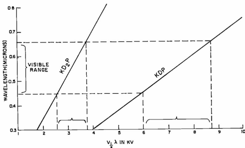
Fig. 16— $V_{\lambda/2}$  versus wavelength.
