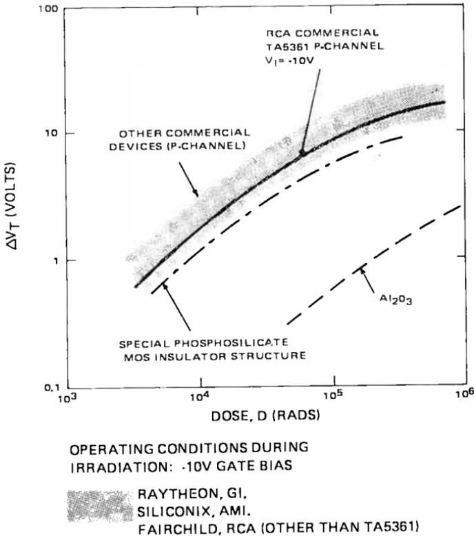
Fig. 7—Typical radiation-induced threshold voltage shifts.
