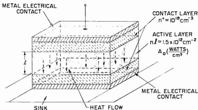
Fig. 1—Layered geometry of a TEO Gunn bulk-effect device.
