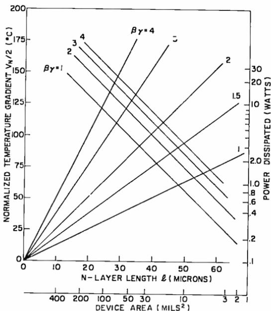
Fig. 7—Steady-state temperature gradient and average power dissipated in active n-layer with a thermal conductivity  $K_1 = 0.5$  watts/°C-cm.
