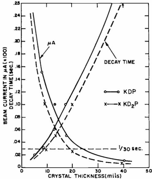
Fig. 17—Decay times versus crystal thickness (measured).
