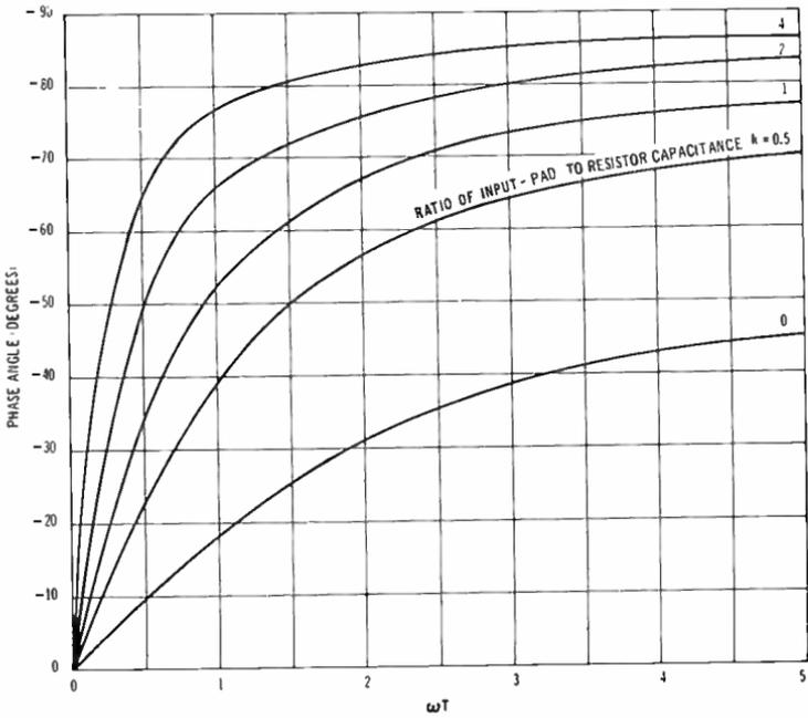
Fig. 3—Resistor phase angle as a function of normalized frequency.
