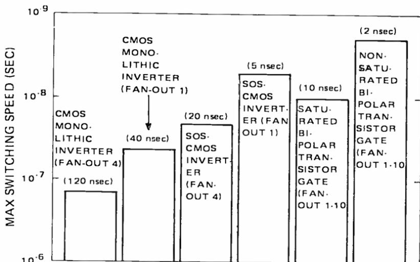
Fig. 5—Comparison of the maximum switching speeds of MOS, bipolar, and other micrologic.
