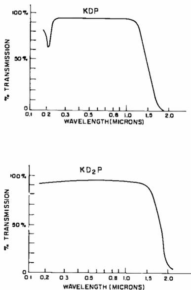
Fig. 2—Transmission characteristic for KDP and KD<sub>2</sub>P.
