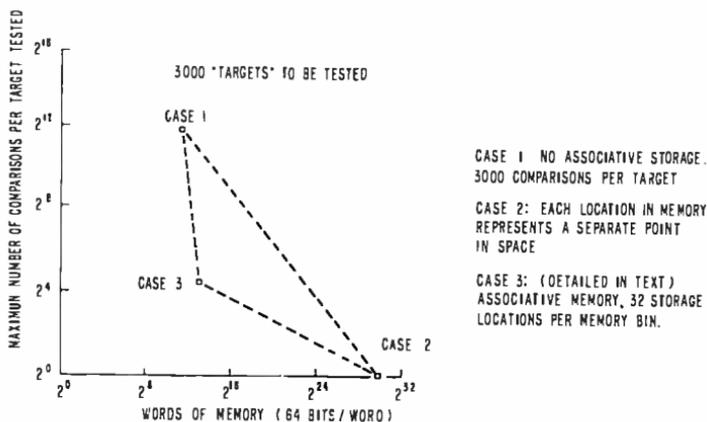
Fig. 11—Comparison of mechanizations for scintillation test.
