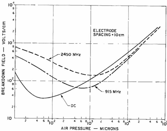
Fig. 6—Vacuum voltage-breakdown field strength as a function of dry air pressure for dc, 915 MHz, and 2450 MHz. The breakdown field is expressed in peak volts/cm.
