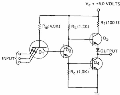
Fig. 4—Schematic diagram of a typical  $T^2L$  logic gate.
