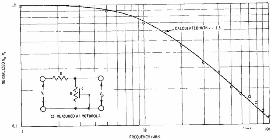
Fig. 4—Experimental verification of resistor model.
