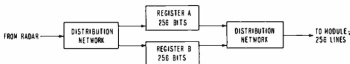
Fig. 4—I/O interface for one module.
