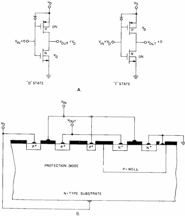
Fig. 1—(Top) Schematic diagram of CMOS inverter circuit and (bottom) cross-section of typical monolithic complementary pair of MOS transistors.
