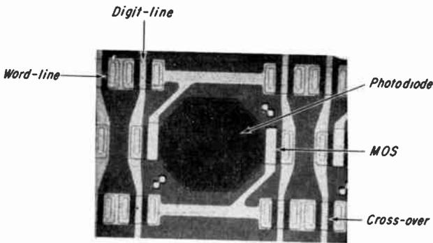
Fig. 4—Detailed photomicrograph of a photodetector cell (85  $\times$ ).
