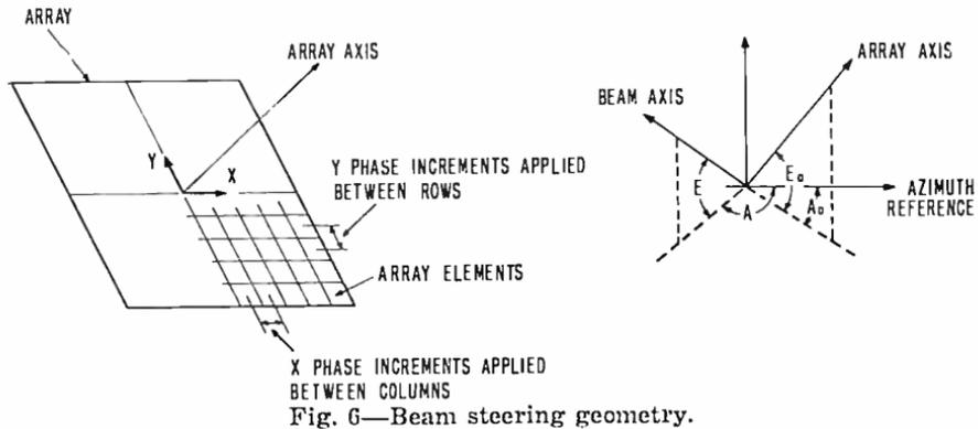
Fig. 6—Beam steering geometry.
