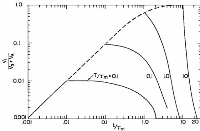
Fig. 8—Single pulse response.
