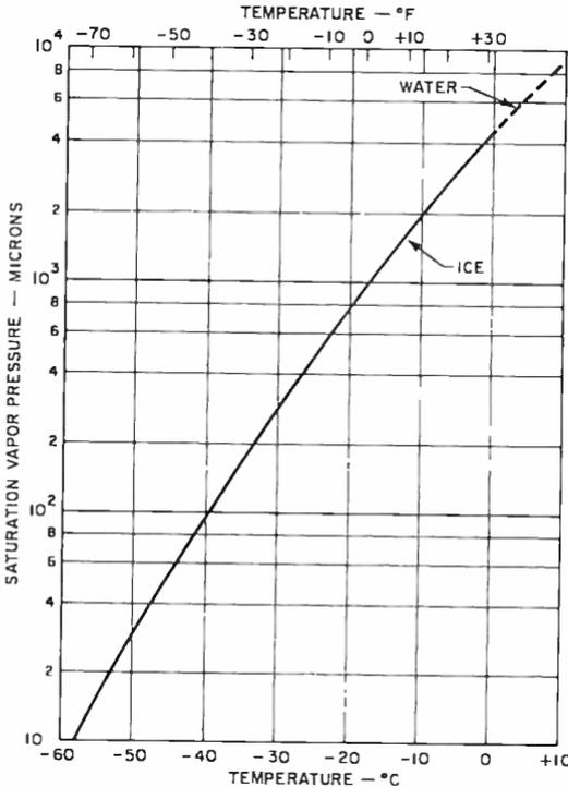
Fig. 8—Saturation vapor pressure as a function of temperature for pure water.
