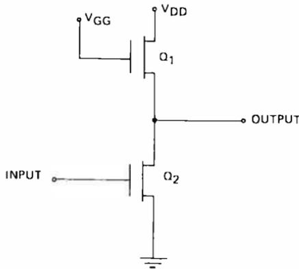
Fig. 2—Schematic diagram of basic PMOS inverter circuit.
