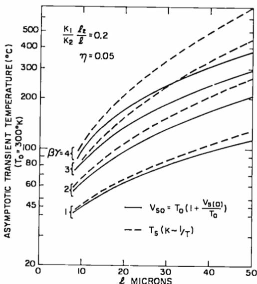
Fig. 9—Steady-state temperature rise at  $x = 0$  (maximum temperature location) for optimum  $nl = 1.5 \times 10^{12} \text{ cm}^{-2}$  in a TEO.
