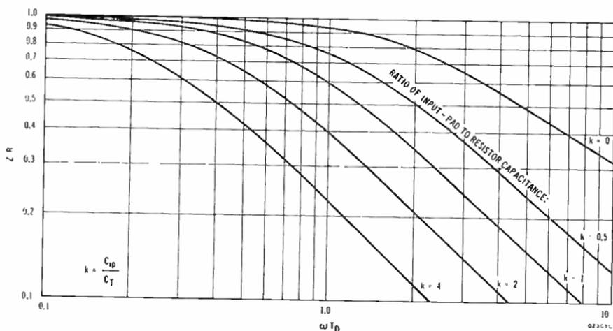
Fig. 2—Magnitude of resistor impedance as a function of normalized frequency.
