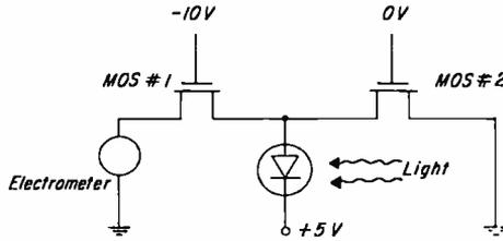
Fig. 7—Circuit diagram of a photocell under illumination.
