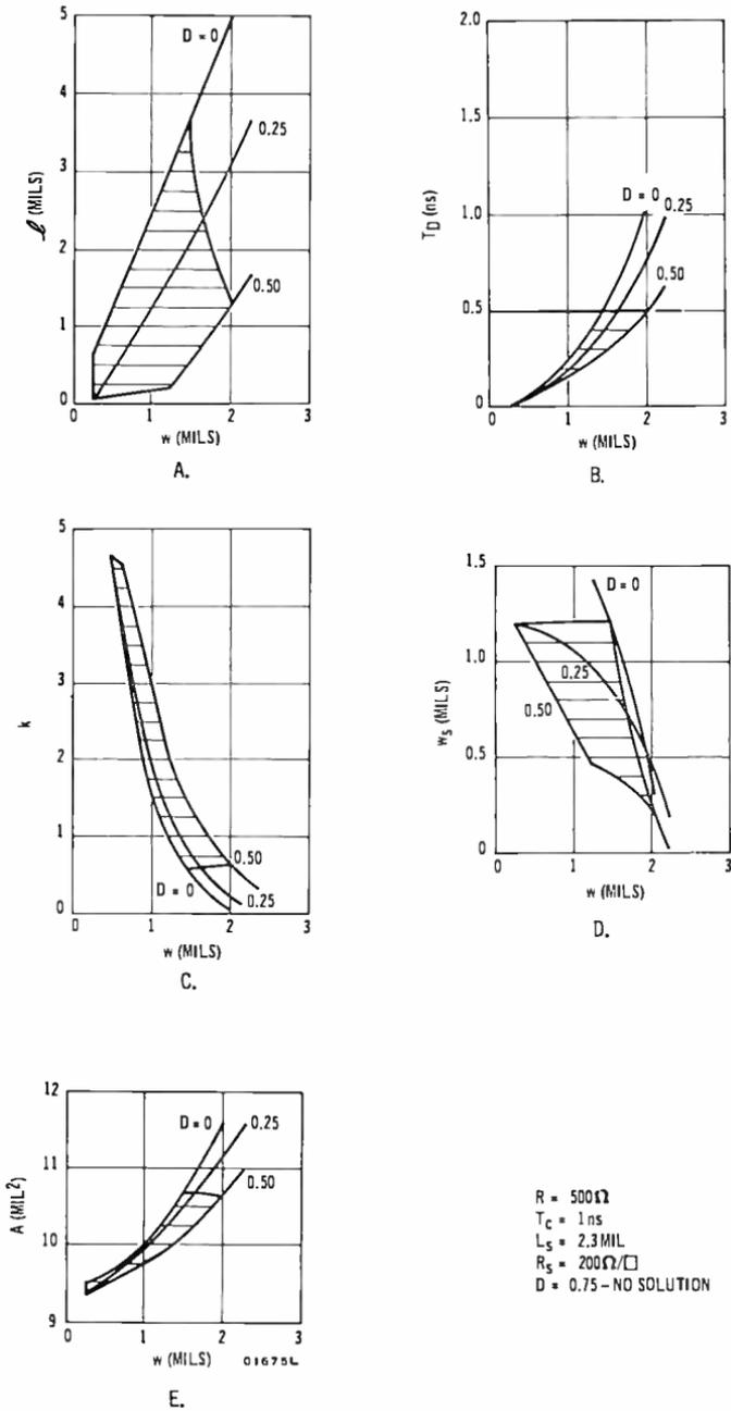
Fig. 7—Effect of varying pad-corner resolution in bar-bell resistor (shaded areas are allowed solutions).
