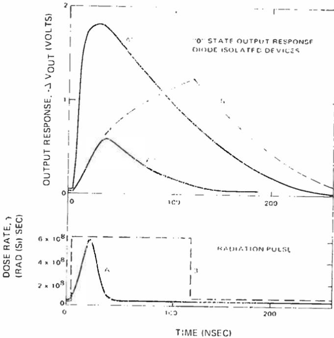
Fig. 13—Comparison of transient output responses of bipolar and CMOS integrated circuits under pulses of ionizing radiation: Curve A' is experimental data by Chang and Raymond on the response of bipolar IC when exposed to pulse of form A; curve A'' is predicted response of RCA type CD4007 gate under an identical pulse; curve B' is experimental data of the authors from which curve A'' was derived (B' was obtained using a longer radiation pulse of form B).
