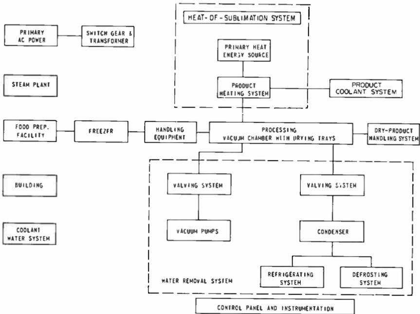
Fig. 7—Block diagram of freeze-dry processing plant.
