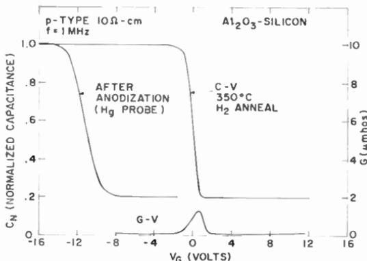
Fig. 16— $C-V$  and  $G-V$  data for a typical  $\text{Al}_2\text{O}_3$  MOS capacitor (10 ohm-cm  $p$ -type silicon).
