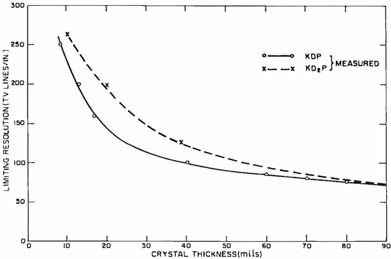
Fig. 12—Limiting resolution versus crystal thickness (measured).
