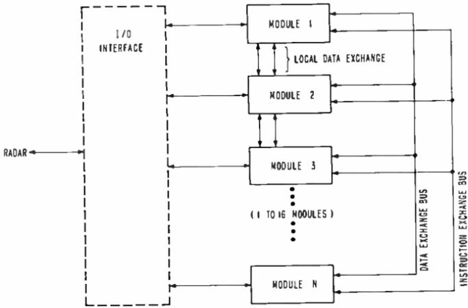
Fig. 1—Modular array computer configuration.
