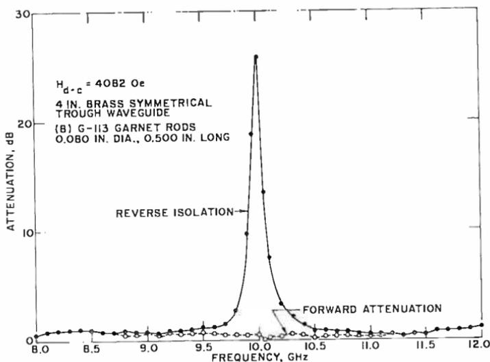
Fig. 2—Performances of a symmetrical trough waveguide ferrimagnetic resonant isolator.
