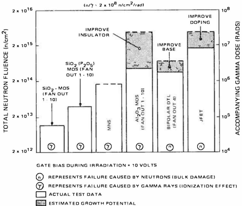
Fig. 9—Comparison of expected failure levels of various forms of digital logic due to permanent damage by neutrons and gamma rays combined.
