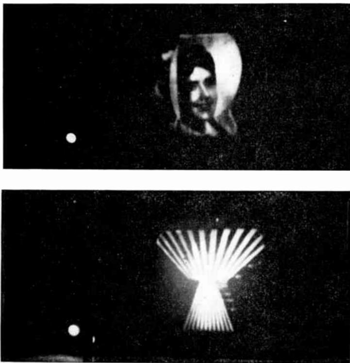
Fig. 13—Photograph indicating resolution (KDP, 8-10 mils).
