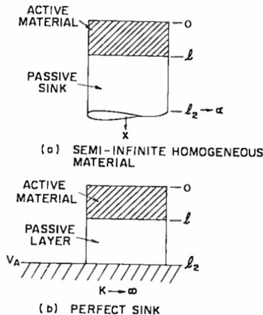
Fig. 4—Finite composite media.
