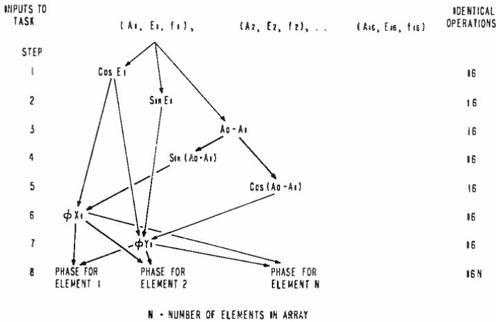
Fig. 7—Processing of phase steering commands.
