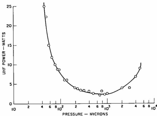
Fig. 5—Typical variation of glow power as a function of pressure for a beef patty 0.5-inch thick at a frequency of 915 MHz.<sup>1</sup>
