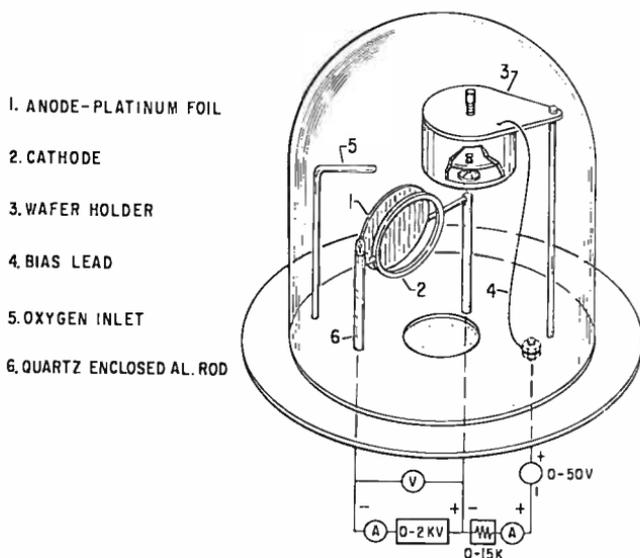
Fig. 15—Method of fabricating  $Al_2O_3$  films by plasma anodization.
