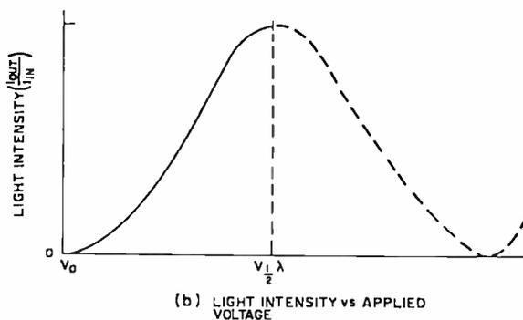
Fig. 1—(Top) Fundamental operation and (bottom) relative light intensity versus applied voltage.
