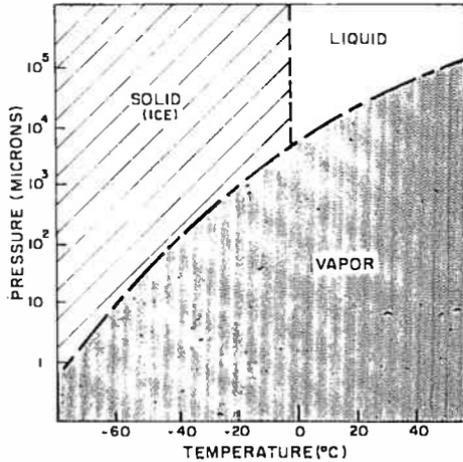
Fig. 1—Phase diagram for water at low pressures.
