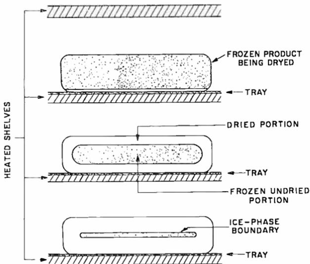
Fig. 3—Regression of ice-phase boundary during freeze drying.
