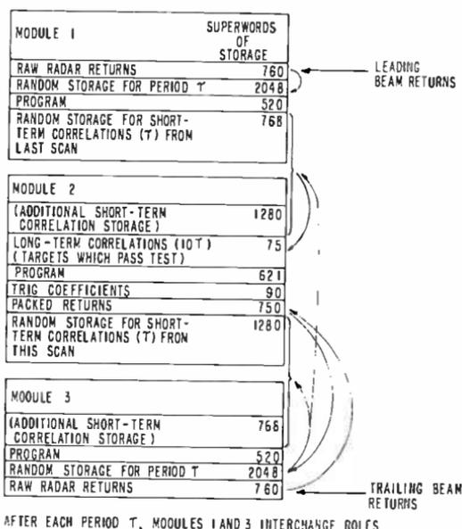
Fig. 10—Parallel processing of scintillation test.
