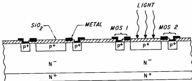
Fig. 3—Cross-section of the MOS-P+N-N+ photosensor array.
