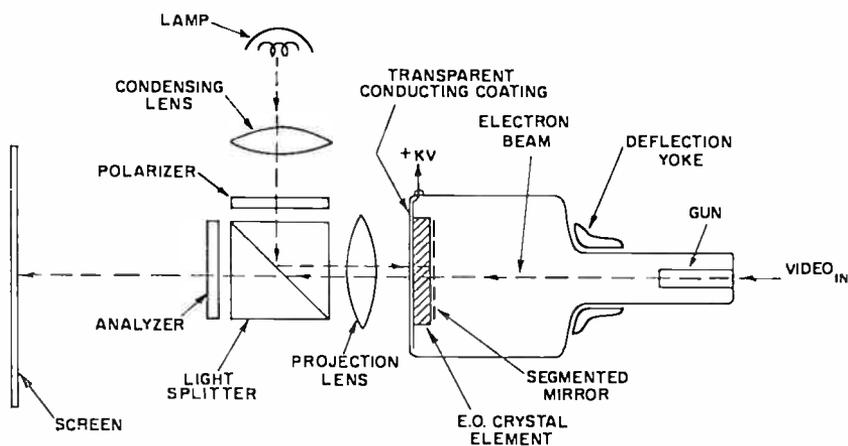
Fig. 3—Reflex on-axis system.
