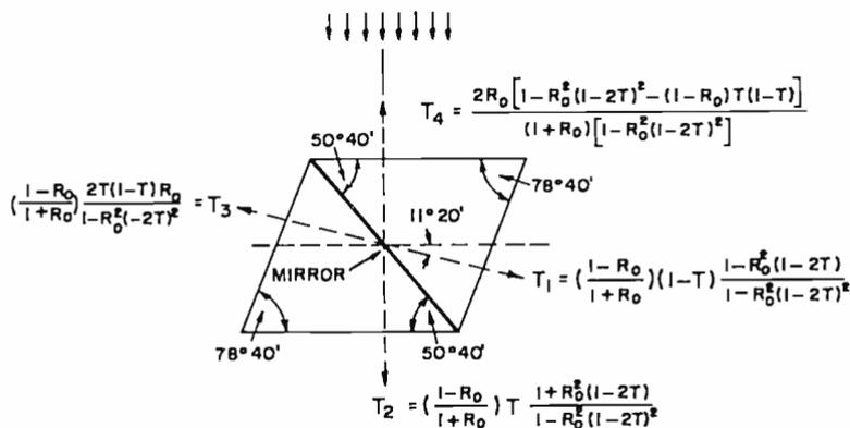
Fig. 5—Dichroic-mirror-prism configuration.
