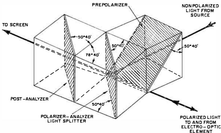
Fig. 6—Dichroic-mirror-prism optical system.
