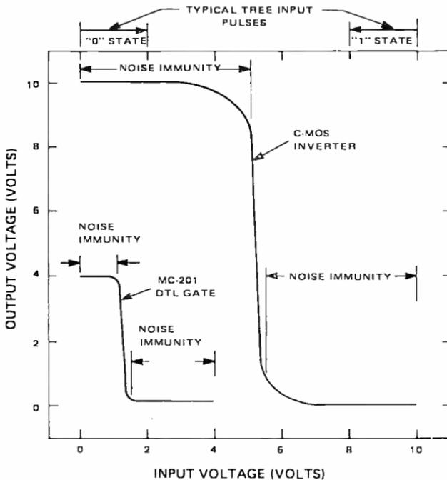
Fig. 10—Comparison of noise immunity of a CMOS inverter and bipolar-transistor DTL inverter.
