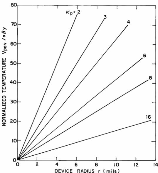
Fig. 6—Average temperature rise due to spreading resistance, with the post thermal conductivity as a parameter.
