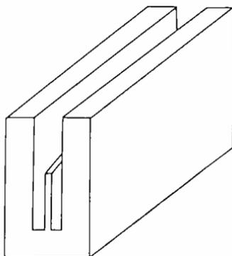
Fig. 1—Symmetrical trough waveguide.
