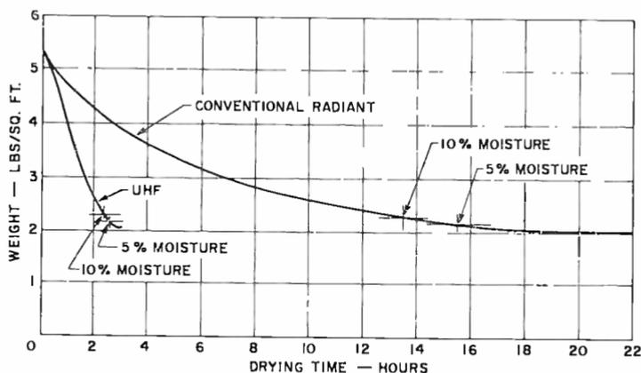
Fig. 4—Comparison of drying curves for UHF and radiant freeze drying of chopped beef 1-inch thick to moisture levels of 0, 5, and 10%.<sup>1</sup>
