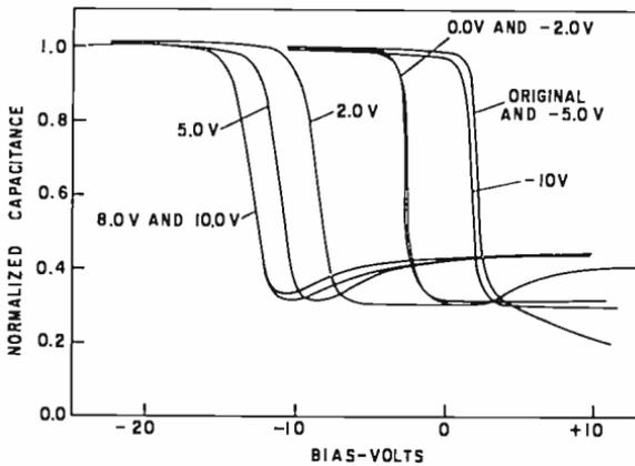
Fig. 20—Effect of 1 MeV bombardment on Al<sub>2</sub>O<sub>3</sub> MOS capacitor formed by vapor deposition.
