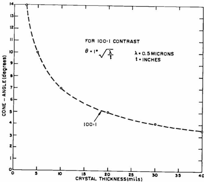
Fig. 15—Crystal thickness versus cone angle for 100:1 contrast.
