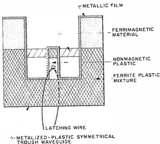
Fig. 4—A latching metalized-plastic symmetrical trough waveguide ferrimagnetic differential phase shifter.
