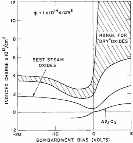
Fig. 19—Relative behavior of  $\text{Al}_2\text{O}_3$  devices under bombardment bias.
