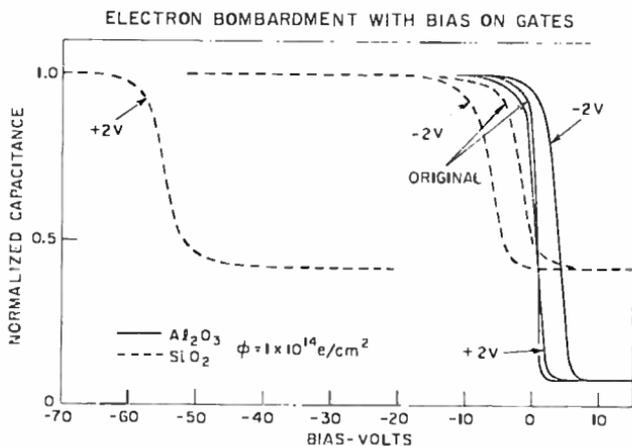
Fig. 18—Effect of 1 MeV bombardment with different gate biases.
