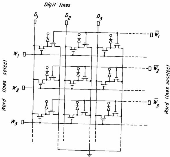
Fig. 2—Circuit configuration of photosensor array. The common cathode of all photodiodes is biased positively.
