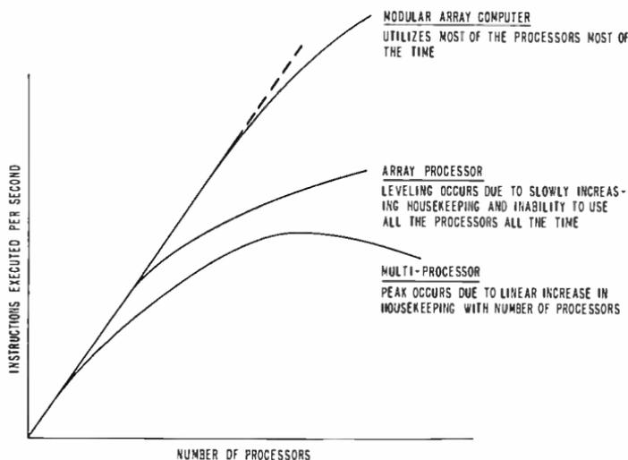
Fig. 3—Relative performance of computer configurations.
