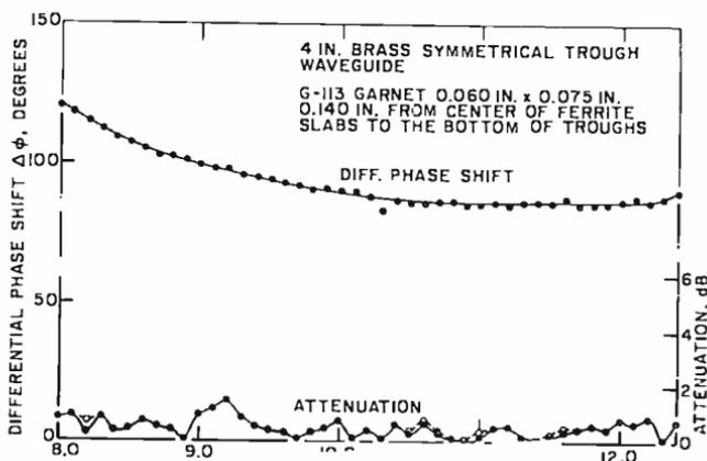
Fig. 3—Performances of a symmetrical trough waveguide ferrimagnetic differential phase shifter.
