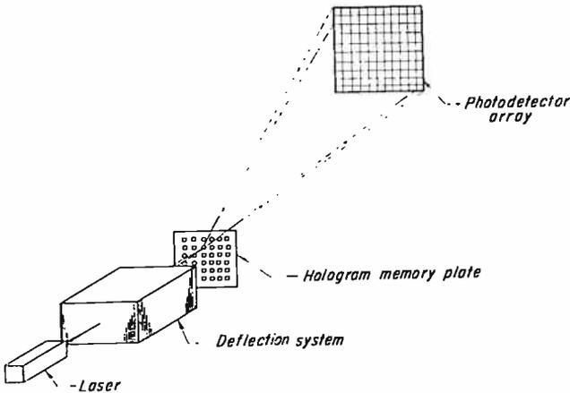
Fig. 1—Typical structure of a holographic read-only optical memory.
