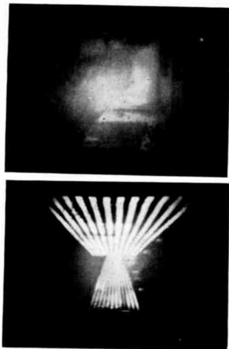
Fig. 18—Photograph indicating poor crystal uniformity (top: test pattern; bottom: blank radar scan).
