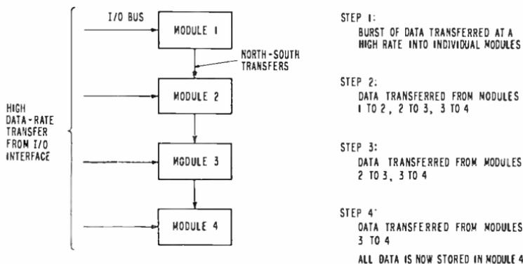
Fig. 5—Loading of burst of radar data into one module.
