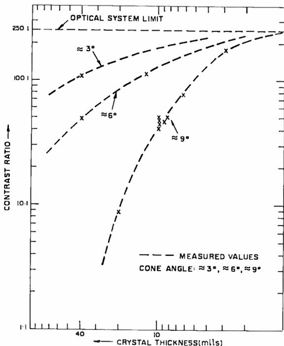
Fig. 8—Contrast ratio versus crystal thickness.
