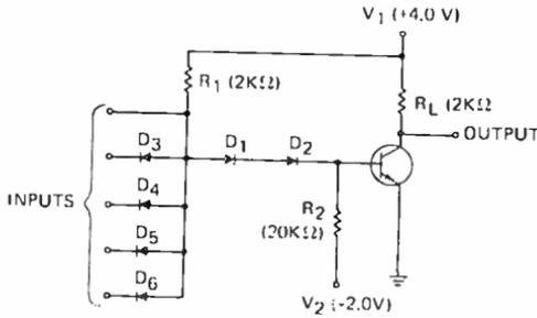
Fig. 3—Bipolar transistor integrated circuit (DTL 4-input NAND gate).
