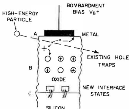
Fig. 6—Charge-trapping mechanism in MOS transistors.
