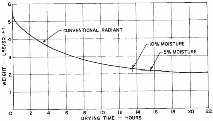
Fig. 2—Typical freeze-drying processing schedule using radiant heat (chopped beef, 1-inch thick).<sup>1</sup>
