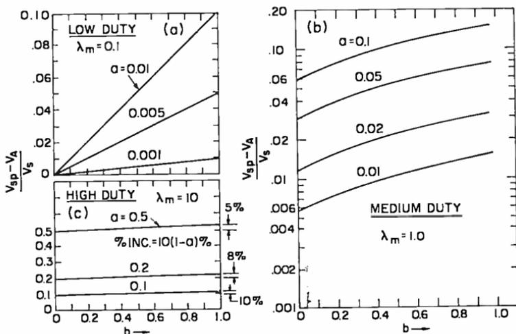
Fig. 10—Temperature rise during pulse for steady periodic heating.
