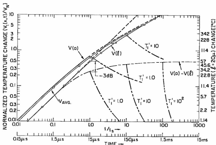
Fig. 5—Transient temperature response of  $n$ -layer terminated in infinite  $n^+$  material due to unit pulse.
