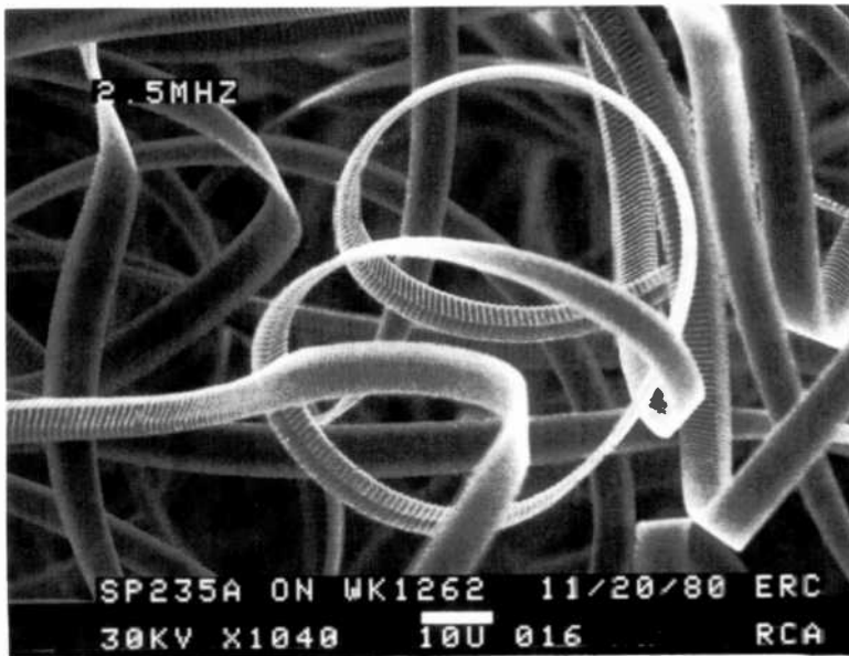
Fig. 10—Scanning electron micrograph of copper chip produced during mastering of 5 MHz signal (calibration mark shows 10 \mu m).
