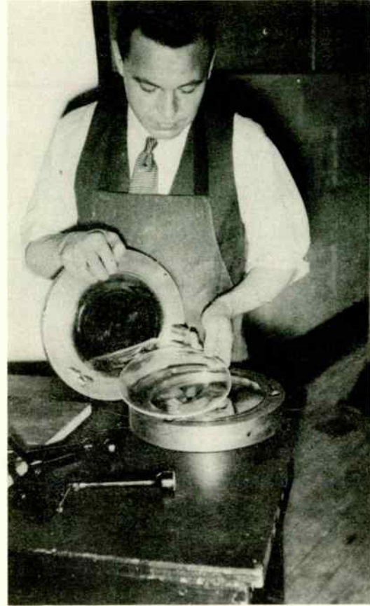
I. G. MALOFF REMOVING PLASTIC LENS FROM MOLD
