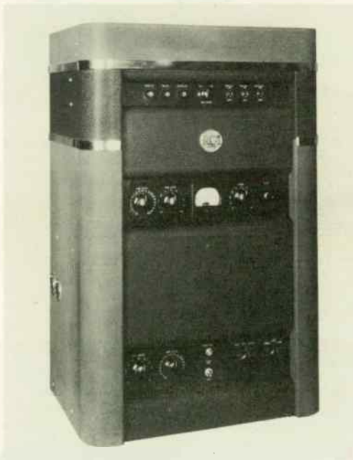
AMPLIFIER CABINET FOR RECORDING EQUIPMENT
