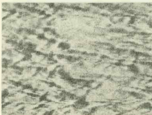
SCANNING MICROSCOPE PICTURE OF POLISHED, COLD-ROLLED STEEL SURFACE, SLIGHTLY ETCHED WITH NITOL
