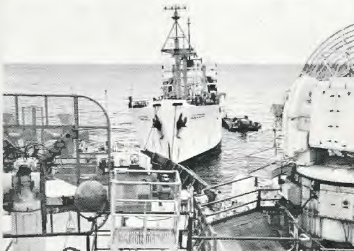
Water is transferred from the Mariner to the Atlantic Missile Range Instrumentation Vessel Timber Hitch.
