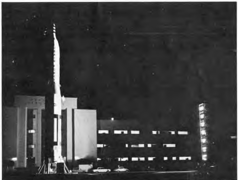
TO LIGHT A NIGHT LAUNCH, MTP's Range Photography unit has successfully tested the use of quartz-iodine sealed-beam lamps; found them effective, and cheaper.
