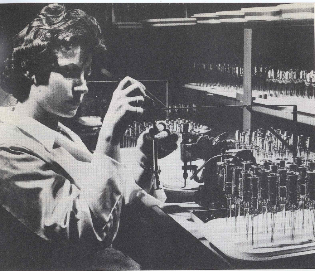
At RCA's modern Silverama plant in Marion, Ind., there's never a compromise with quality. Consider the assembly of electron guns, for instance. Since a tiny speck of dust in the wrong place can limit top performance of a picture tube, RCA assembles its electron guns in a dust-free, super-clean "White Room," as illustrated above and below.
