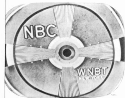
Figure 22—Horizontal Drive Control Misadjusted
