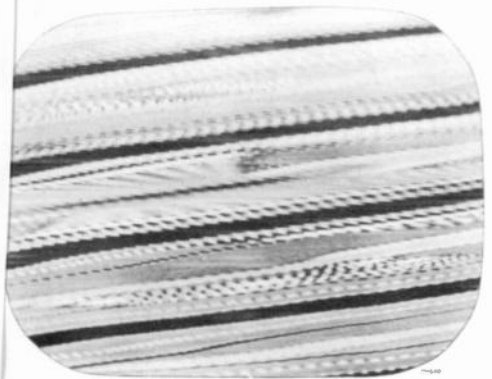
Figure 24—Test Pattern Showing Out of Sync Condition When Horizontal Hold Control Is in a Counter-clockwise Position—Just Before Pulling Into Sync
