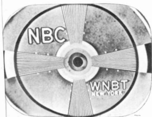
Figure 20—Horizontal Linearity Control Misadjusted (Picture Cramped in Middle)
