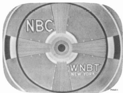
Figure 21—Focus Magnet and Ion Trap Magnet Misadjusted
