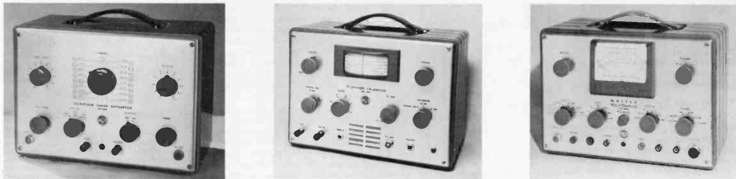
Fig. 2. (Left) Instant channel selection is a feature of this television sweep generator. (Center) Television calibrator for the precision alignment of wideband amplifiers. (Right) The vacuum tube voltmeter is practically a universal test instrument applicable to all types of radio and electronic servicing.
