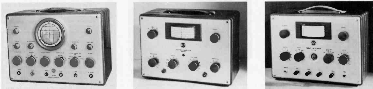
Fig. 3. (Left) The oscilloscope is a useful tool in visual alignment procedures and for observing waveforms. (Center) The r.f. test oscillator is a basic AM servicing instrument. (Right) The audio oscillator is valuable in the service shop and may be used to locate performance difficulties in video amplifiers.
