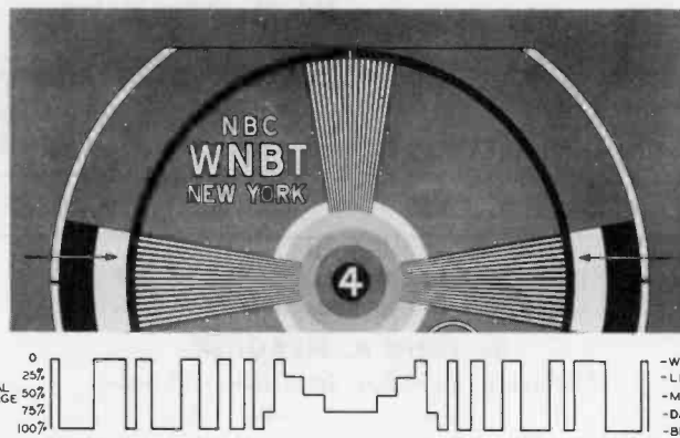
FIGURE 4—WAVEFORM OF SIGNAL VOLTAGE ALONG ONE LINE OF WNBT TEST PATTERN.
