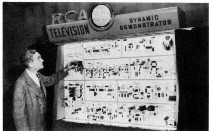
A complete, operating 30-tube television receiver "a-la-bread board" is put through its paces by the designer, John Meagher, Television Specialist of the RCA Tube Department. Mr. Meagher's "Television Service" series is currently running in RCA RADIO SERVICE NEWS.
