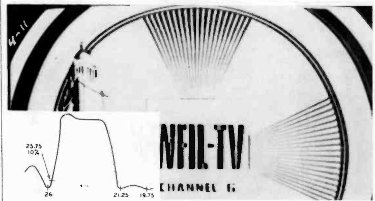
Fig. 9—Poor low-frequency response, evidenced by weak horizontal wedge. This was caused by tuning adjacent-channel sound trap close to picture carrier. Similar to Fig. 1.
