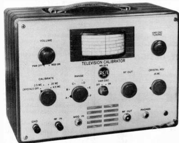
Fig. 2. The television calibrator comprises a high-quality vfo signal generator, dual crystal frequency standards, and a heterodyne frequency meter.
