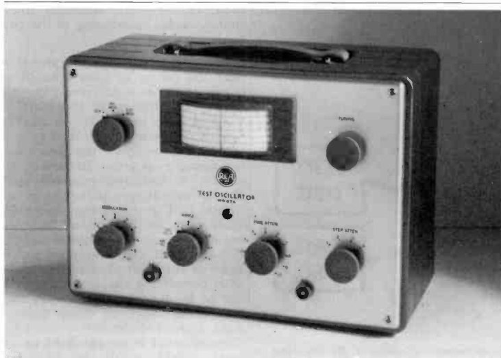
Fig. 3. Although primarily an AM service instrument, this reliable test oscillator may be used in combination with other instruments, as a marker generator in aligning TV sets.
