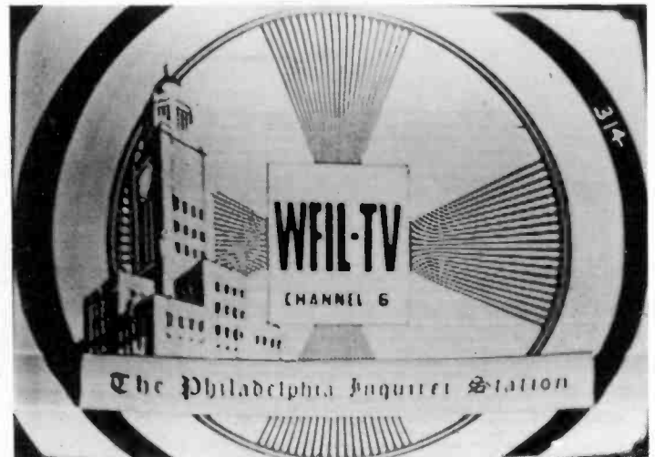
Fig. 10—This photograph was made with a camera shutter speed of 1/100 second to show how the horizontal wedge of a test pattern appears when formed by only one field: Every other horizontal scanning line is missing. The effect resembles, but is not the same as, an out-of-interlace condition.
