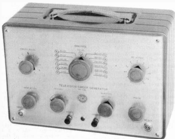
Fig. 1. This modern sweep-frequency generator delivers an output which is flat within \pm 1.5 db, and provides a maximum attenuation ratio of 20000/1.
