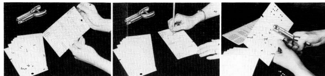
In preparing a punched card: first, line up index slots and bottoms of Master Card and blank card. Clip the two cards together. Next, as shown center, use a sharp-pointed pencil to inscribe hole outlines on blank card. Then, center each penciled-hole outline exactly in die on top of punch before punching hole.
