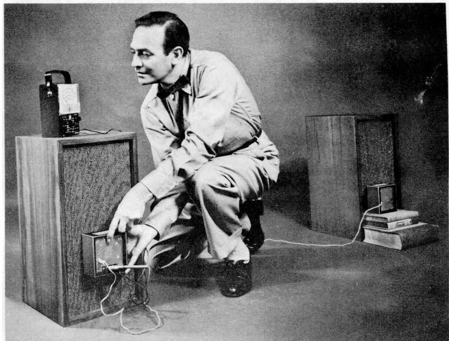
Here, a service technician uses RCA's two-unit WG-360A to check phasing between the left-hand and right-hand speaker assemblies in a stereo system.
