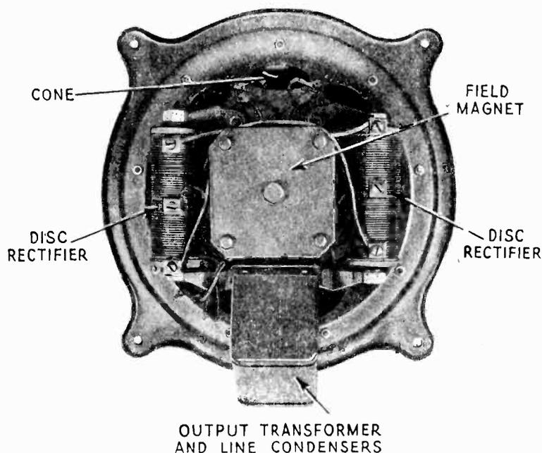
*Figure 21—Reproducer assembly showing parts*
