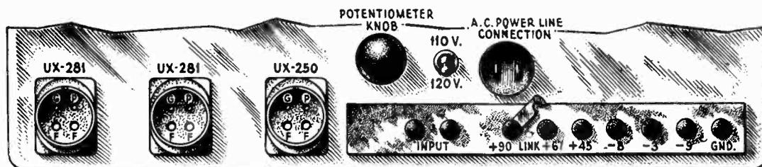
Figure 9—Location of Radiotron socket contacts and socket power unit binding posts.
