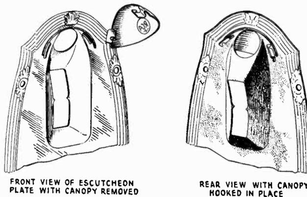
Figure 7—Method of fitting canopy into escutcheon plate.
