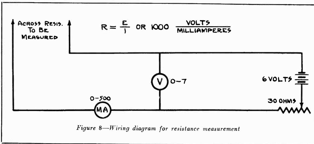
Figure 8—Wiring diagram for resistance measurement
