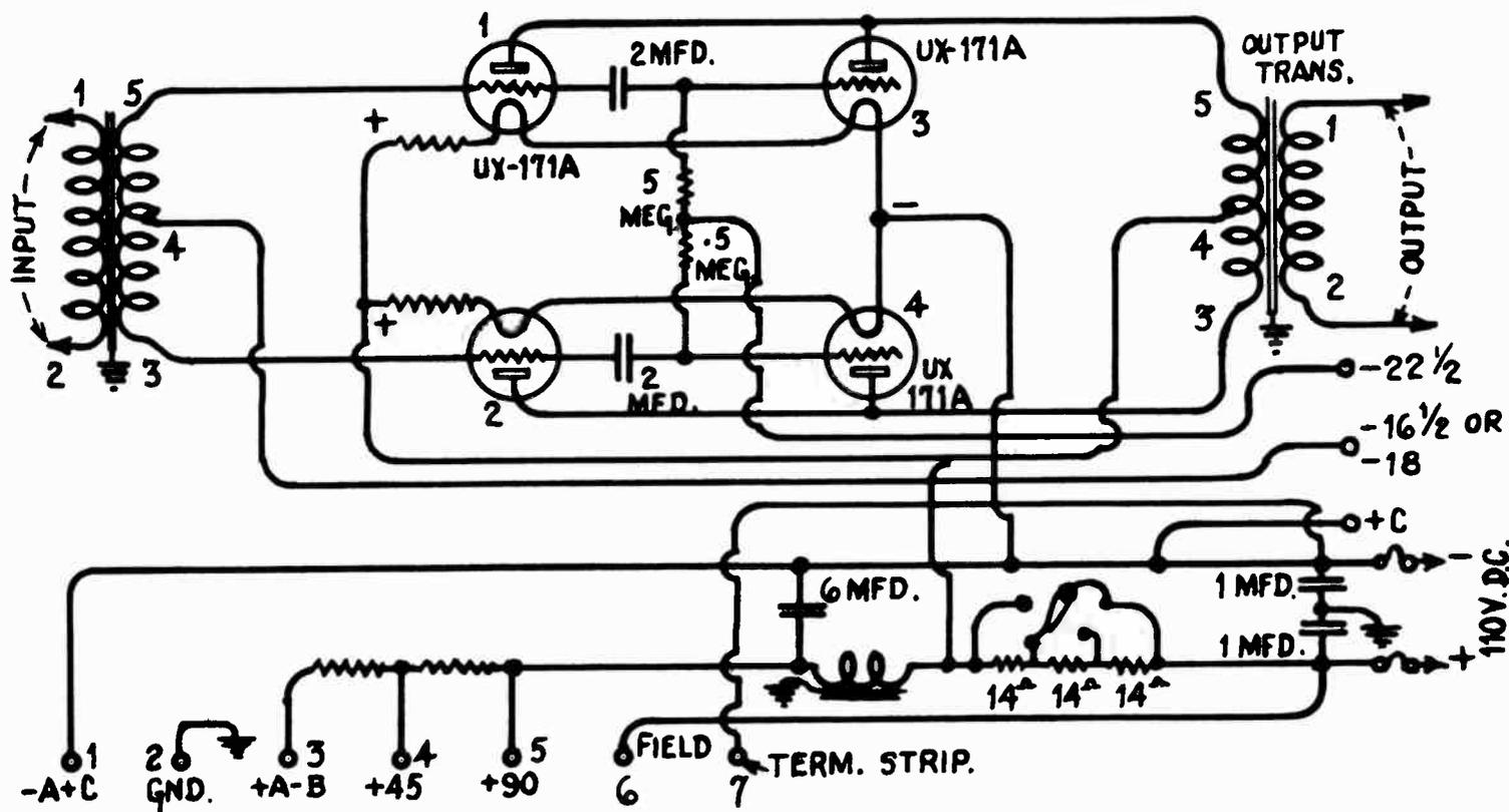
Figure 3 -- Radiola 32 D.C. socket power unit schematic circuit with terminal connections and voltages.
