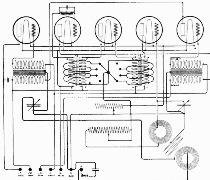
FIG. 6 - SCHEMATIC WIRING DIAGRAM OF RADIOLA IX
