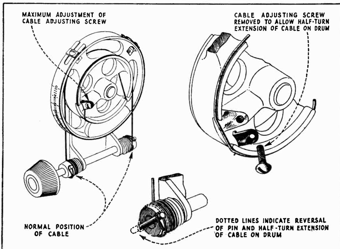
Figure 4—Three-gang condenser cable and drum operating mechanism
