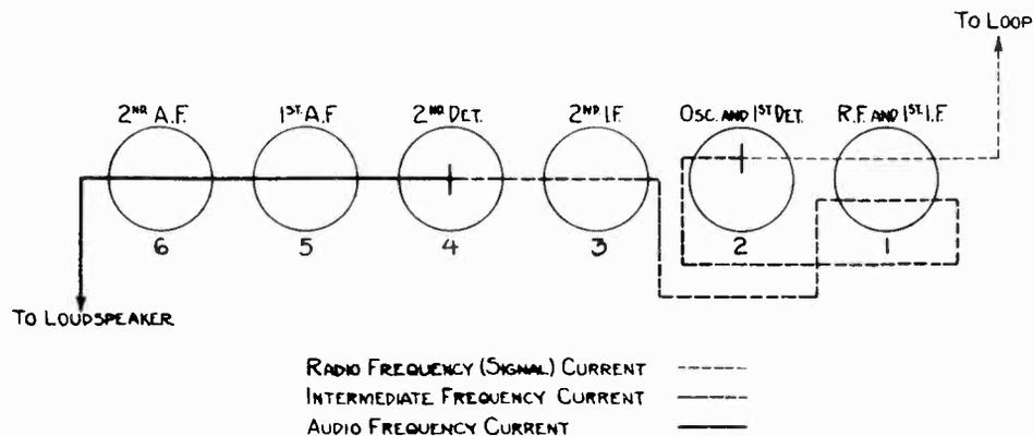
Figure 1—Radiotron Sequence
