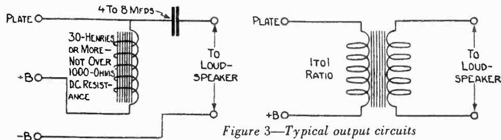
Figure 3—Typical output circuits
