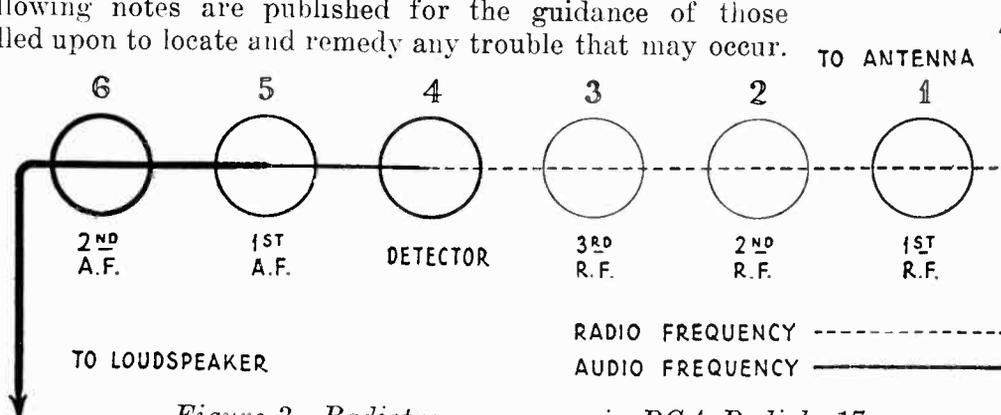
Figure 3—Radiotron sequence in RCA Radiola 17
