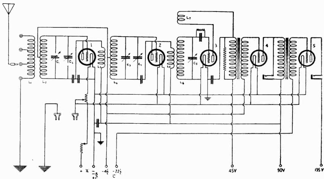
Figure 1—Schematic circuit of RCA Radiola 20
