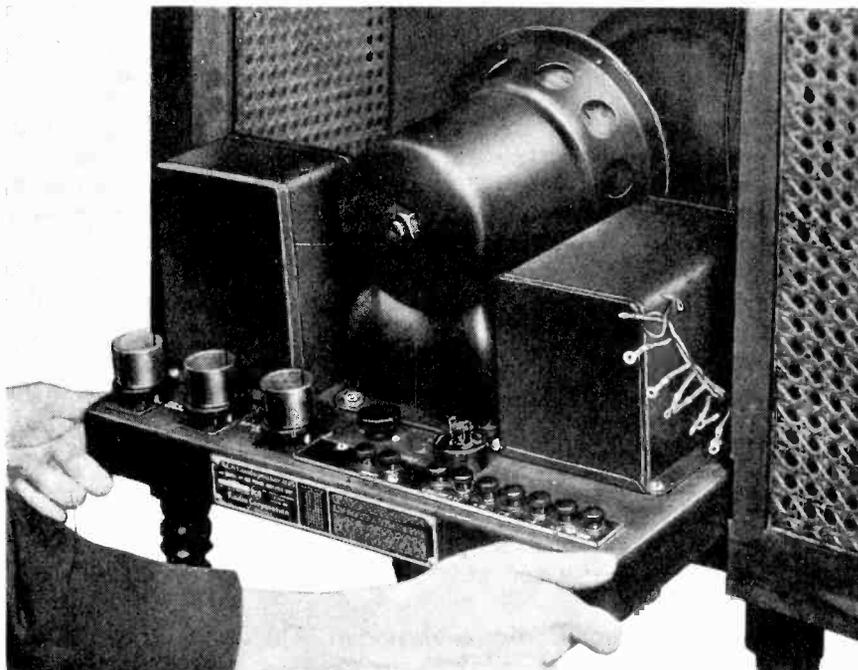
*Figure 10—Removing chassis assembly from cabinet.*
