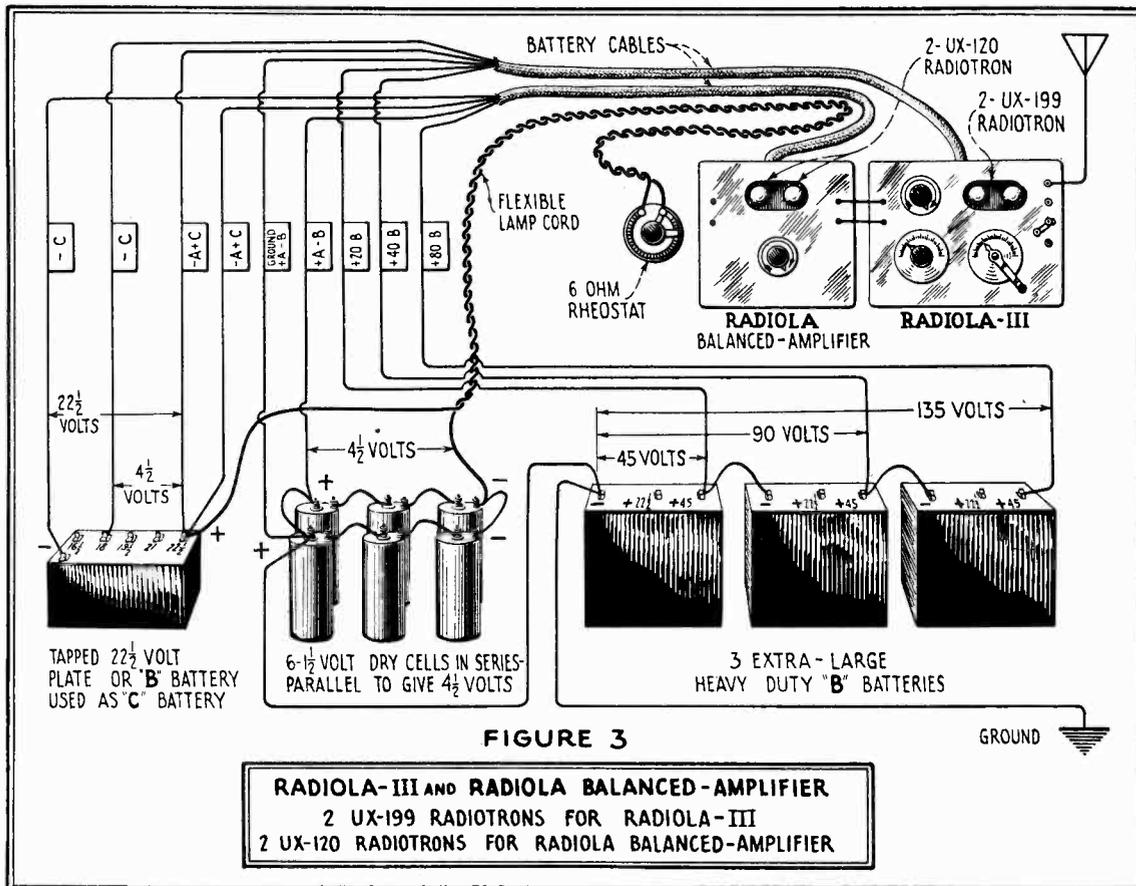
A six ohm external rheostat is connected in the battery circuit according to the diagram in Figure 3. The following apparatus will be required:
