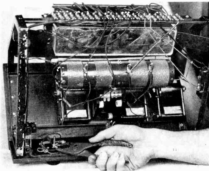
*Figure 4—Adjusting contact arm on rheostat*
