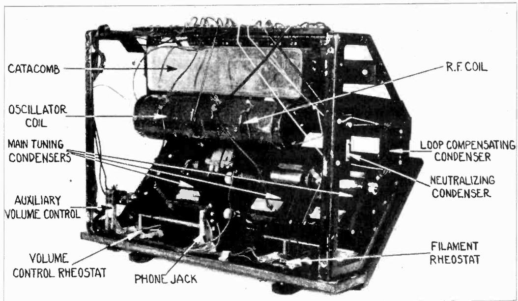
Figure 2—Rear view of panel assembly
