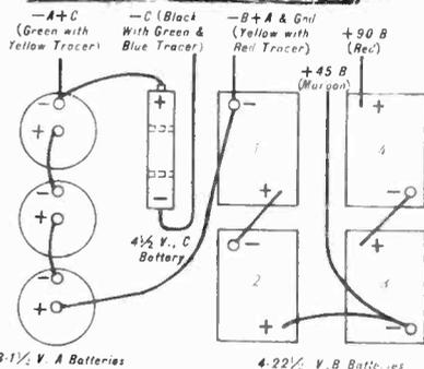
Diagram of Battery Connections for Portable Unit
