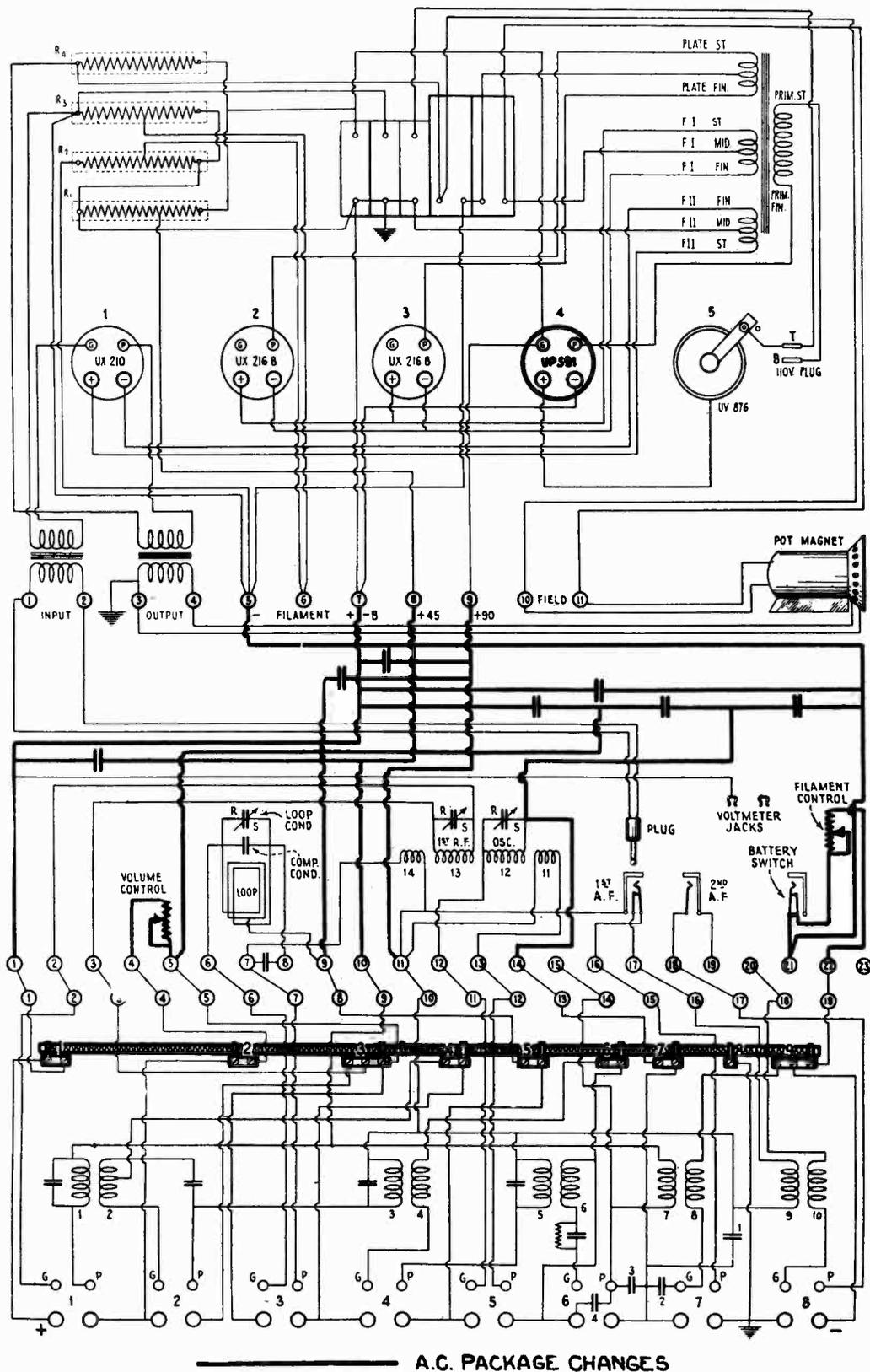
Figure 4—Radiola 28 A.C. operated continuity circuit diagram
