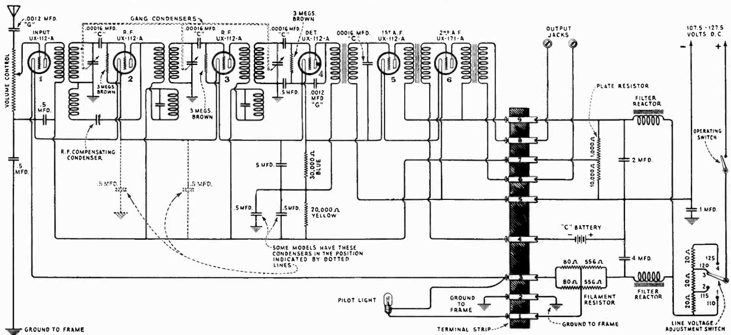
Figure 4—Schematic circuit diagram of Radiola 18 D.C.
