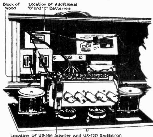
Location of UR-556 Adapter and UX-120 Radiotron
