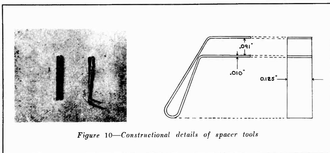
armature correctly it will be first necessary to make a set of spacer tools (Figure 10). These are made of  $\frac{1}{8}$ " stock phosphor bronze .010" thick and bent to give two surfaces .091" apart. Two of these tools are necessary. After the two screws are loosened at each end of the armature these tools are inserted at each end between the armature and pole pieces (Figure 11). The screws are then tightened with the spacer tools in place. This completes the adjustment.
