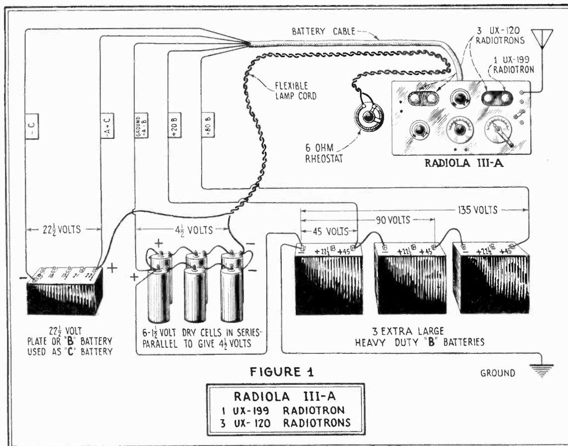
"A" battery decreases thru use, it will be necessary to advance the setting of the external Rheostat to maintain normal filament terminal voltage. "A" battery renewal is not required until it becomes necessary to advance the external Rheostat to its maximum current position to obtain normal results.
