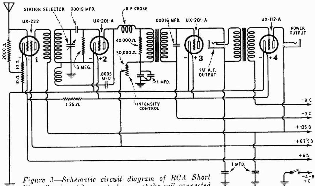
Figure 3—Schematic circuit diagram of RCA Short Wave Receiver (Some sets have a choke coil connected in the antenna circuit instead of the 2000-ohm resistor shown)
