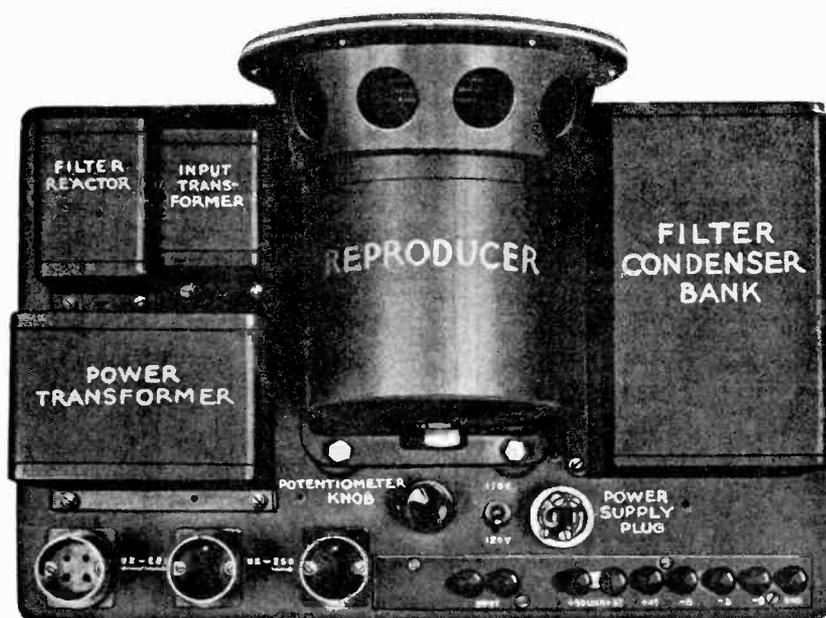
Figure 2—Top view of chassis assembly.
