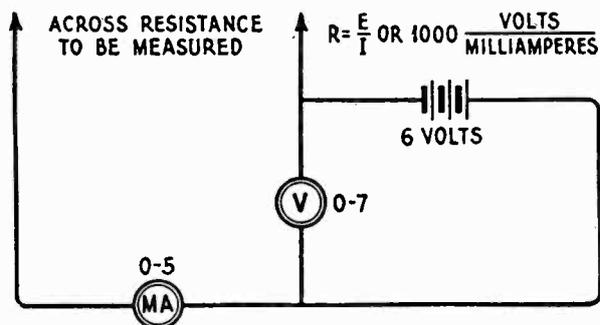
Figure 8—Schematic circuit for resistance measurement.
