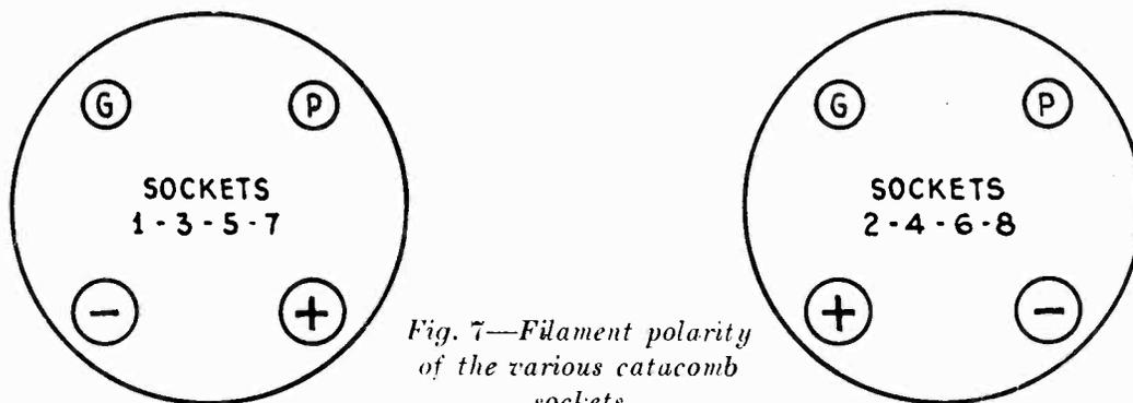
*Fig. 7—Filament polarity of the various catacomb sockets*
