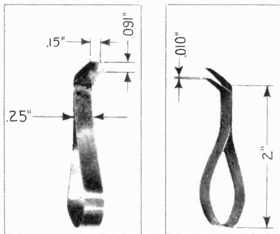
Figure 12—General appearance and correct dimensions of armature spacing tools
