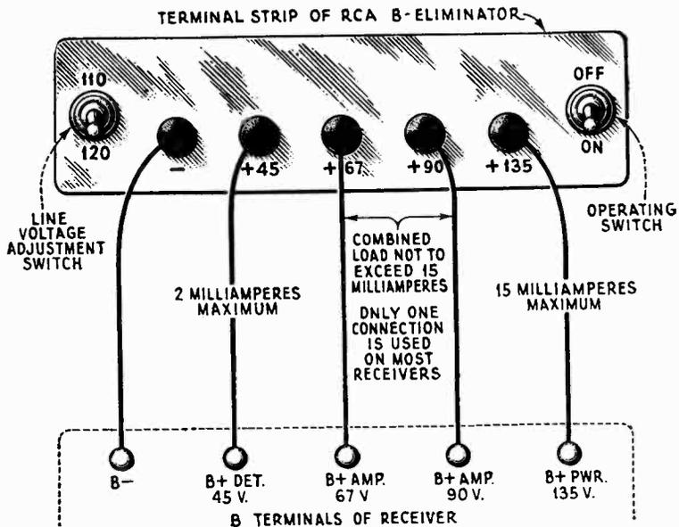
Figure 2—Connections from RCA B-Eliminator to a receiver
