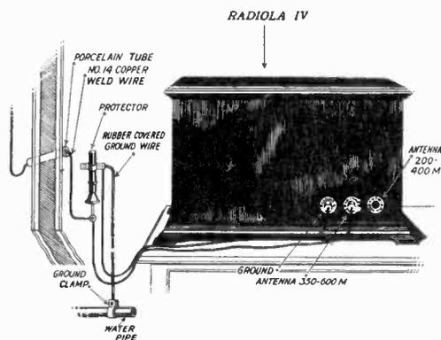
Fig. 2. Installation of Radiola IV
