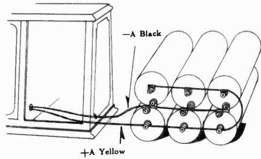
Fig. 3—Showing Method of Connecting A Batteries
