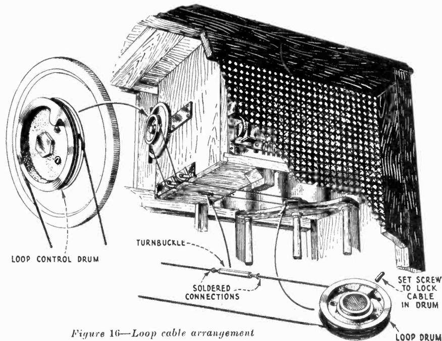
Figure 16—Loop cable arrangement
