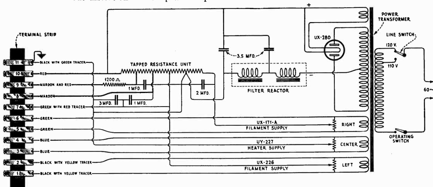
Figure 4A—Schematic circuit diagram of socket power unit.
