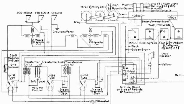
Fig. 5. Schematic Wiring Diagram of Radiola IV
