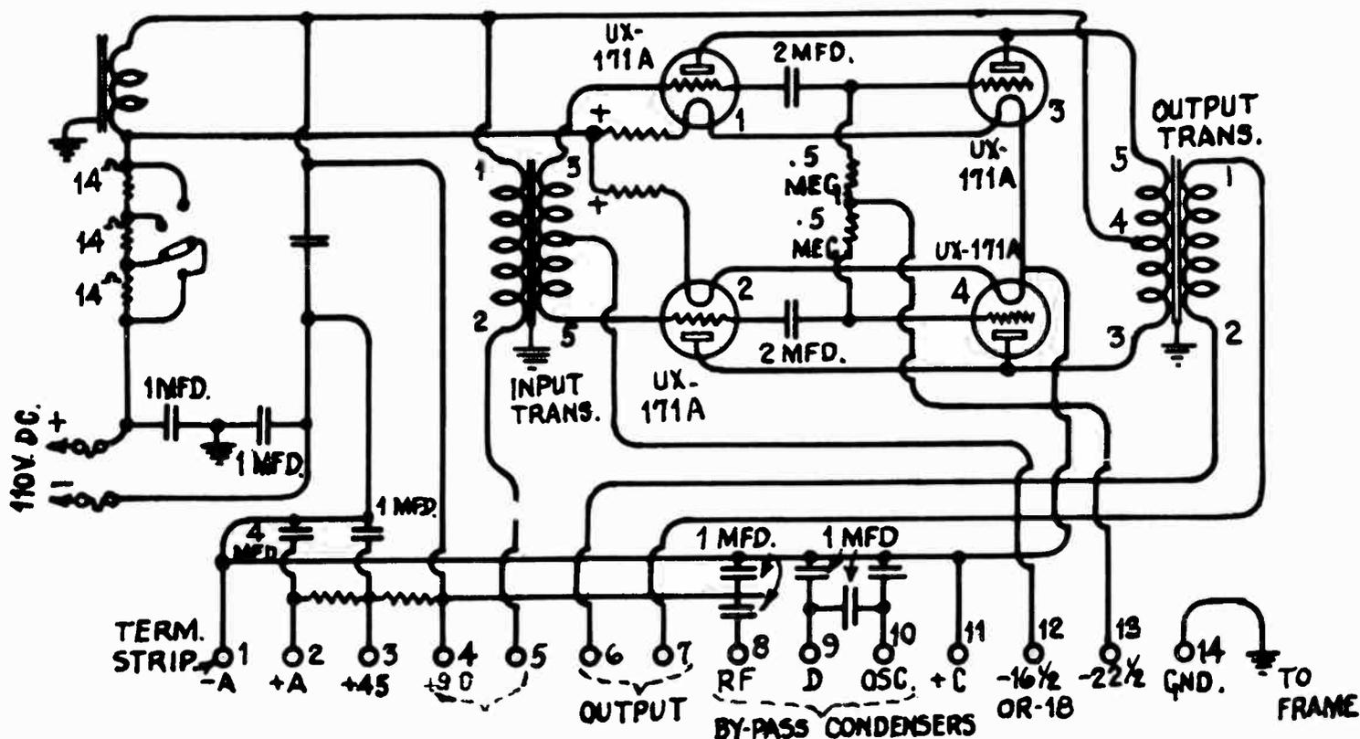
Figure 2 -- Radiola 30A D.C. Socket Power Unit schematic circuit with terminal connections, plate, grid and filament voltages.
