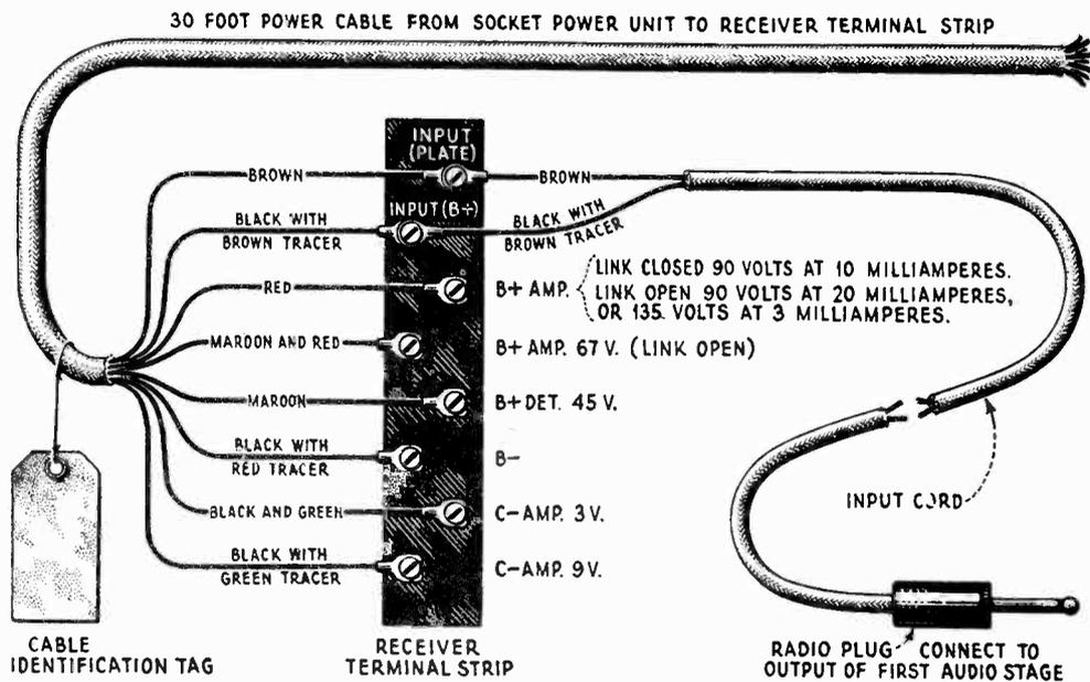
Figure 5—Thirty-foot power cable and receiver terminal strip.
