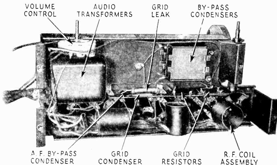
Figure 2—Sub-chassis view of receiver assembly showing parts
