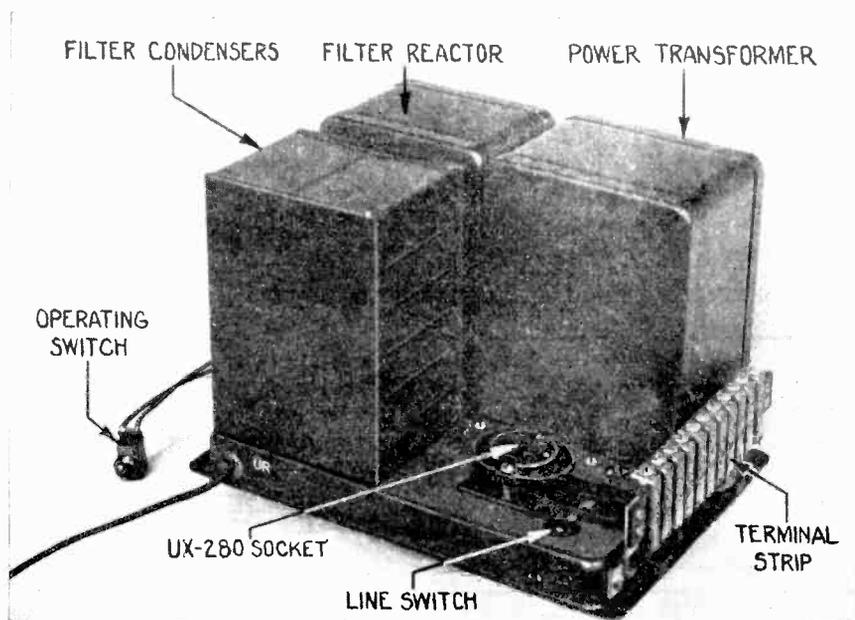
Figure 2—Socket Power Unit showing various parts.
