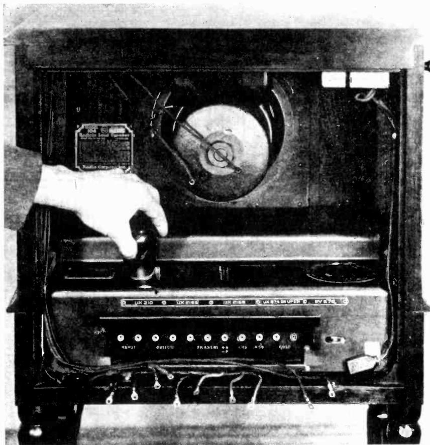
*Figure 6—Removal of R.P.A. connections, Radiotrons and Rectrons preparatory running continuity tests*
