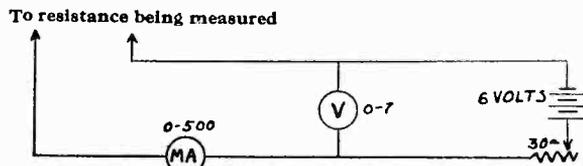
Fig. 4—Wiring Diagram for Resistance Measurement
