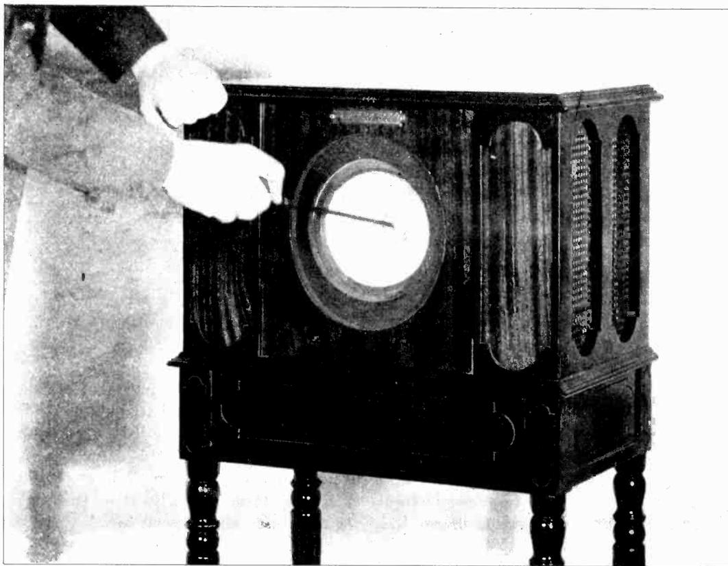
*Figure 4—Readjusting cone*
