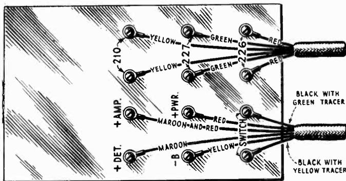
Figure 13—Sterling S. P. U. terminal board showing color scheme of connections
