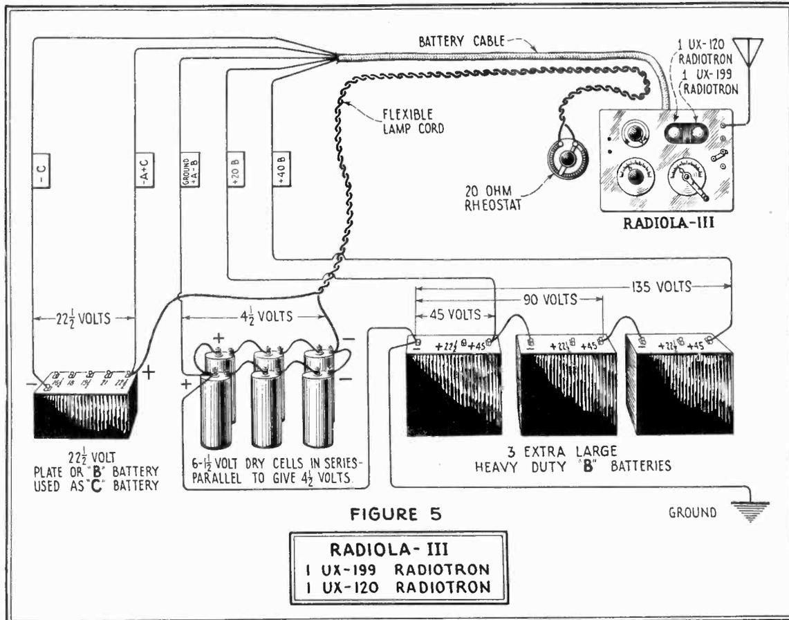
Before connections are made the *external* Rheostat should be turned to its "OFF" position (so that movable arm does not touch resistance winding). All connections should then be checked against Figure 5.
