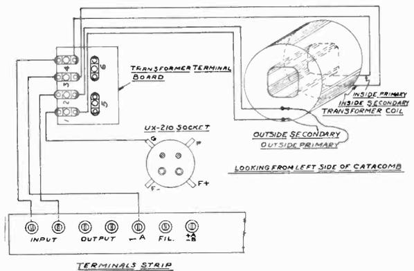
9-40 Input Transformer Wiring
