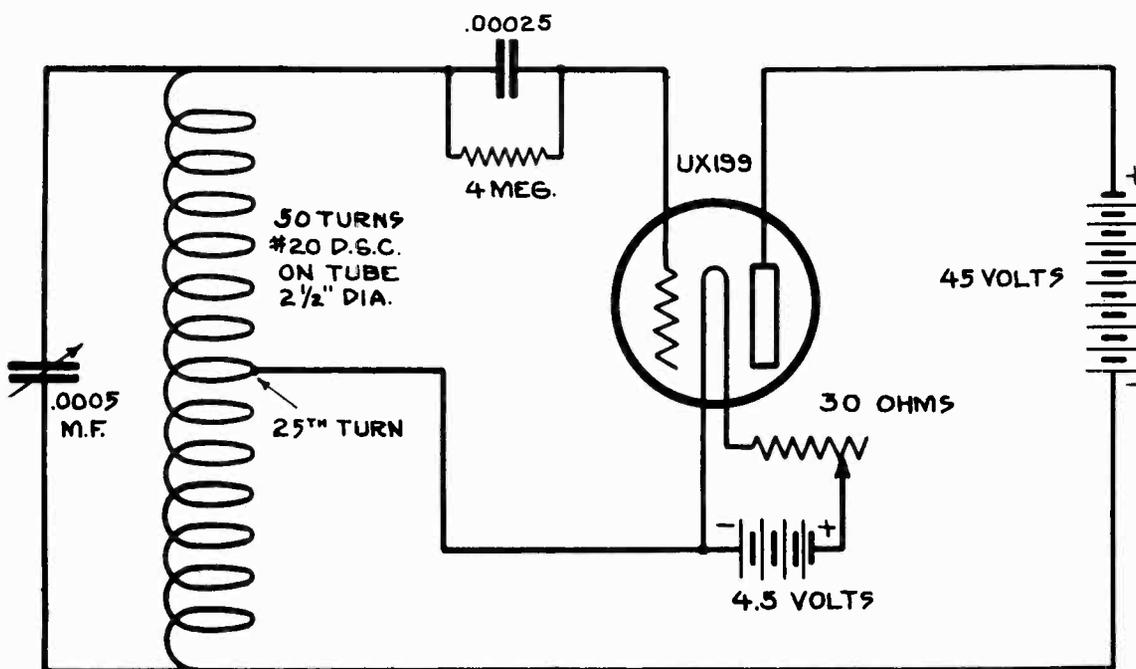
Figure 4—Wiring diagram of the modulated oscillator
