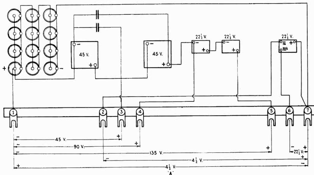
Figure 6—Correct voltage readings across battery terminal strip
