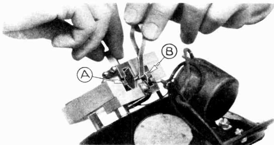
*Figure 5—Armature bracket adjusting screws A and B*
