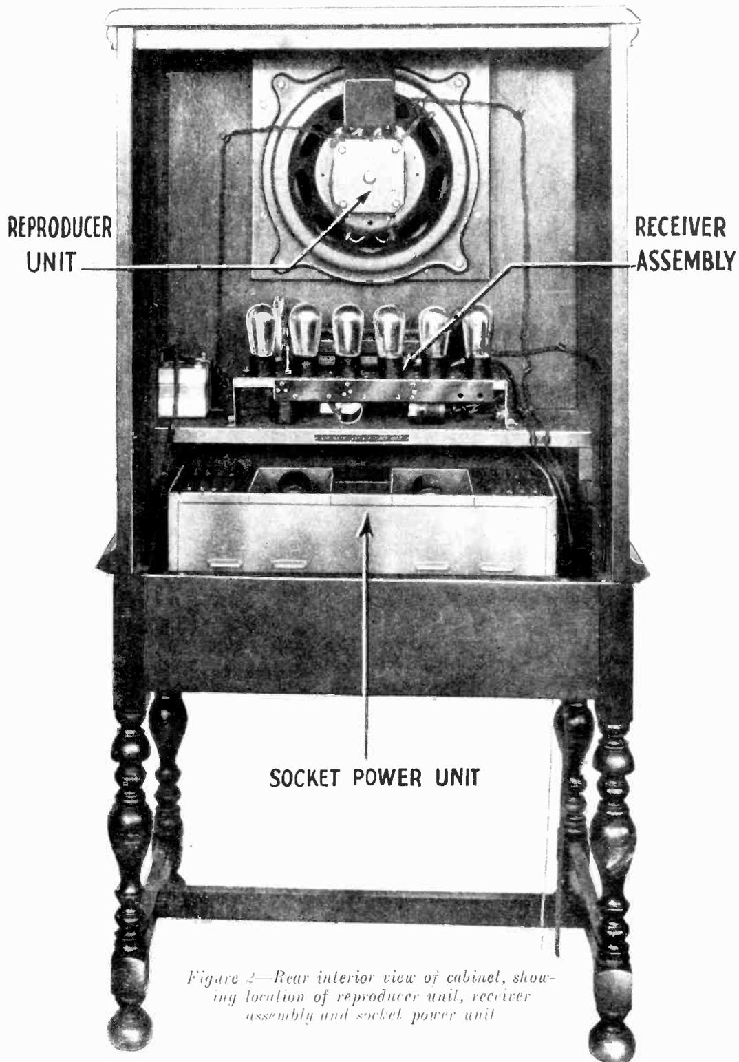
*Figure 2—Rear interior view of cabinet, showing location of reproducer unit, receiver assembly and socket power unit*
