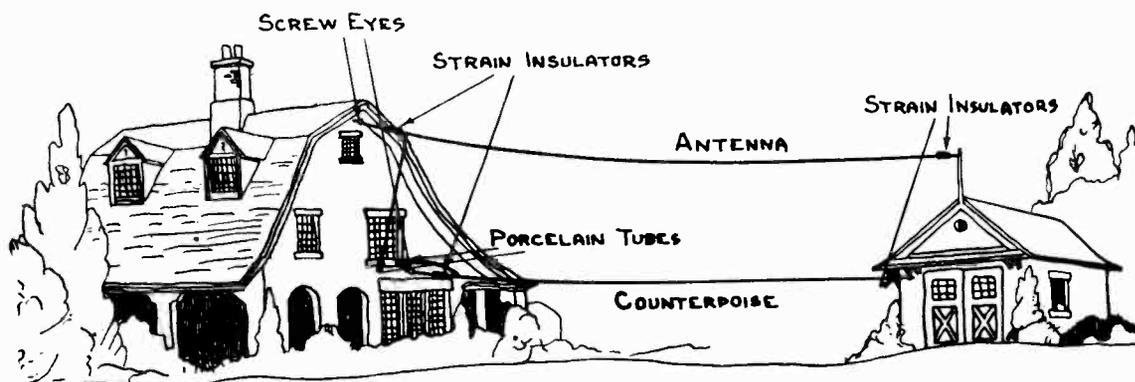
Figure 3—Typical Outdoor Antenna Installation
