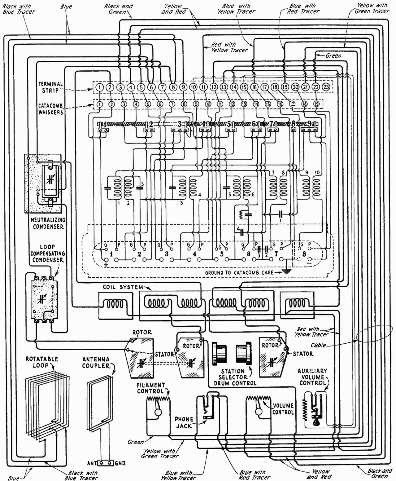
Figure 9—Panel and loop assembly continuity wiring diagram
