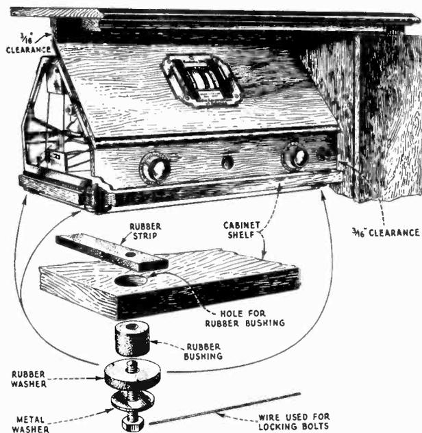
Figure 8—Panel assembly supports with rubber insulation to prevent microphonic action
