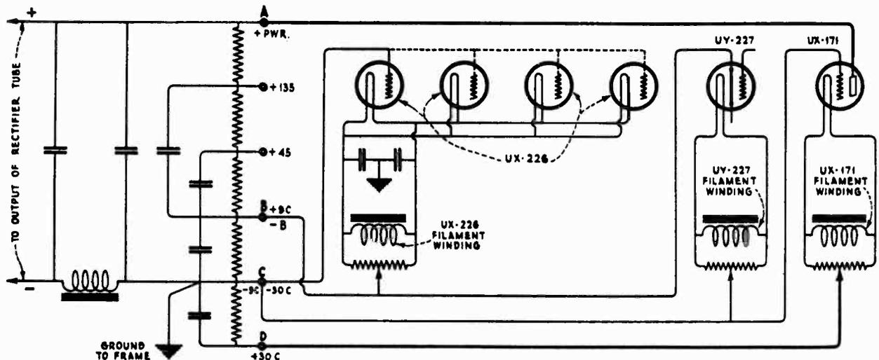
Figure 18—Schematic circuit for securing grid biasing voltages.
