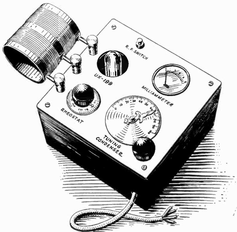
Figure 5—Complete model of R.F. and A.F. oscillator
