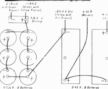
Diagram of Battery Connections When Using Home Battery Box
