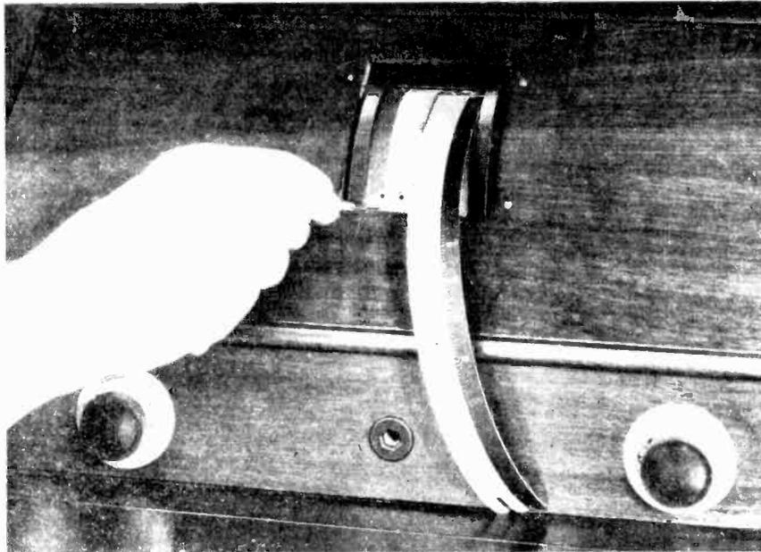
*Figure 15—The correct method of replacing dial scales*
