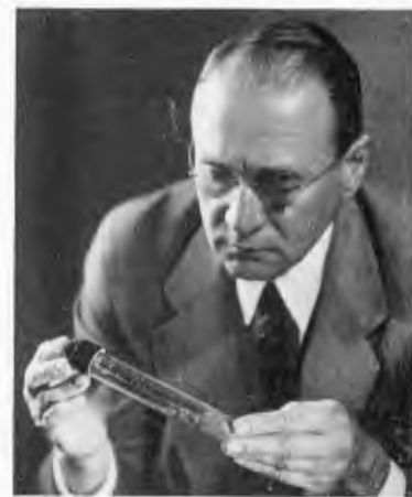
Dr. V. K. Zworykin examining the new electron multiplier tube which has wide application in all types of amplification circuits.
