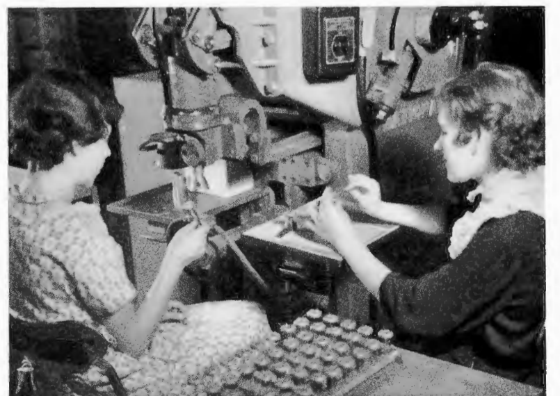
Development of power welding apparatus, controlled to split-second accuracy by thyatron control tubes, was an important factor in making possible the new improved RCA Metal Tubes which are a feature of the new 1936 RCA Victor Receivers.
