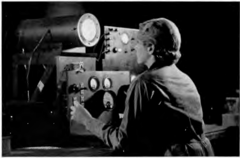
One of the reasons for the long life of RCA Victor Auto Vibrator Units is the exact adjustments made with the aid of a Cathode Ray Oscillograph. Perfect mechanical as well as electrical alignment is insured on every unit.
