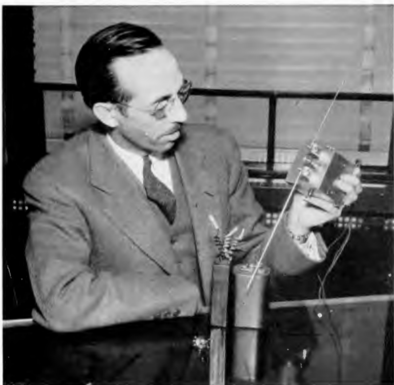
O. B. Hanson, Chief Engineer of the National Broadcasting Company, holds in his hand the world's smallest micro-wave transmitter, capable of flinging the human voice a distance of four miles. The transmitter, developed by NBC and RCA engineers, operates on wave-lengths of one meter or less, at a power of .2 watt. Also shown are the special pocket-size batteries, and the tiny "acorn tube" used in the set.
