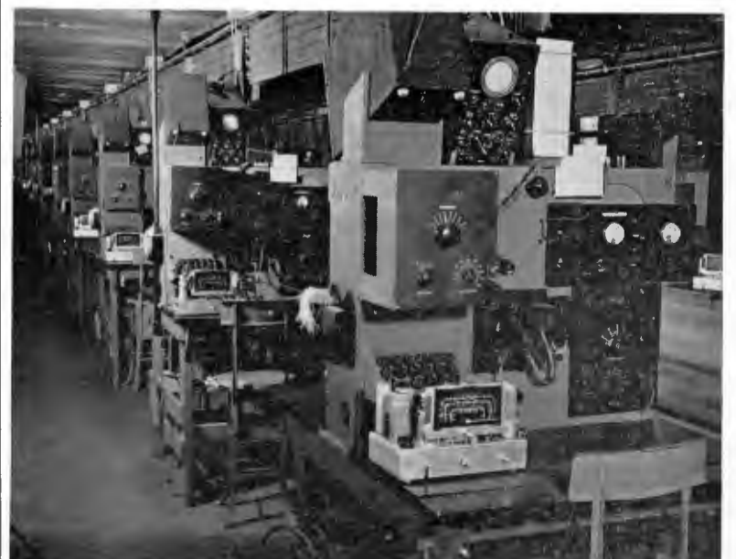
Test, test, test at every stage of manufacture is one of the reasons for the dependability of RCA Victor products. Above is shown a long line of chassis test benches in the RCA Victor plant. Note the oscillograph over each bench
