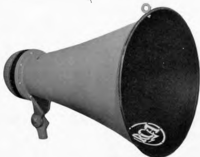
The new RCA Commercial Sound Loudspeaker MI-6260 features a permanent magnet for field excitation, thereby eliminating the extra expense of such units and their associated wiring. It has an excellent frequency response from below 140 cycles to 8000 cycles
