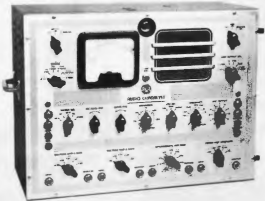
Front view of RCA's Audio Chanalyst which employs signal tracing as an efficient testing principle for diagnosing trouble in audio amplifiers, loudspeaker systems, and pick-up devices.
