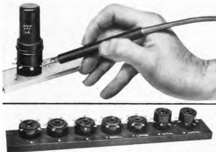
Point to point signal tracing, signal injection, and circuit checking of tubes and voltages under operating conditions is a simple matter where RCA Testpoint Adapters are used. Under working conditions, a tube in need of testing is removed from socket and inserted in a suitable adapter. The adapter with the tube is then placed back in the socket, leaving base connections easily accessible. Set of RCA Testpoint Adapters consists of seven units, one for each of the seven most common tube base types. Catalogued as MI-18760, they are available from tube and parts distributors and sell for $7.50 per set, including ready-for-use rack.
