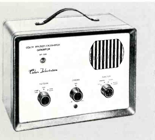
WR-64A Color-Bar/Dot/Crosshatch Generator provides 10 color bars for accurate demodulator alignment; a stable crosshatch pattern for adjusting linearity, raster size, and overscan; and a small-dot pattern for convergence adjustments.
