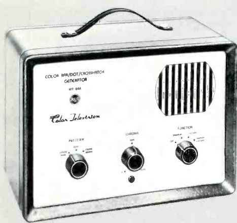
WR-64A Color-Bar/Dot/Crosshatch Generator provides 10 color bars for accurate demodulator alignment; a stable crosshatch pattern for adjusting linearity, raster size, and overscan; and a small-dot pattern for convergence adjustments.
