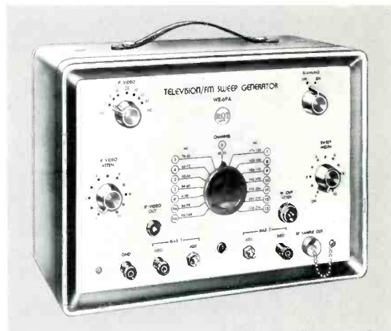
WR-69A Television/FM Sweep Generator includes pre-set switch positions for all VHF television channels and the FM broadcast band.
