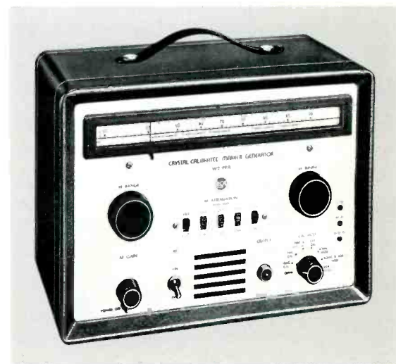
WR-99A Crystal-Calibrated Marker Generator combines the functions of the multiple-marker generator, re-broadcast transmitter, and heterodyne frequency meter, and contains facilities for checking calibration at 240 separate crystal checkpoints.
