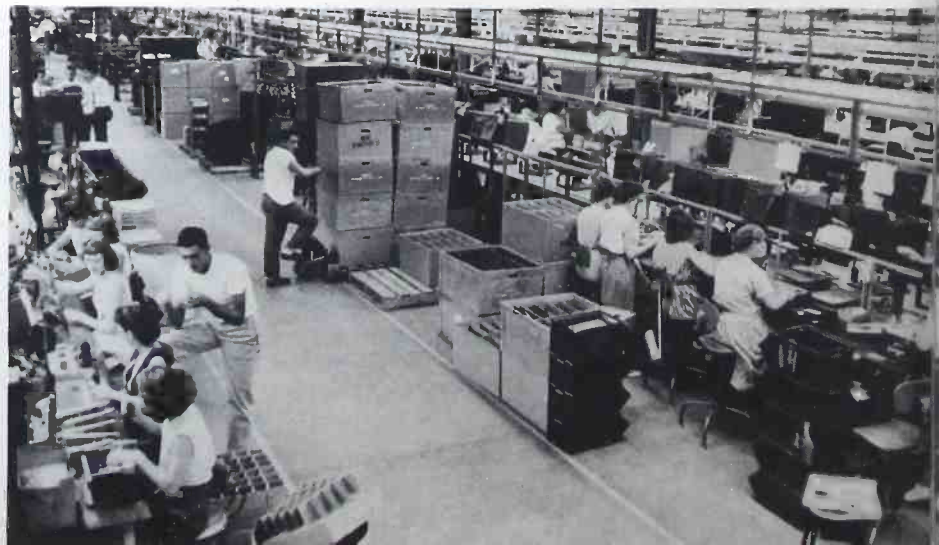
An overall view of the record-changer and amplifier assembly lines at RCA Victor's factory at Cambridge, Ohio. The plant, world's largest producer of packaged hi-fi instruments, has fifteen assembly lines capable of turning out 6,000 sets in an eight-hour shift.
