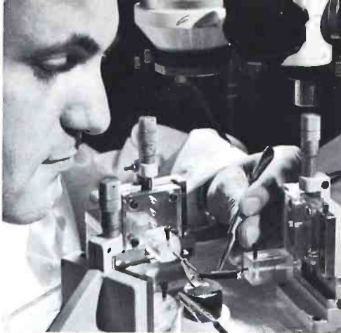
Fig. 4—An electrical probe is positioned over a silicon wafer containing 2,200 insulated-gate field-effect MOS (metal-oxide semiconductor) transistors. RCA Laboratories research produced this device which combines properties of a conventional transistor and an electron tube. It has promise for future micro-electronic circuitry.
