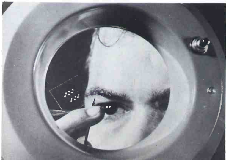
Fig. 7—RCA Laboratories research produced the first practical amplifying device to be made entirely by evaporation techniques—the TFT (thin-film transistor), shown above in a test unit. The tiny device can be made so small that over 20,000 could fit in a square inch of surface. The process promises breakthroughs in the mass production of ultraminature transistor circuits.
