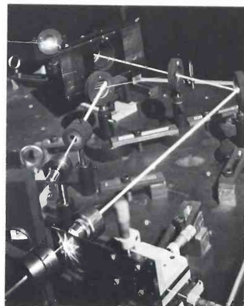
Research and development programs in laser technology and holography led to many new concepts and products. The photo shows one method used for constructing a hologram. An argon laser beam (top, left) enters an optical obstacle path where it is split into two beams by a half-silvered mirror and sent along separate paths to become the object and reference beams required to produce a hologram. The beam on the left is the object beam and can be seen to diverge into a cone just before it strikes the object (a transparency) to be holographed,
