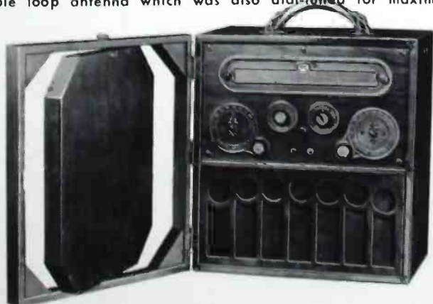
The "Radiola 26", an early superheterodyne portable receiver. The lid contained a rotatable loop antenna which was also dial-tuned for maximum sensitivity.
