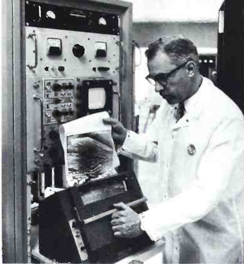
Weather pictures from the RCA APT camera system on the Nimbus II satellite are automatically transmitted to small ground stations where they are reproduced on a facsimile machine as shown. Storage of the weather picture on the APT camera vidicon tube permits transmission to simple ground stations located in any area of the world. The APT system is one of two advanced RCA television systems aboard the experimental Nimbus II satellite.
