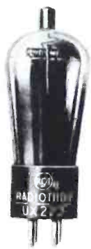
UX-222 Sharp-Cutoff Tetrode—1927
