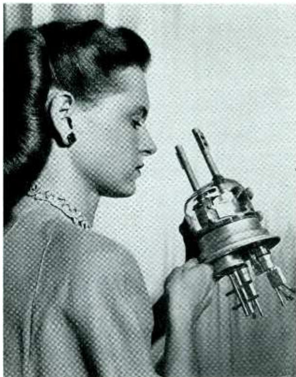
Five-kilowatt power tube developed by RCA for transmission of both television sight and sound.
