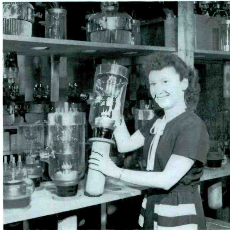
This stock of spare tubes insures continuous operation of RCA's 52 powerful overseas transmitters at Rocky Point, New York.
