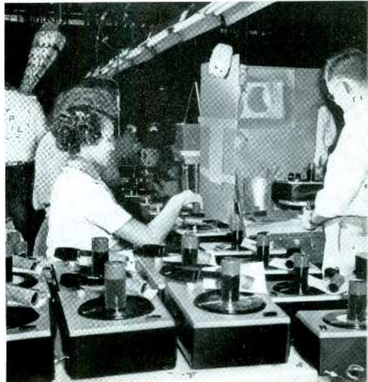
Automatic 45-rpm phonograph attachments pass final tests at the Indianapolis plant of RCA Victor.
