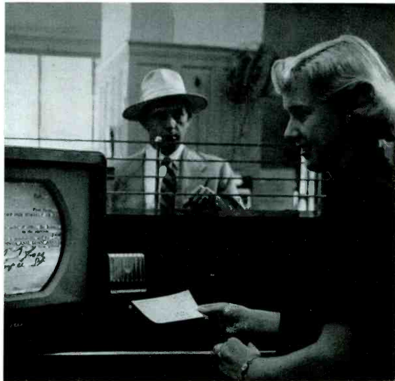
Bank employee uses RCA's Industrial TV system to compare signatures on checks, other documents.
