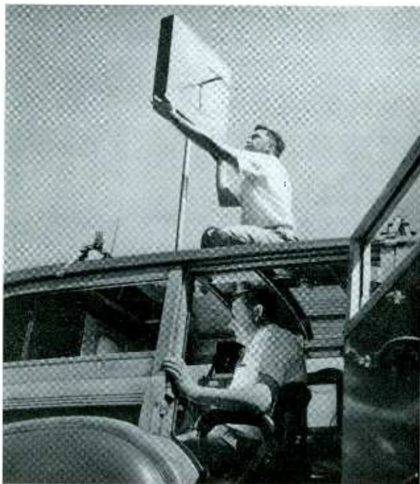
Antenna on roof of station wagon is used to make field tests of the RCA-NBC experimental UHF television station near Bridgeport, Conn.
