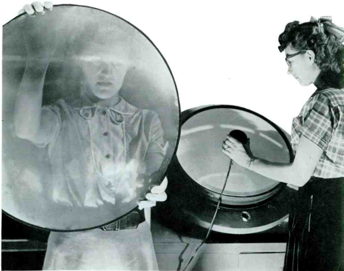
RCA's round metal color TV picture tube and aperture mask undergoing inspection at the RCA Tube Division plant in Lancaster, Pa.
