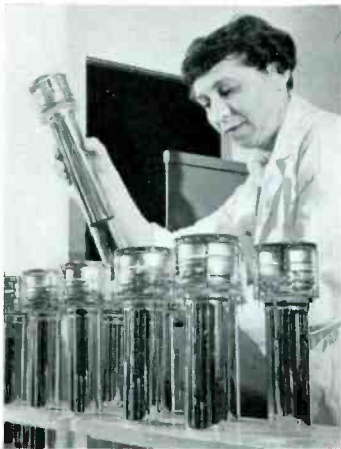
One of the intermediate inspection steps in the manufacture of RCA Image Orthicon camera tubes at the Lancaster plant.
