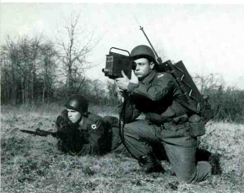
In the field, RCA-built portable television unit enables soldier-scouts to send battle picture to the command post.
