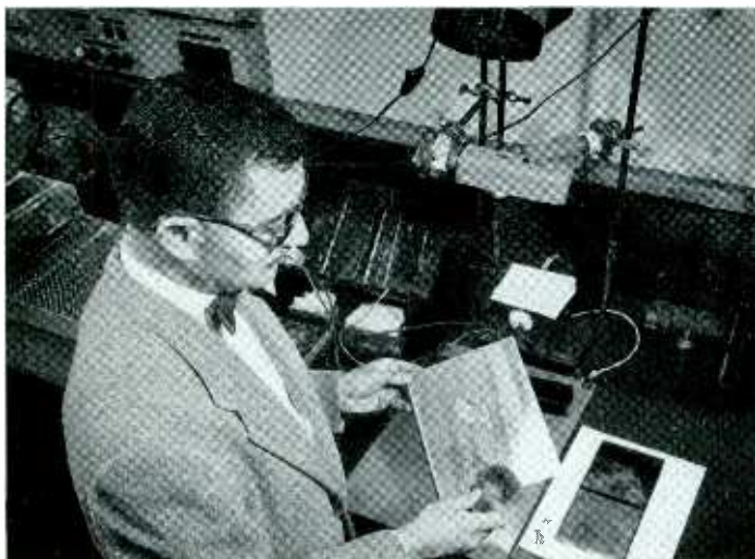
RCA "Electrofax" is a high-speed process of electronic printing on any solid surface. One use is in production of printing plates as shown above.
