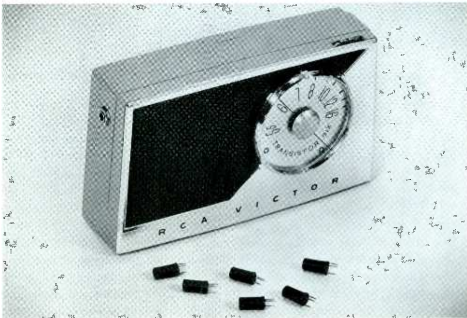
Tiny transistors (foreground) are being used in a host of new electronic devices including RCA Victor's latest pocket-size radio.
