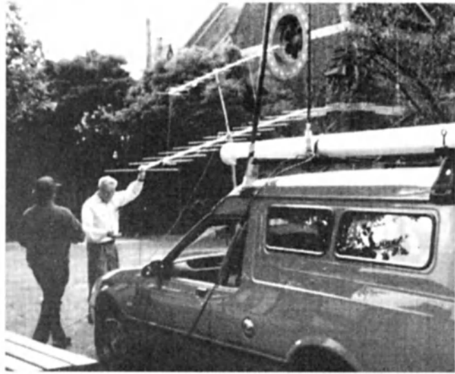
Mal (SWL) and Ken VK3CEA adjusting the antennas during a satellite pass. In the foreground is Tony VK3CAT's 'CatMobile' movable antenna support. The thick pole above the left door is an 8-metre telescopic squid pole used to support the HF wire antenna.
