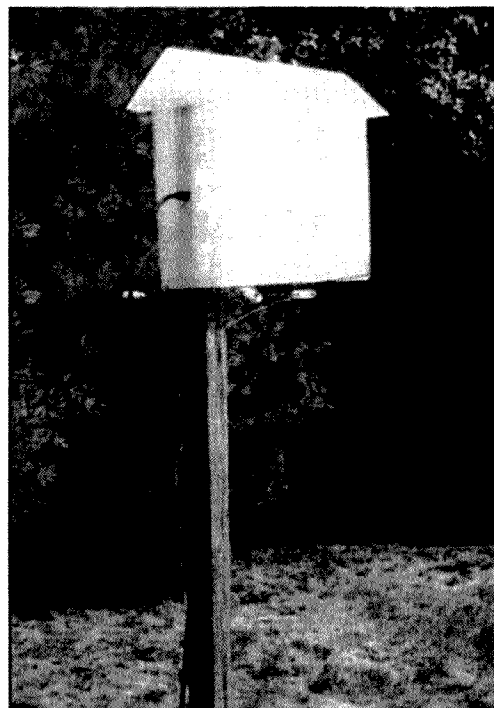
Figure 3 – The tuner assembly, enclosed in its weatherproof 'birdhouse'. The assembly is supported on wooden 4 x 4 post, which also supports the elevated radials.
