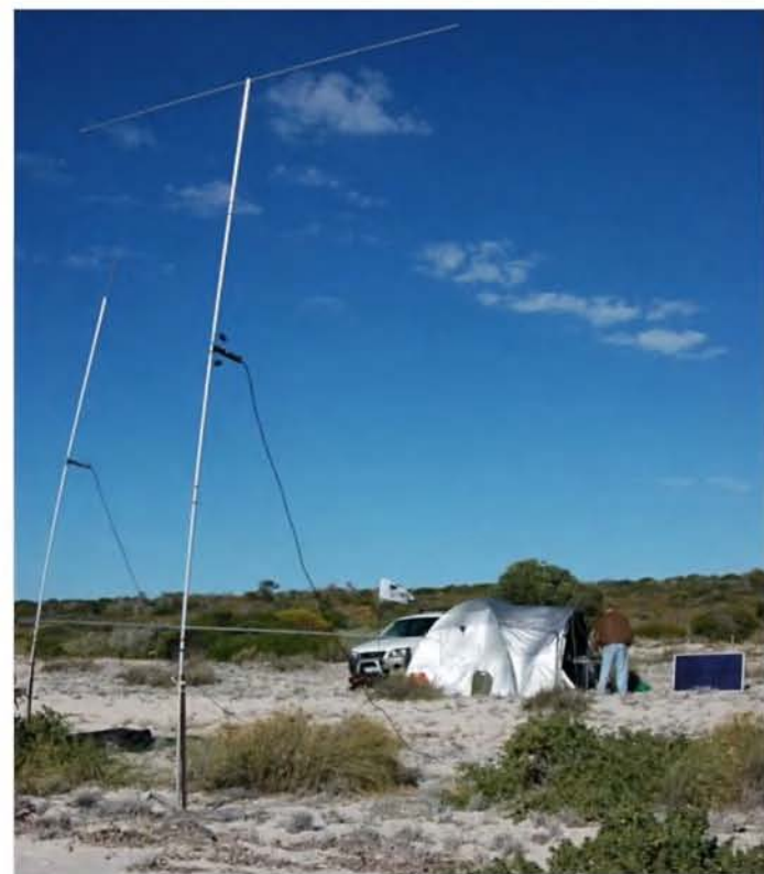
Photo 2 - The low band operating tent with the Force 12 Sigma XK40 antennas in the foreground. One is set for 20 m and the other for 40 m to allow quick change over.
