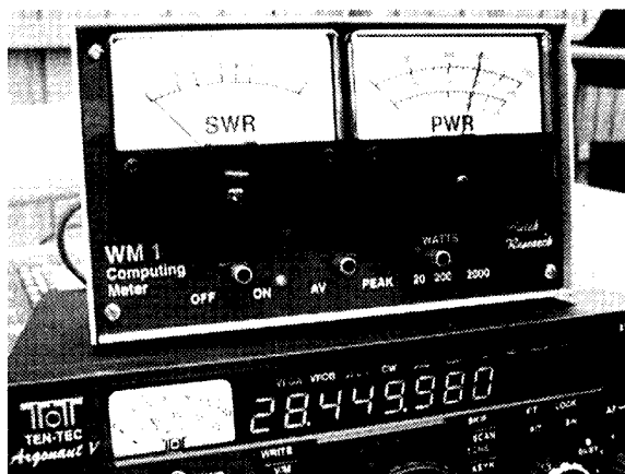
A WM1 connected to a Ten-Tec Argonaut with the power adjusted to 10 watts
