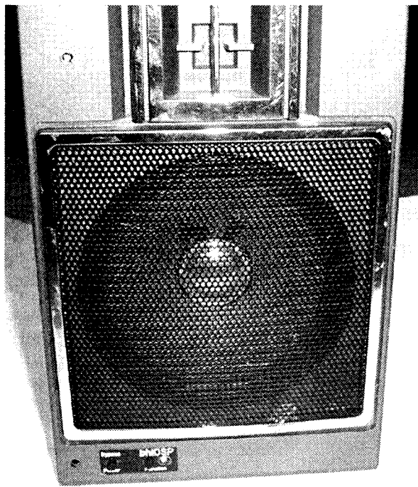
Photo 3 - Front view of the discarded Sony speaker housing showing, at the lower left corner, the two button control keyboard and tri-colour LED of the NEDSP1062 KBD. At the upper left is a 4 mm hole with the sounder behind.
