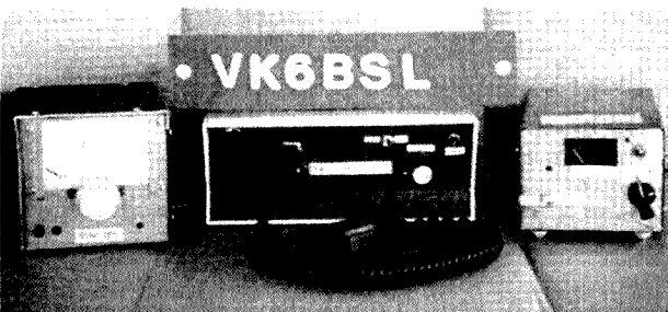
Photo 1 - From left to right, the VFO, the DSB transceiver, and the linear and SWR metering.
