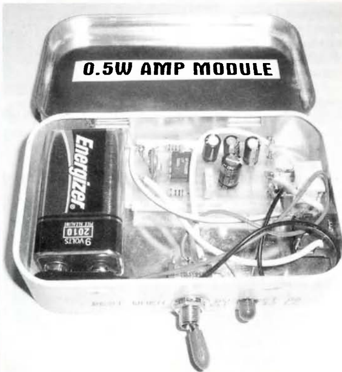
Photo 4. The 0.5 W amplifier mounted in an Altoids tin.
