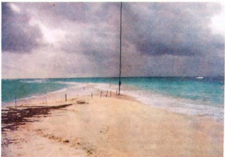
Photo 2: The 20 metre fibreglass pole supported the 160/80 m antenna. No problem with a ground plane here!
