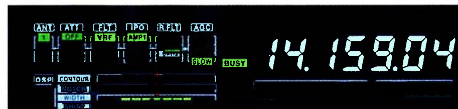
Photo 2 - The main receiver part of the bright, multi-coloured main display which includes a “block diagram” of the receiver front end, showing the antenna, attenuator, pre-selector, pre-amp, roofing filter and AGC settings in use.
