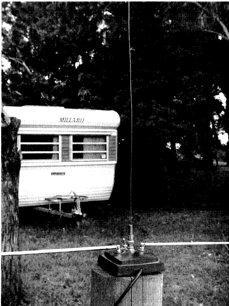
Figure 1: The set up in the field for FM or SSB use on 2 m. This antenna has been used in three states and 15 countries (as G3ZDR/p) with great results.
