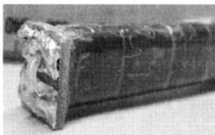
Photo 3: Formers wrapped in tape, I used clear tape just so you could see the formers, but other should work just as well. Also note I had to trim down the end pieces of PCB a bit to fit. The end shown is the end that goes to the resistors so that one centre conductor is bent over to connect to the other side and the other centre conductor is cut off flush.
