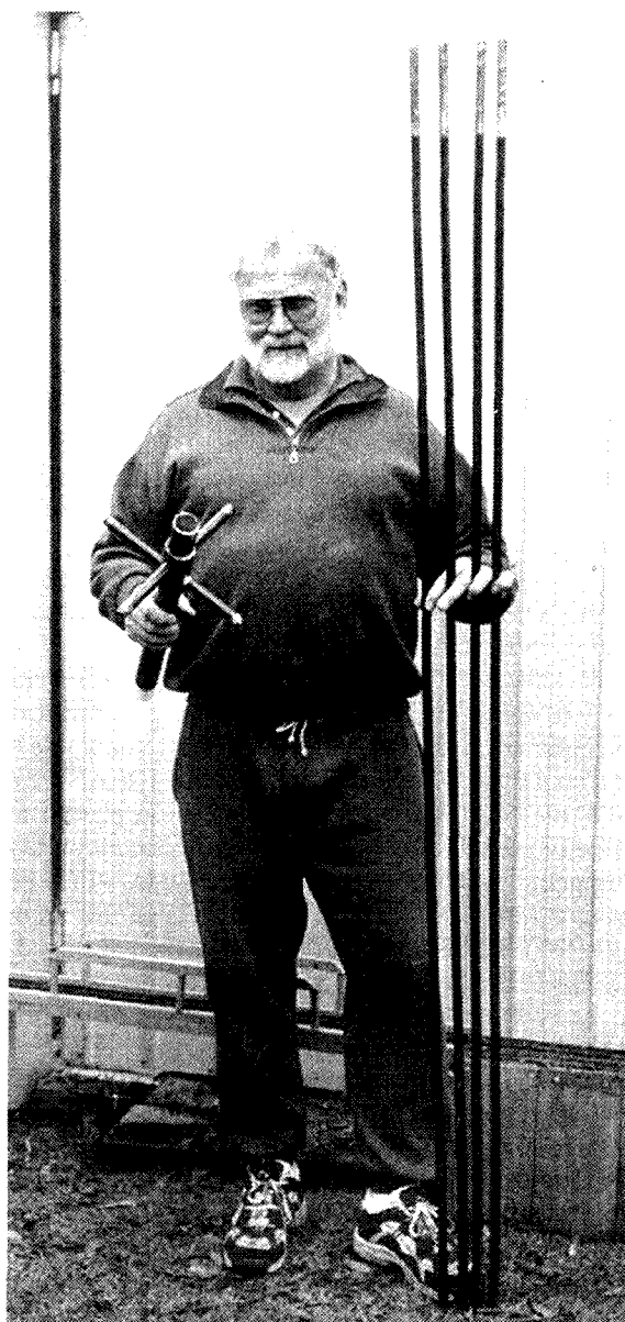
Photo 1: David VK5BUG holding the capacity top hat alloy tubes and their mounting boss.
