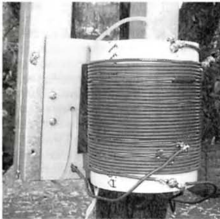
Figure 6 - Coil of 80 metre terminal unit.
