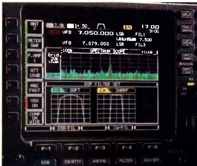
Photo 3: The large LCD screen displaying the mini spectrum scope and the filters. Note the graphical representations of the 'soft' and 'sharp' filter shapes.
