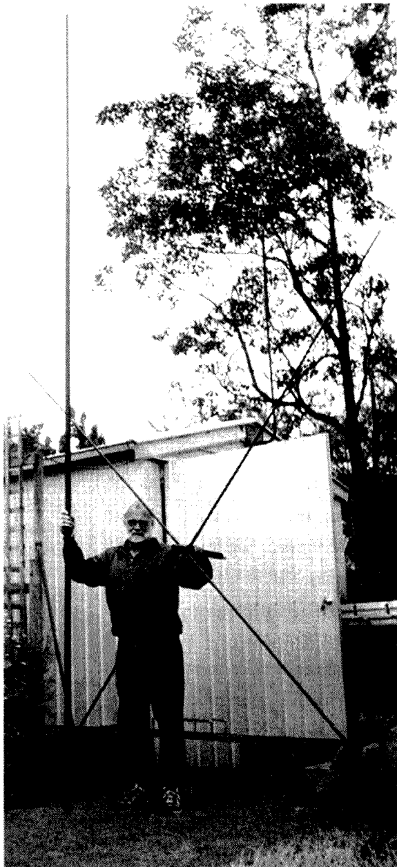
Photo 2: VK5BUG holding the top tubing section and capacity hat 'cross' for the 160/80 m "BlackBelter".
