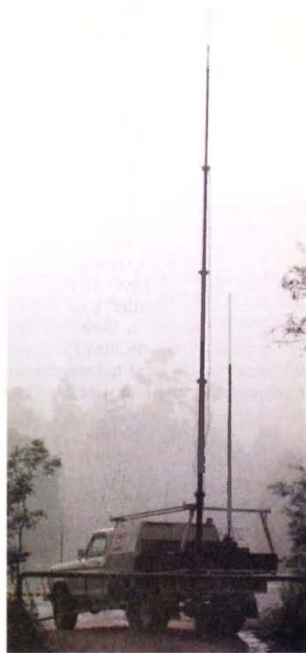
The VK7MBD truck-mounted 12 metre telescoping mast.
