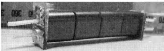
Photo 2: Partially assembled. Note outer braid of coax is taut, and holds the formers together.
