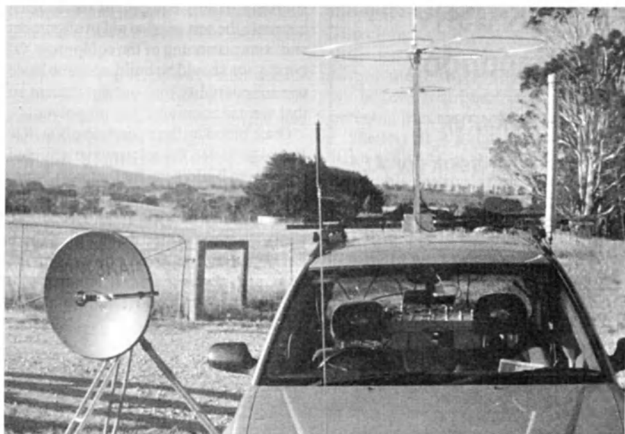
The VK3KAI station used in the 2005 Summer VHF/UHF Field Day Contest. The station antennas can clearly be seen. From L to R: Ex-PayTV dish for 10 GHz, a vertical whip for 6 m and HF liaison, a Big Wheel for 144 MHz (front), a pair of Big Wheels on 70 cm (behind, with only the bottom of the pair visible) and an Alford slot antenna on 23 cm mounted in a plastic radome.
