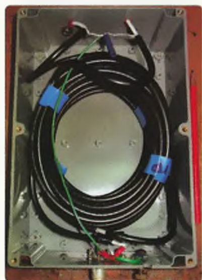
Figure 6: The completed air cored balun. Note that the two coils of coaxial cable are coiled in opposite directions.
