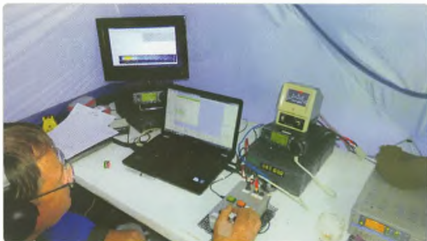
Photo 2: Jack VK3WWW operating the two metre station. To the left of the image is the setup for PSK31 including a second transceiver and monitor.
