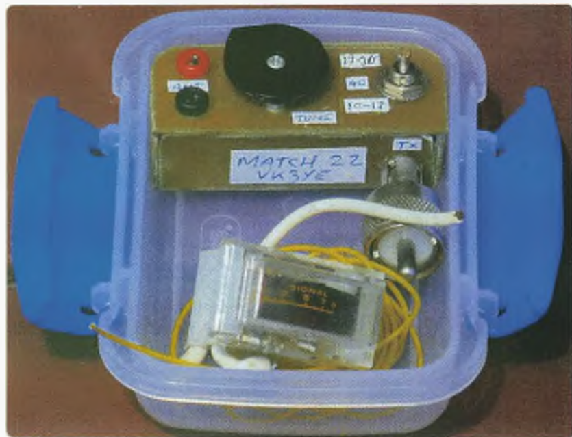
Photo 3: Light design. Where weight is critical build items on L or U shaped chassis (in this case circuit board material) and use the outer box to provide protection and hold accessories.
