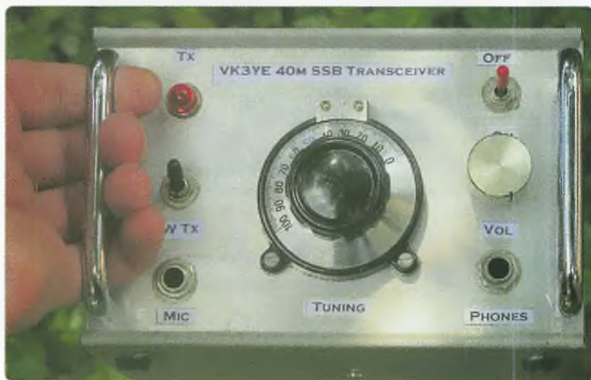
Photo 1: A tuning dial occupies pride of place while handles provide protection when packed.
