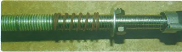
Photo 8: The threaded rod travel limiter.
