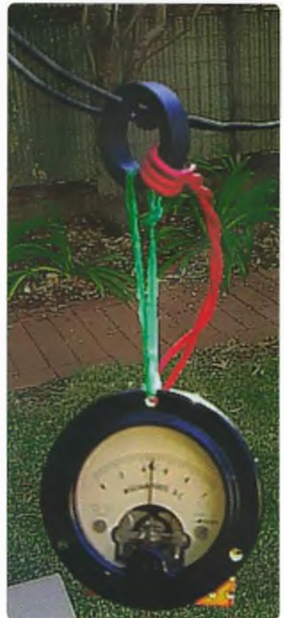
Photo 1: A toroidal current transformer coupled to a detector.
