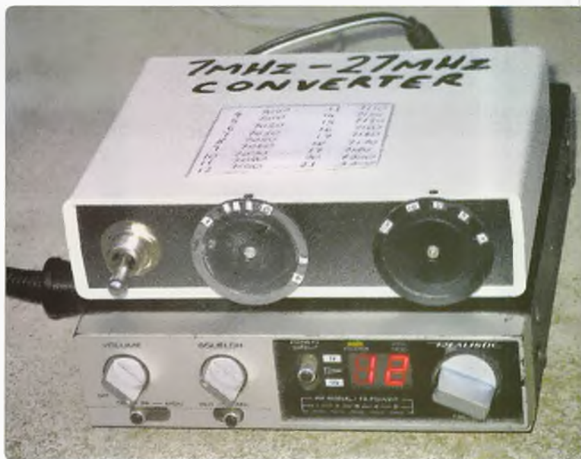
Photo 1: Converter in use with 27 MHz AM CB.
