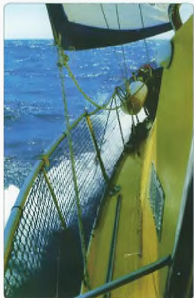
Photo 2: Showing the slightly bent rail on Colleen after the rescue package 'collided' with it.
