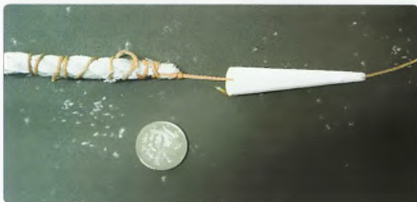
Photo 3: The homebrew nozzle and associated workings, shown referenced to a ten cent coin.
