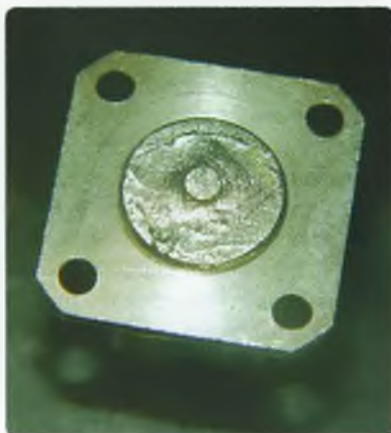
Photo 2: Shorting disc soldered onto type N male connector.
