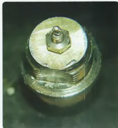
Photo 3: Shorting disc soldered onto SO239 connector.
