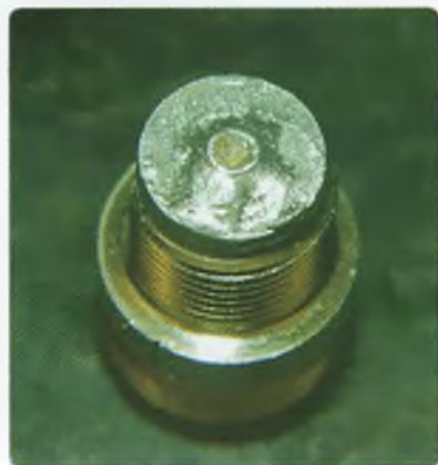
Photo 1: Shorting disc soldered onto type N female connector.
