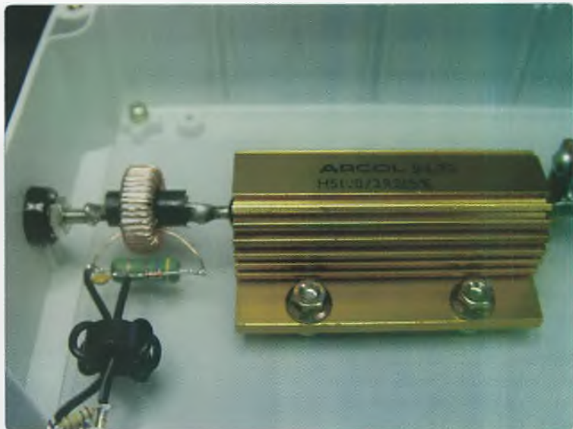
Photo 2: Load resistor plus current transformer.
