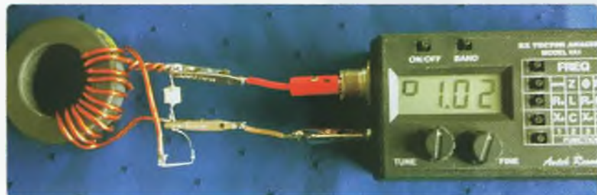
Photo 1: Shows the result obtained at 14.2 MHz with a 75 Ω resistor terminating the device and a 100 pF capacitor across the input prior to final assembly.
