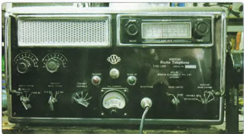
Photo 6: The Vaughan/Weston LM6 AM transceiver.
