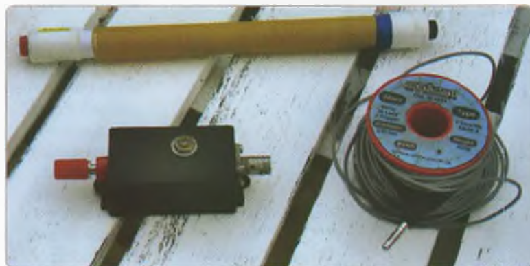
Photo 2: Triband loaded end-fed antenna.
