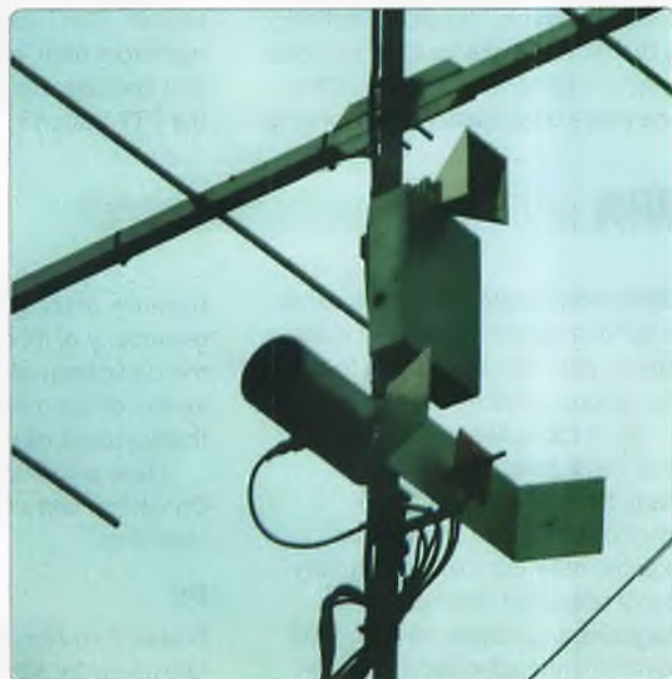
Photo 1: 10 GHz transverter (box with horn antenna) mounted 'remotely' on pole.
