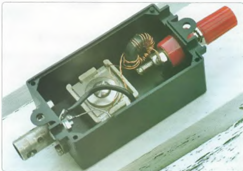
Photo 1: Inside the transformer unit.
