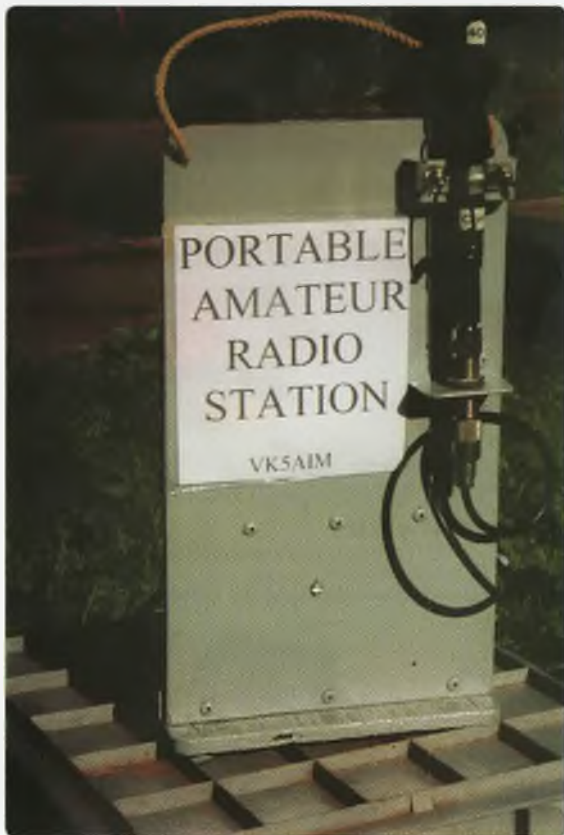
Photo 3: The back of the IC-703 portable setup, with the bracket and antenna mount. The label/notice is for visitors!
