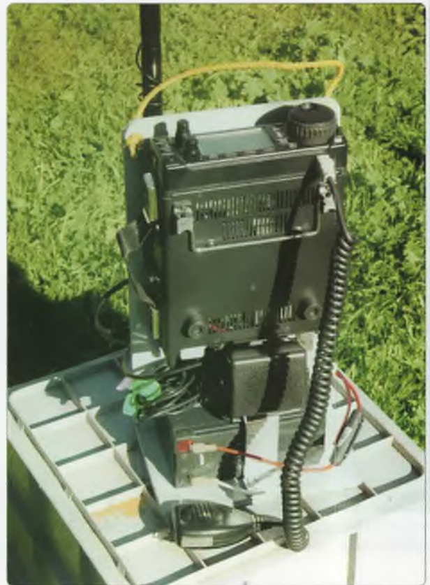
Photo 4: The complete IC-703 portable setup, complete with carry handle.
