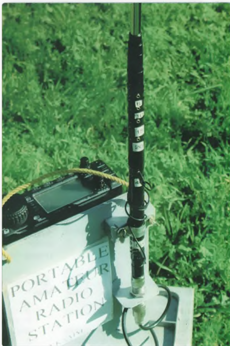
Photo 1: The multiband whip antenna and the band changing wander lead with tapping points.
