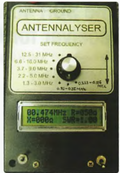
Photo 4: Additional switch positions on the front panel.
