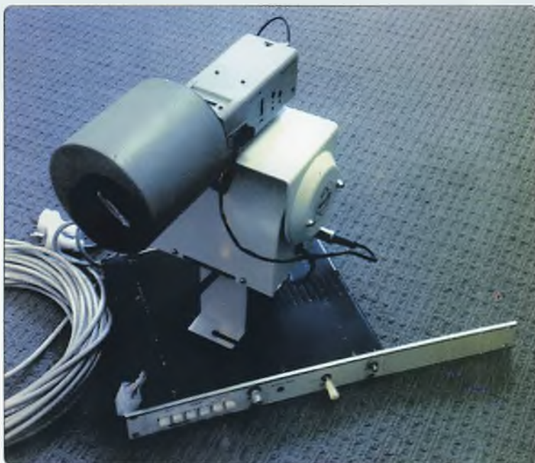
Photo 3: A remotely controlled hi-resolution DATV studio camera. Photo courtesy of Justin VK7TW.
