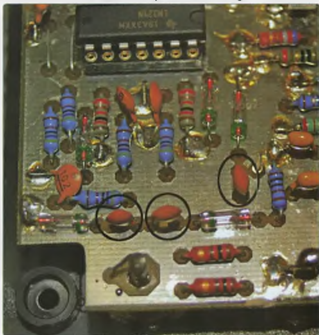
Photo 2: The three ceramic capacitors to change.
