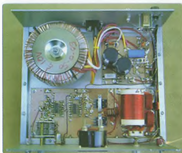
Photo 2: Internal view showing suggested 'Paddyboard' construction.
