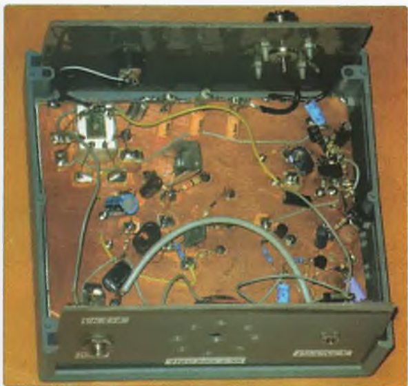
Photo 1: The top view of the Knabless Wonder's circuit board.
