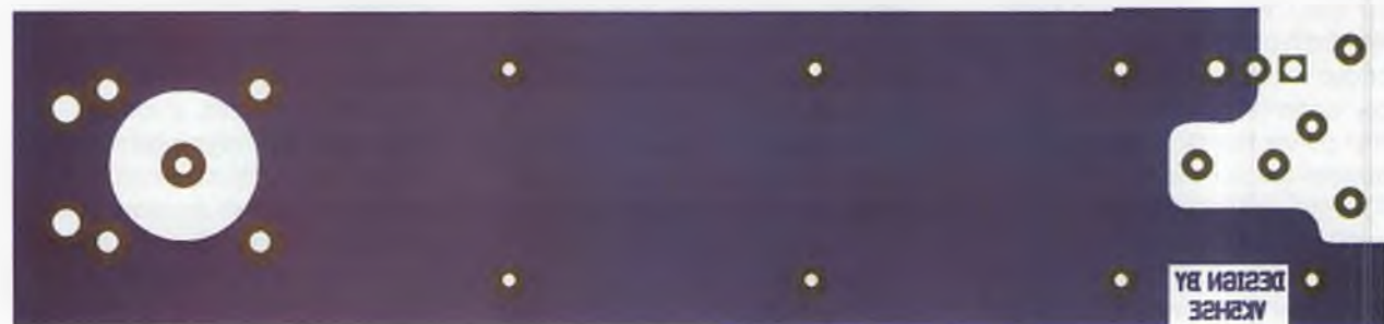
Figure 4: The dummy load bottom layer.
