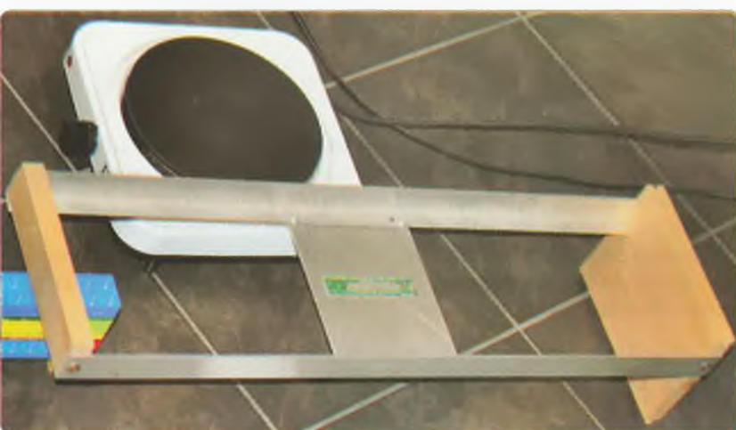
Photo 1: The lift-off jig.
