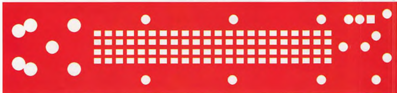
Figure 2: The dummy load solder mask.
