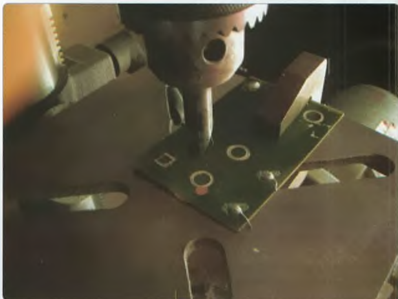
Photo 2: The test run went well, but remember that the job must be well clamped and appropriate safety equipment used.
