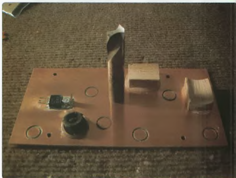
Photo 1: The solder pads have been cut – note the modified drill bit.
