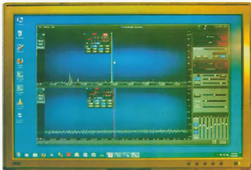
Photo2: The Flex-6500 set up for simultaneous monitoring of 20 and six metres.
