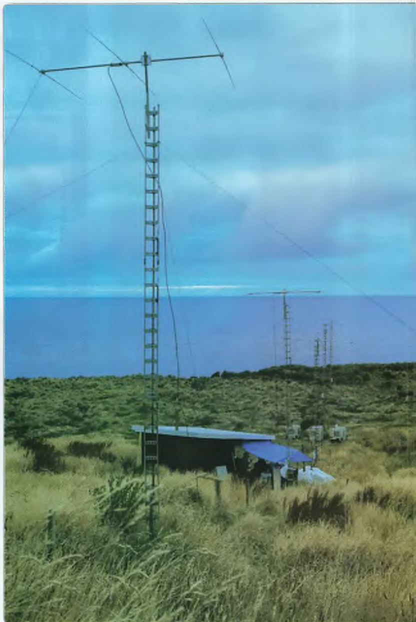
Photo 4: Second operating site with Yagis and towers. Photo courtesy of Nadir EY8MM.
