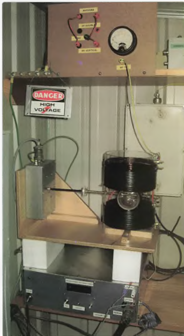
Figure 12: The completed unit with variometer inside the garden shed. The Liquid Crystal Display on the control unit shows measured antenna characteristics and tuning details. Note the common mode inductor in the CAT-5 network cable which helps reduce interference. The High Voltage sign isn't just for show; there is about 1500 V of RF potential at the top connector of the variometer when the transmitter is operating.
