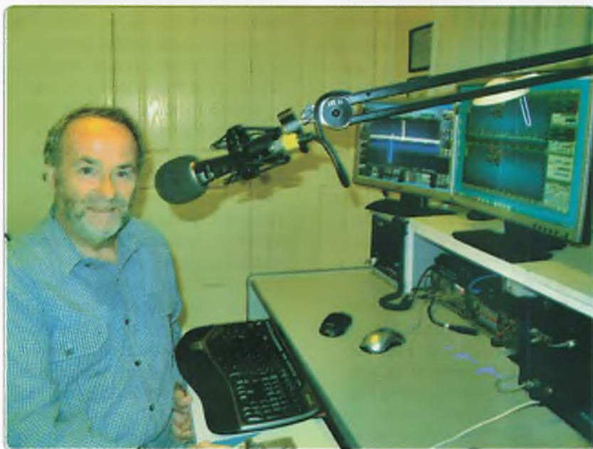
Photo 5: The author's Flex station – the Flex-5000 on the left and the Flex-6500 on the right.
